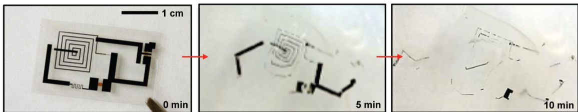
Figure 14: Images showing the time sequence of dissolution the water soluble electronics in DI water
