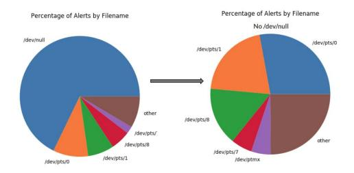
Further inspection revealed that /dev/null was causing a majority of the false positives. Because /dev/null is essentially the garbage can of the OS, we felt comfortable whitelisting it. We did so and reran the program. This drastically reduced the number of alerts generated.
