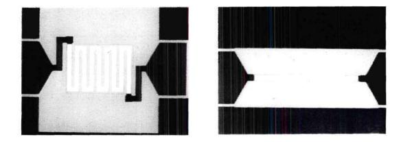
Figure 6.6 Serpentine and linear resistor designs for the single-sided resistors. To evaluate the design limits, length, width, and number of squares were varied.
