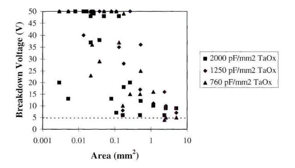
Figure 6.22 Breakdown voltage verses area for different thicknesses of  $Ta_2O_5$  after top passivation. Values at 50 volts did not break down.
