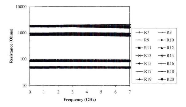
Figure 6.8 Linear resistors on flex.
