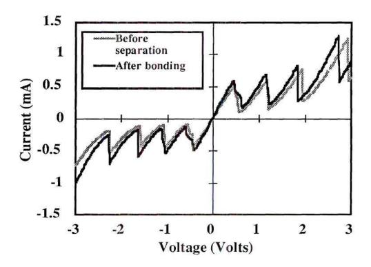
Figure 3.5 Four vertically stacked 16  $\mu m^2$  RTDs before and after substrate removal and bonding.
