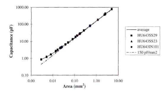
Figure 6.24 Capacitance verses area for 2kA DLC on flex at 10kHz for parallel plate capacitor design. Dashed (150pF/mm<sup>2</sup>) and dotted (200pF/mm<sup>2</sup>) lines give the theoretical values of capacitance for the stated capacitance per unit area (CPUA).
