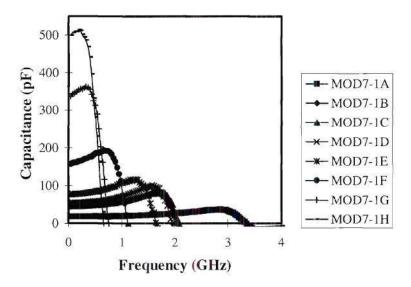
Figure 6.28 One port measurements showing resonant frequency for 1000A Ta $_2O_5$  parallel plate capacitors. See Table 6.6 for areas.
