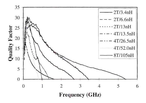
Figure 6.14 Quality Factor, Q, of thin film inductors on flex with far-field (over 90 mils away) ground plane.
