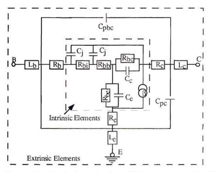
Figure 8.3 Equivalent circuit of HBT when normally biased.<sup>4</sup>
