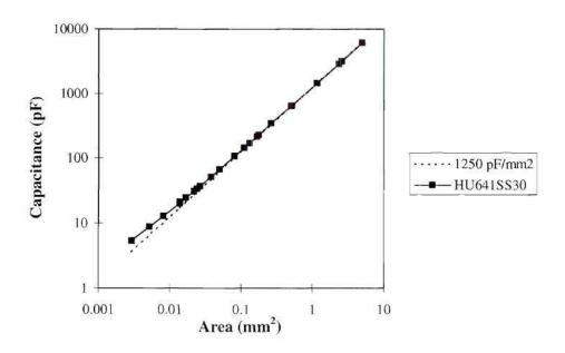
Figure 6.26 Capacitance verses Area for 1.5kA Ta<sub>2</sub>O<sub>5</sub> on Flex at 10kHz for parallel plate capacitor design. Dotted (1250 pF/mm<sup>2</sup>) line gives the theoretical values of capacitance for the stated capacitance per unit area (CPUA).
