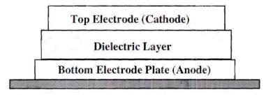
Figure 6.3 Cathode and anode definitions of the thin film capacitor.
