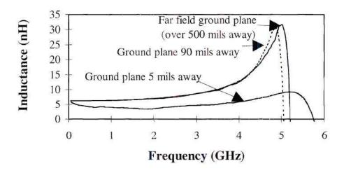
Figure 6.15 Measured inductance vs. frequency for the 3.4 nH inductor design with the ground plane distance varied. Measured inductance value was 6.3 nH.
