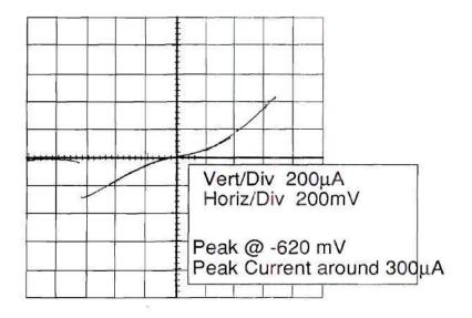
Figure 3.18 Negative region current-voltage characteristics of RTD after integration with comparator circuit.
