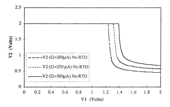
Figure 3.23 Measured current-voltage characteristics of comparator circuit without RTD.
