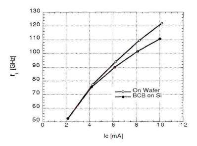
Figure 5.8 Comparison of HBT cutoff frequency verses  $I_c$  before and after integration to Si.
