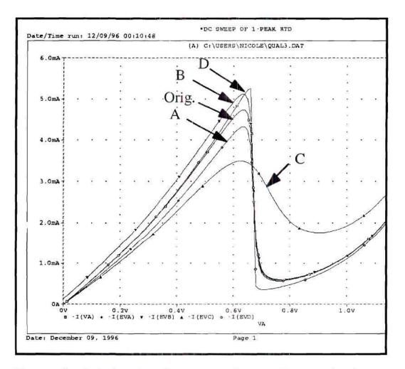
Figure 3.7 Variations in DC response of the RTDs resulting from changes in the parameters in the resonant tunneling current equation.
