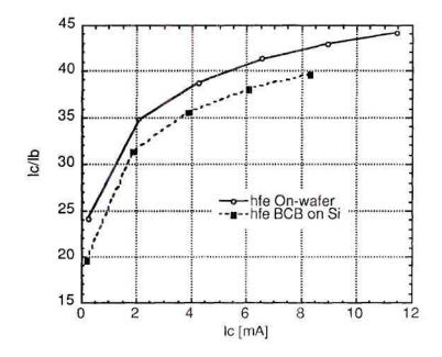
Figure 5.7 DC  $\beta$  vs. collector current plot of HBT before and after bonding to BCB on Si.
