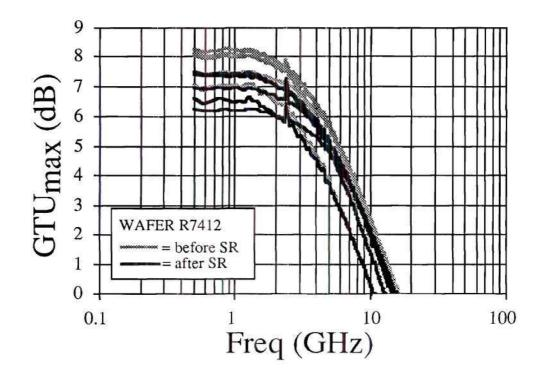
Figure 4.6  $GTU_{max}$  of a THETA for  $V_{ce}$ =1.5V,  $I_b$  from 0.5 to 2.5 mA (0.5 mA steps), and  $I_e$  from 2.8 to 11.5 mA before and after substrate removal and bonding to sapphire.  $F_{max}$  was around 17 GHz for  $I_e$ =11.5 mA. Similar characteristics were observed for alumina and quartz host substrates.
