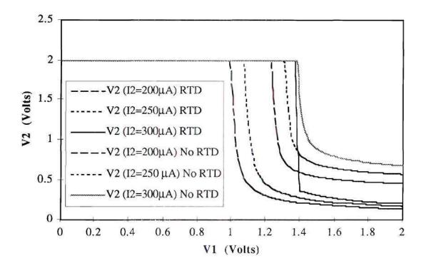
Figure 3.24 Measured current-voltage characteristics of comparator circuit with and without RTD. When the current reached 300  $\mu$ A, the RTD switched.
