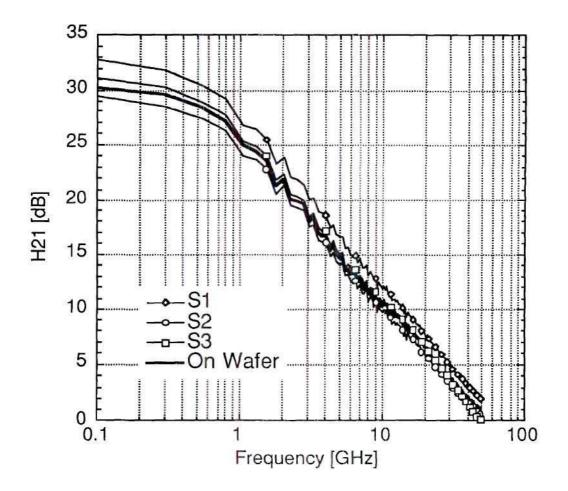
Figure 5.5 H<sub>21</sub>of HBT at Vce=1.5V Ic=2mA on various substrates.
