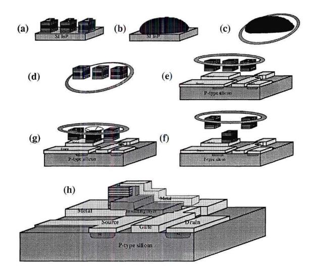
Figure. 2.3 Substrate removal and bonding using a transfer diaphragm. The transfer diaphragm enables the alignment and bonding of the thin film devices to the host substrate as well as the ability to process both top and bottom of the device. Post-processing of top contact pads is done after device has been contact bonded to the host substrate.
