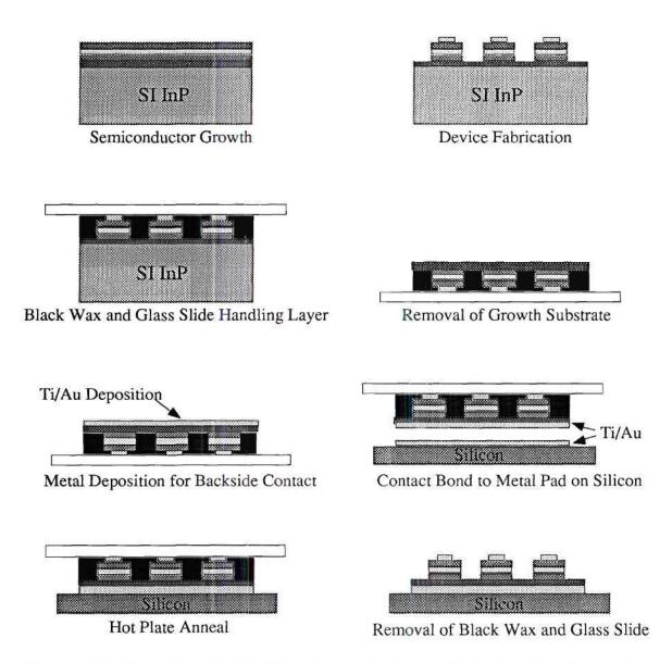
Figure. 2.2 Transfer of thin film devices to host substrate without use of transfer diaphragm. Contacts are made on both sides of the device.
