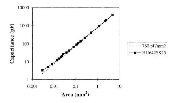
Figure 6.27 Capacitance verses Area for 2.3kA  $Ta_2O_5$  on Flex at 10kHz for parallel plate capacitor design. Dotted (760 pF/mm<sup>2</sup>) line gives the theoretical values of capacitance for the stated capacitance per unit area (CPUA).
