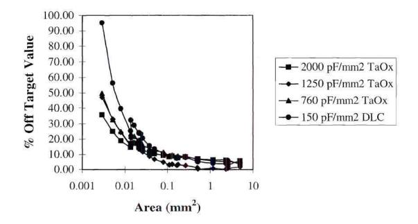
Figure 6.23 Percentage off target verses capacitance.
