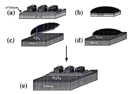
Figure. 2.1 Substrate removal and bonding of RTDs onto silicon host substrates.
