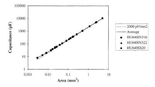
Figure 6.25 Capacitance verses Area for 1kA  $Ta_2O_5$  on Flex at 10kHz for parallel plate capacitor design. Dotted (2000 pF/mm2) line gives the theoretical values of capacitance for the stated capacitance per unit area (CPUA).
