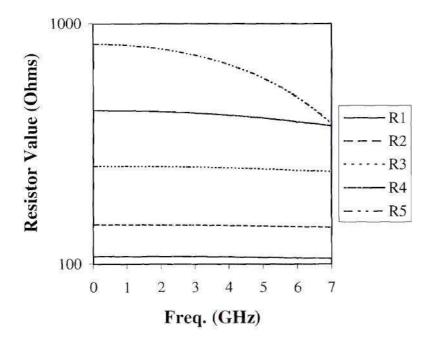
Figure 6.7 Two-sided resistor design results. Ground plane is on the back of the 1 mil flex.
