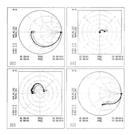
Figure 5.4 Comparison of S-parameters of HBT on-wafer (dark line) and HBT on BCB insulated Si substrate (gray line).
