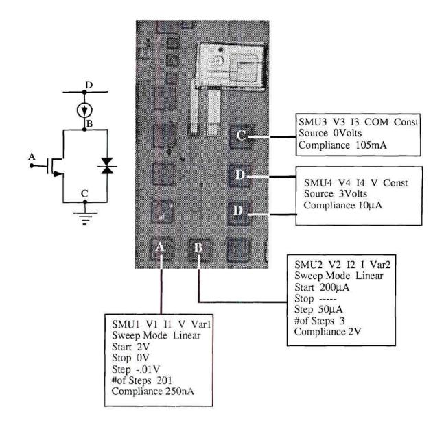
Figure 3.22 Bias conditions for testing of comparator circuit with InP-RTD.
