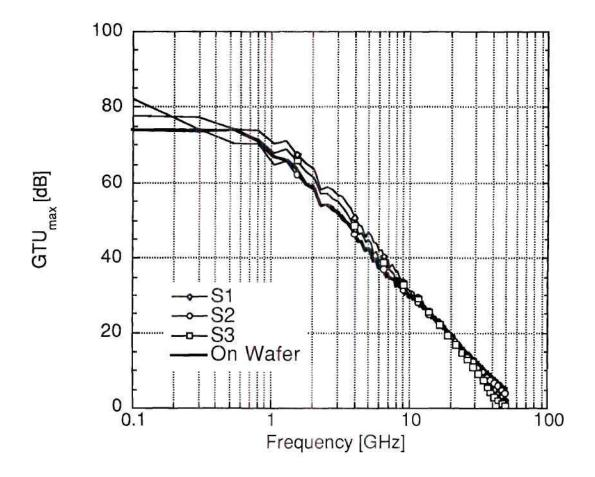
Figure 5.6  $GTU_{max}$  of HBT at  $V_{ce}$ =1.5V and  $I_c$ =2mA on various substrates.
