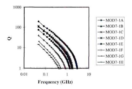
Figure 6.29 Quality factor vs. frequency for 1000A Ta  $_2O_5$  parallel plate capacitors with different areas. See Table 6.6 for area for particular capacitor.
