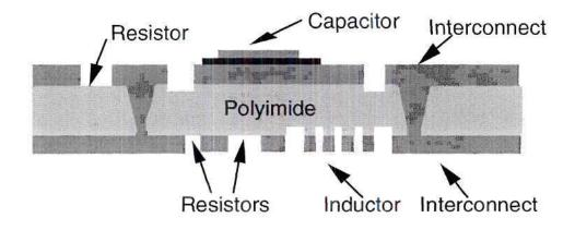
Figure 6.1 Cross-section of two-sided integrated passives on flex.
