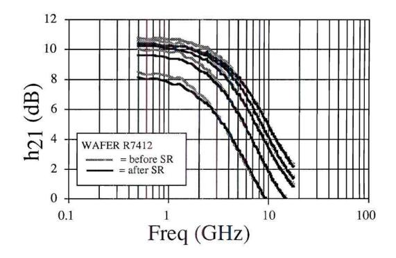
Figure 4.5  $H_{21}$  of the THETA for  $V_{ce}$ =1.5V,  $I_b$  from 0.5 to 2.5 mA (0.5 mA steps), and  $I_c$  from 2.8 to 11.5 mA before and after substrate removal and bonding to sapphire.  $F_t$  exceeded 20 GHz for  $I_b$ >1.5 mA ( $I_c$ >6.8 mA). Similar characteristics were observed for the alumina and quartz host substrates.
