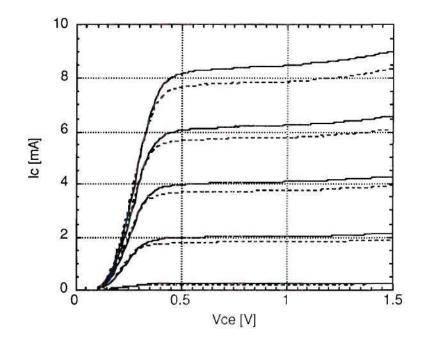
Figure 5.3 IV characteristics of HBT on-wafer (solid) and bonded to BCB on Si (dashed).
