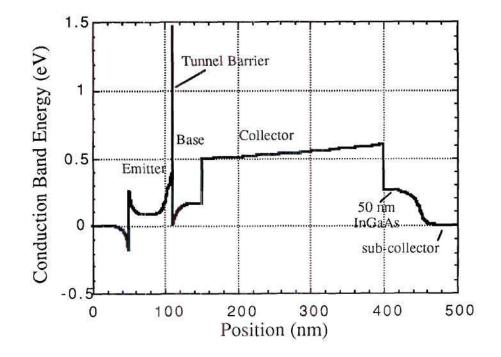
Figure 4.1 Computed conduction band profile for the Tunneling Hot Electron Transfer Amplifier. The emitter thickness has been reduced in the simulation so that the entire structure can be seen in one plot.
