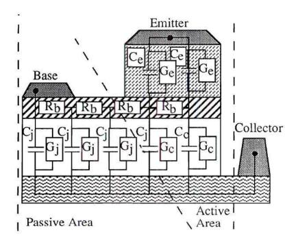
Figure 8.2 Lumped element circuit for the HBT.<sup>3</sup>
