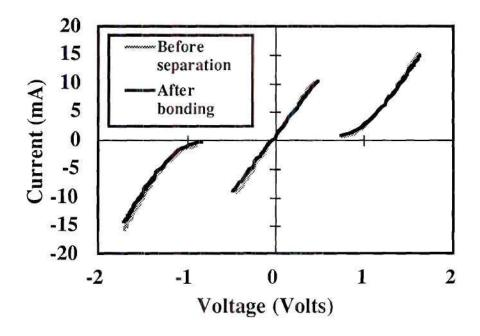
Figure 3.4 256  $\mu m^2$  high PVR RTD before and after substrate removal and bonding. The corresponding positive and negative PVRs were 13 and 21, respectively.
