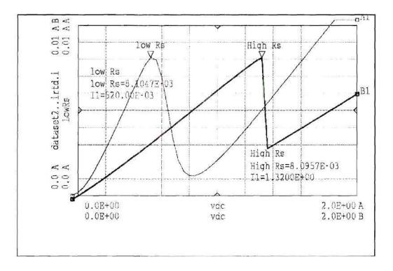
Figure 3.10 DC characteristics of low and high series resistance RTDs modeled using MDS.
