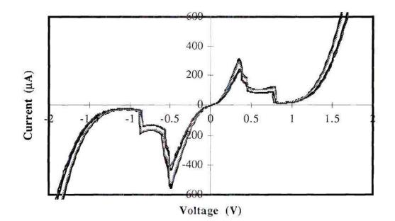
Figure 3.11 On wafer DC characteristics of low current 6  $\mu$ m RTD's with thick planarizing nitride.
