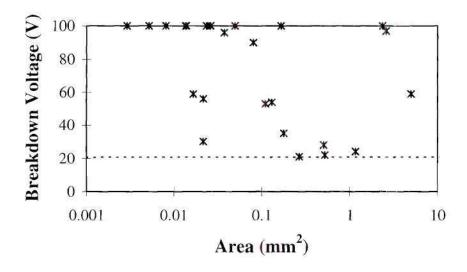
Figure 6.21 Breakdown voltage verses area for different thicknesses of DLC after top passivation. Values at 100 volts did not break down.
