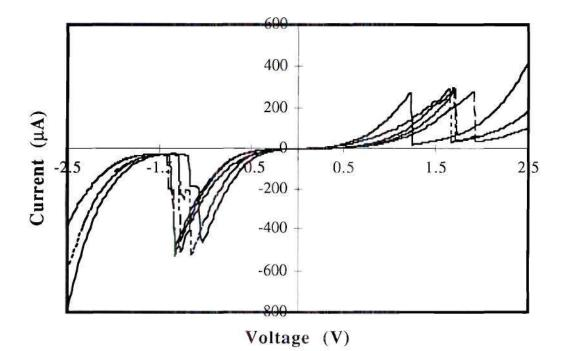
Figure 3.12 Low current 6  $\mu$ m RTD's with thick planarizing nitride after substrate removal and bonding.
