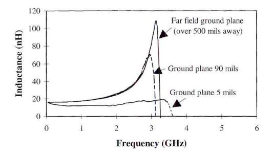
Figure 6.17 Measured inductance verses frequency for 13.5 nH inductor design with the ground plane distance varied. Measured inductance was found to be 16.6 nH with far field greater than 90 mils away.
