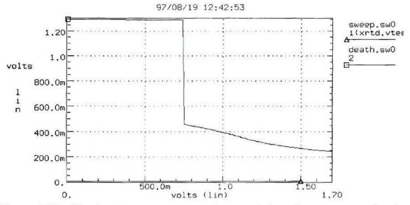
Figure 3.21 Simulated current-voltage characteristics of comparator circuit with RTD.
