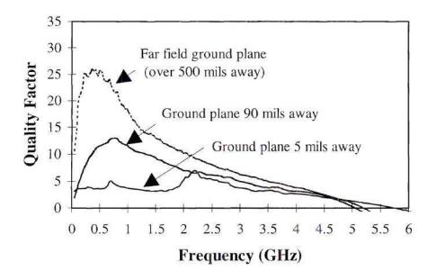
Figure 6.16 Changes in quality factor vs. frequency for the 3.4 nH inductor design as a function of distance of ground plane.
