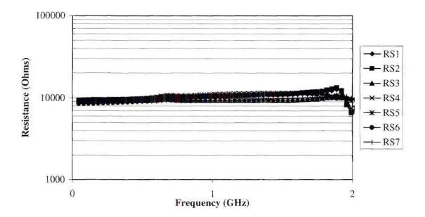
Figure 6.11 Serpentine resistors on flex. Higher parasitics than the linear resistors can be observed, partially due to capacitive coupling between lines.
