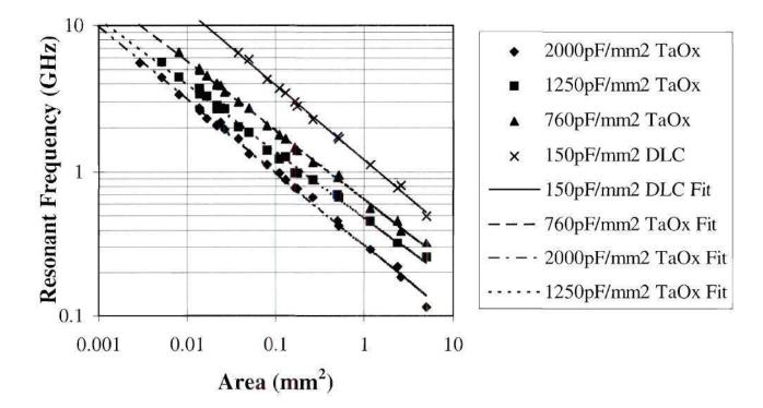
Figure 6.34 Resonant Frequency vs. Area for Different CPUA of Ta<sub>2</sub>O<sub>5</sub> and DLC.
