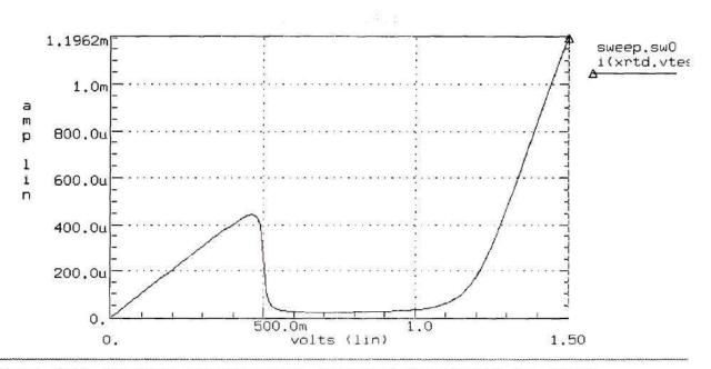
Figure 3.19 Modeled current-voltage characteristics of RTD for circuit simulations.
