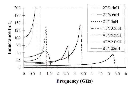
Figure 6.13 Inductance verses frequency for different inductance values and designs for ground plane over 90 mils away.
