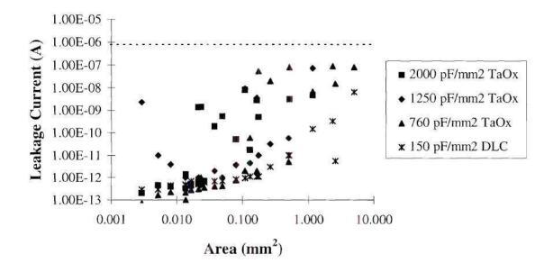
Figure 6.20 Leakage current at 5 volt bias verses area.
