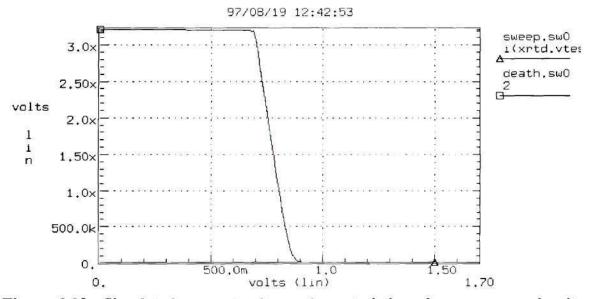
Figure 3.20 Simulated current-voltage characteristics of comparator circuit without RTD.
