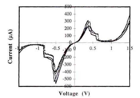
Figure 3.14 Low current 6  $\mu$ m RTD's after wet etch of nitride and substrate removal.
