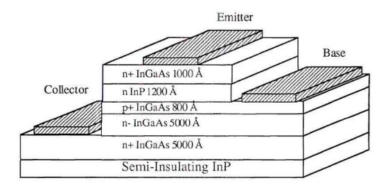
Figure 5.2 SHBT device structure used in this study.
