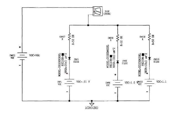
Figure 3.8 A large signal model in MDS for simulation of current-voltage characteristics of RTD.
