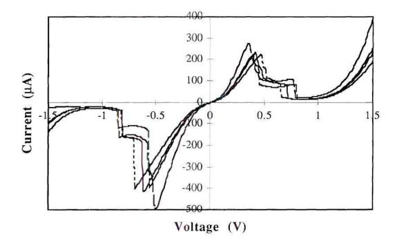
Figure 3.13 Current-voltage characteristics of on wafer low current 6  $\mu$ m RTD's after RIE nitride removal.
