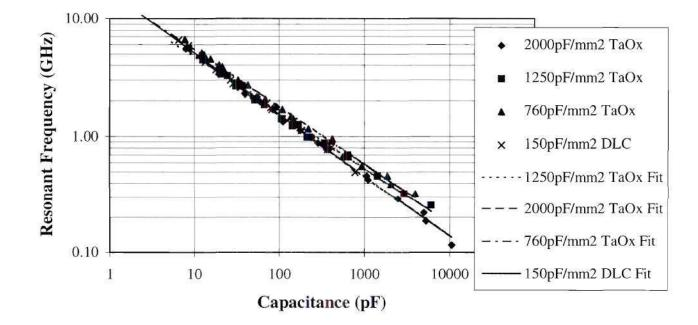
Figure 6.33 Resonant frequency verses capacitance for different CPUA  $Ta_2O_5$  and DLC.
