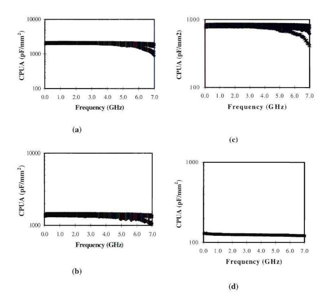
Figure 6.32 Capacitance per Unit Area (CPUA) verses frequency for the first row of the (a) 1000A  $Ta_2O_5$ , (b) 1500A  $Ta_2O_5$ , (c) 2500A  $Ta_2O_5$ , and (d) 2000A DLC parallel plate capacitors. The CPUA remains constant for the smaller footprint devices while the larger footprint devices, show a drop due to larger parasitics which were not included in the extraction.
