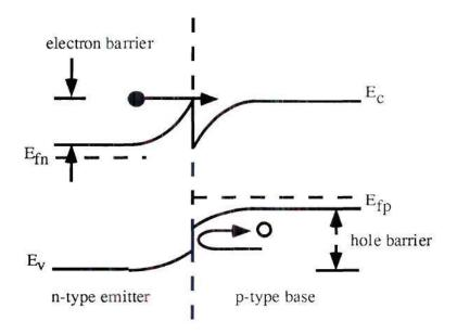
Figure 5.1 Energy band diagram of the emitter-base transition region of the HBT.<sup>2</sup>
