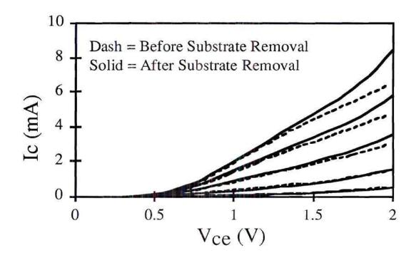
Figure 4.4 DC characteristics of a THETA before and after substrate removal and bonding to silicon coated with 0.5  $\mu$ m of silicon nitride.
