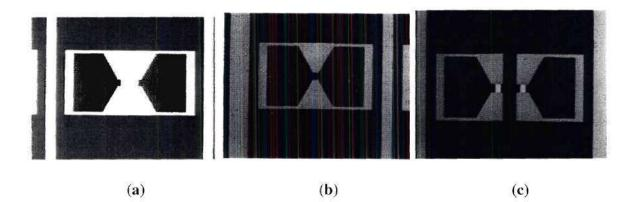
Figure 6.4 (a) Open, (b) through, and (c) matched load on-wafer LRM calibration designs for de-embedding the resistor launches and transition region from one-side TaN resistors.
