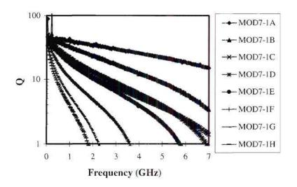
Figure 6.31 Quality factor verses frequency of some of the 150pF/mm<sup>2</sup> DLC parallel plate capacitors extracted from 1-port measurements.
