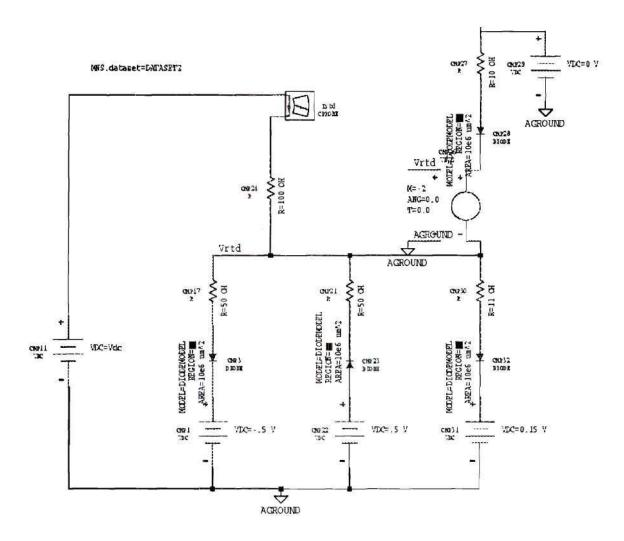
Figure 3.9 A resistor is added in series with the model for simulation of the voltage shift which occurred for the thin film RTDs.
