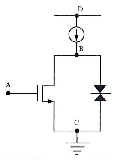
Figure 3.15 Silicon comparator circuit with integrated InP RTD.
