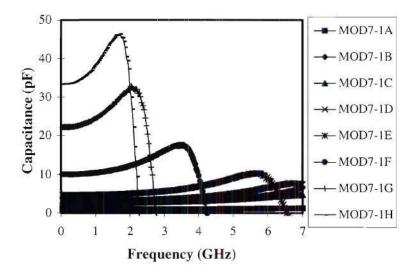
Figure 6.30 Capacitance verses frequency of some of the 150pF/mm<sup>2</sup> DLC parallel plate capacitors extracted from 1-port measurements.
