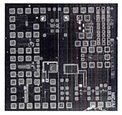
Figure 3.16 Photograph of RTD integrated with Si comparator circuit.
