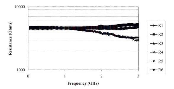
Figure 6.9 Linear long length resistors on flex. Higher parasitics are due to increased length of resistors.
