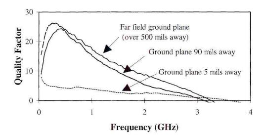
Figure 6.18 Changes in quality factor vs. frequency for a 13.5 nH inductor design as a function of distance of ground plane.
