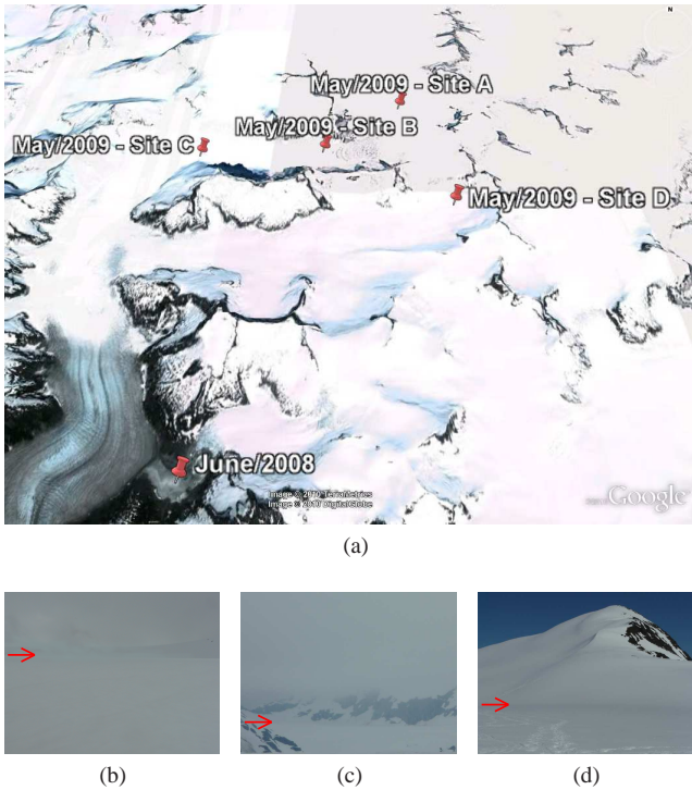
Fig. 1: (a) A map of the relative positions of the various test sites on Mendenhall Glacier during the June 2008 and May 2009 field tests. Test site on Lemon Creek Glacier is not shown. (b)-(d) Sample images from Lemon Creek Glacier and Mendenhall Glacier showing obscured horizons. For clarity, the horizon line is indicated on each sample image.
