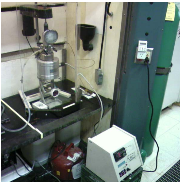
Figure 36. Parr 4560 reactor with a Parr 4842 set for hydrogenation.
