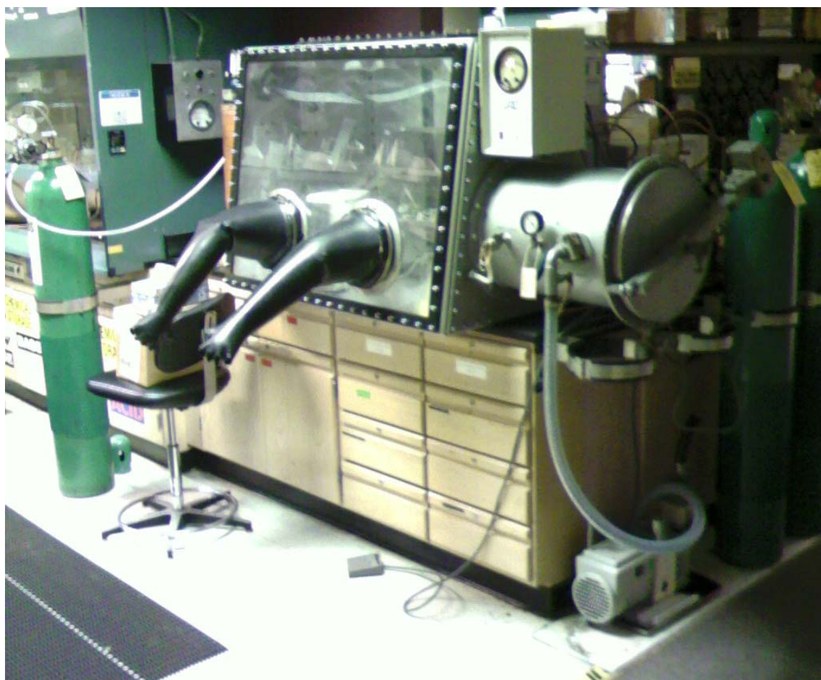
Figure 33. Glove-box set for air sensitive chemical storage.
