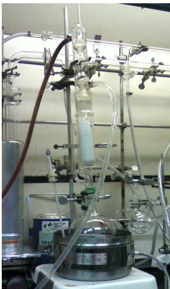
Figure 41. Soxhlet extractor used for ethanol organosolv lignin preparation.
