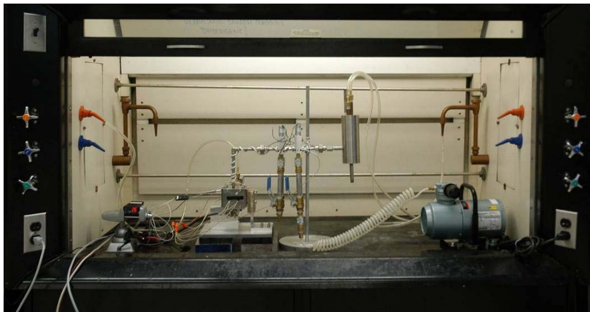
Figure 40. The experimental lignin pyrolysis setup used for bio-oil production.
