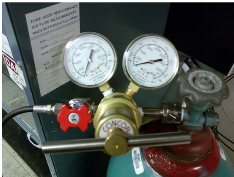
Figure 37. Safety shut-off valve connected to a hydrogen (CGA-350) regulator.
