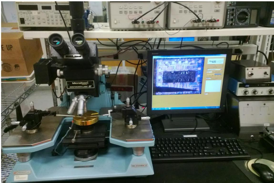
**Figure 4-9: Wentworth labs probe station. Capable of probing and taking color images using custom computer software. CREE LED source was fitted to improve image quality and to enable computer control of the light intensity.**
