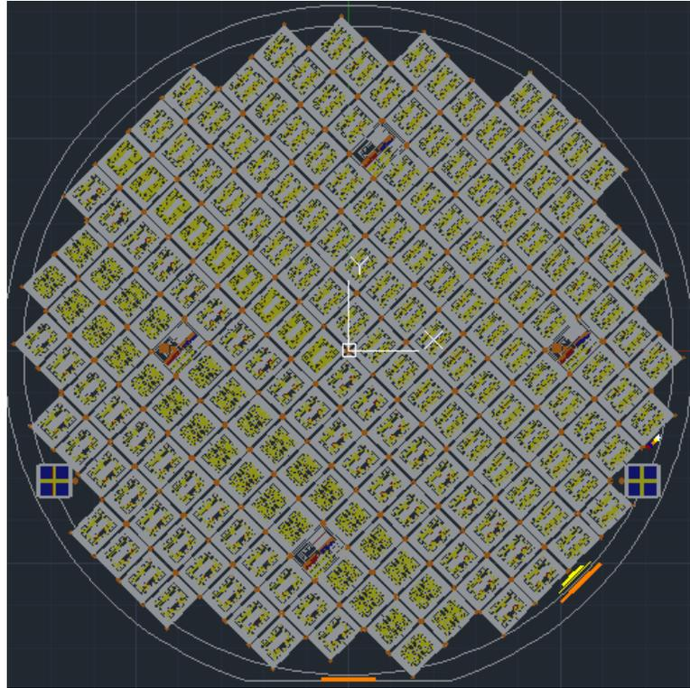
**Figure 3-9: Wafer layout.**
