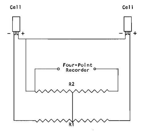
Fig. 4.-Photoelectric Cell Connections
