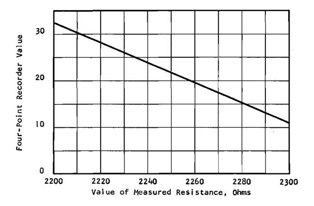
Fig. 2.-Calibration Curve for Resistance
