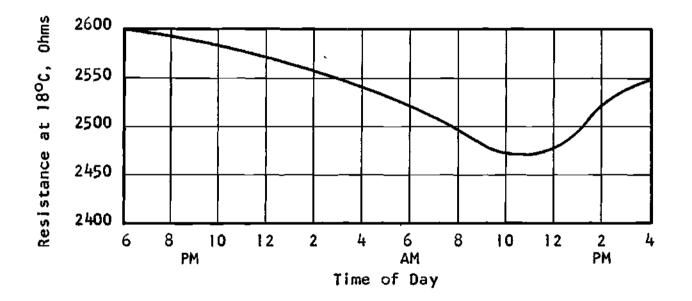
Fig. 7.-Variations in Resistance at Chattahoochee Pumping Station, June 23 and 24, 1956
