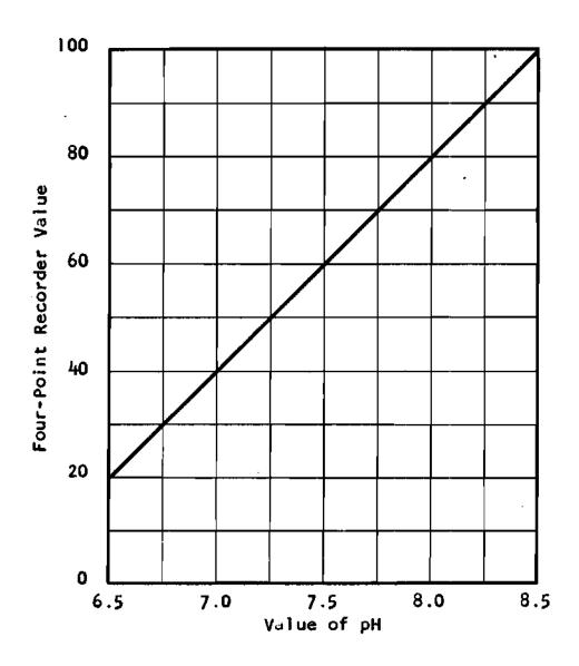
Fig. 1.-Calibration Curve for pH
