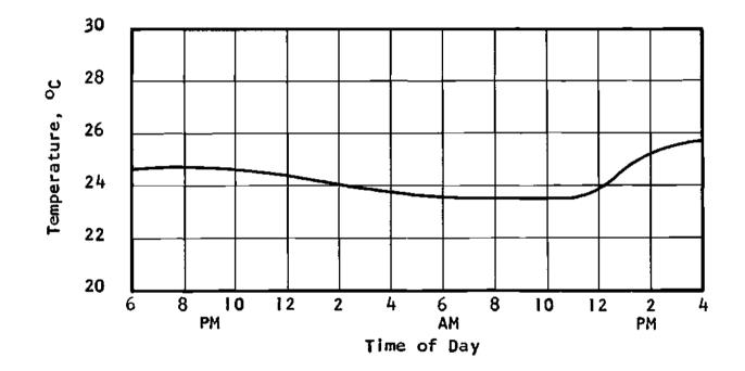
Fig. 9.-Variations in Temperature at Chattahoochee Pumping Station, June 23 and 24, 1956
