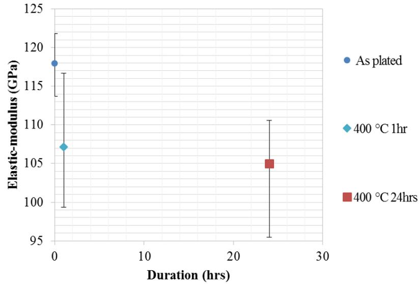
**Figure 6.14: Average elastic modulus values before and after 400 °C annealing of different durations**
