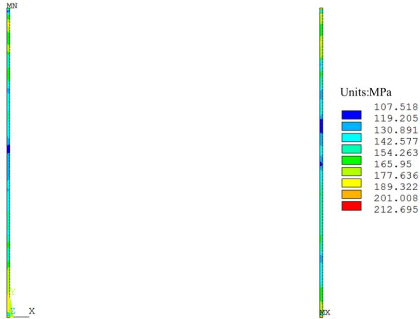
**Figure 7.11: 1<sup>st</sup> principal stress in dielectric layer**
