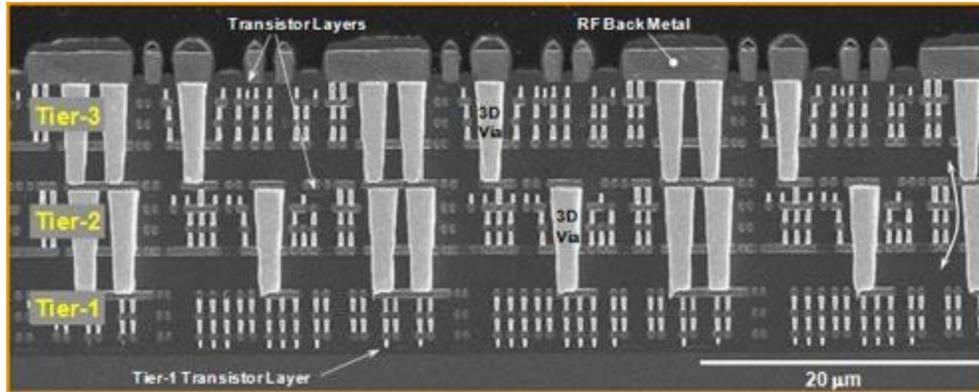
**Figure 1.7: 3D silicon integration (Source: MIT)**
