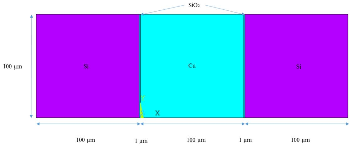
**Figure 7.4: 2D isotropic copper model of copper trench with 100 μm silicon**
