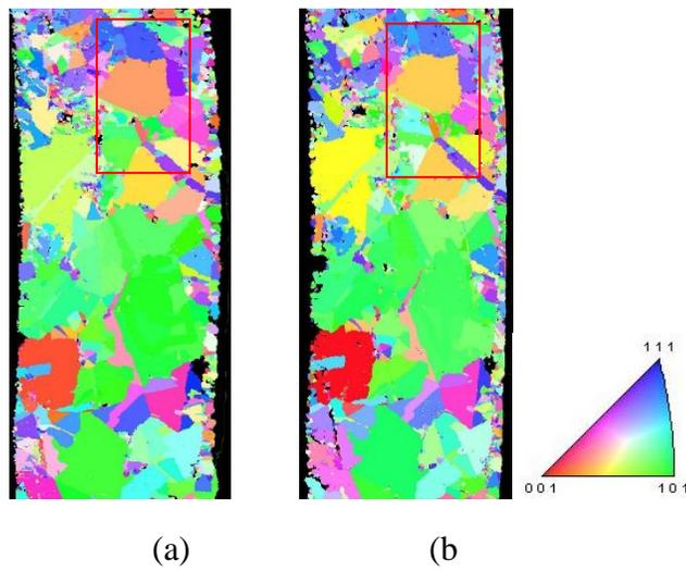
**Figure 5.17: EBSD images: (a) aged at room temperature for one year, and (b) annealed at 400 °C for 180 minutes**
