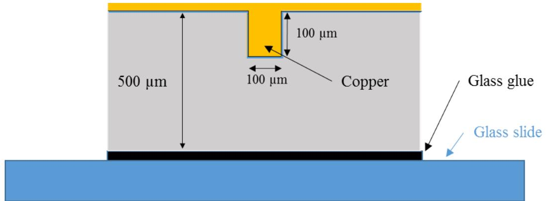
**Figure 7.1: Schematic of copper-plated silicon trench**
