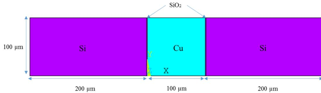
**Figure 7.2: 2D isotropic copper model of copper trench with 200 μm silicon**
