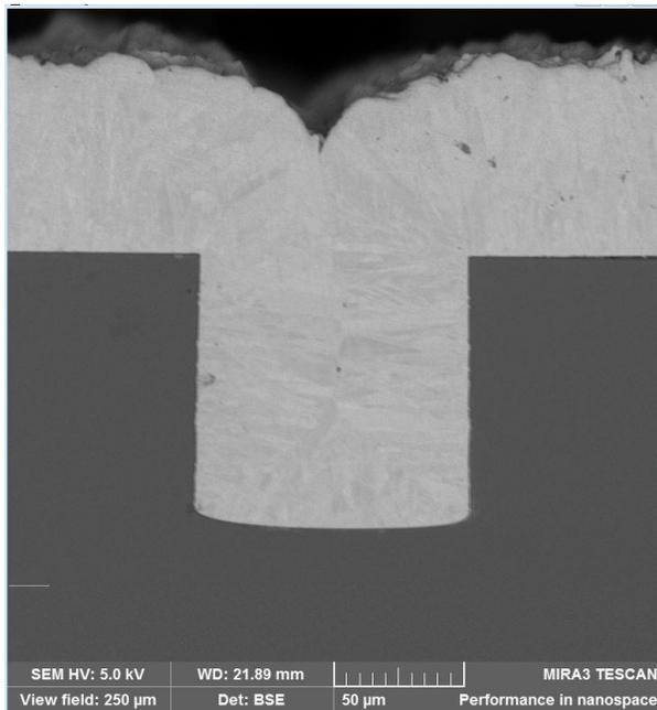
**Figure 4.9: SEM cross-section view of a copper-plated silicon trench**
