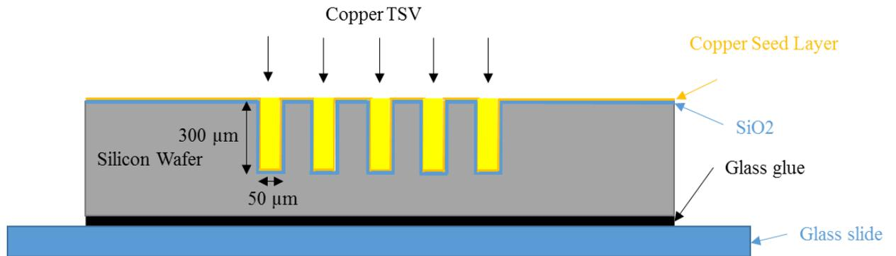
**Figure 5.1: Schematic view of copper TSVs cross-section view**
