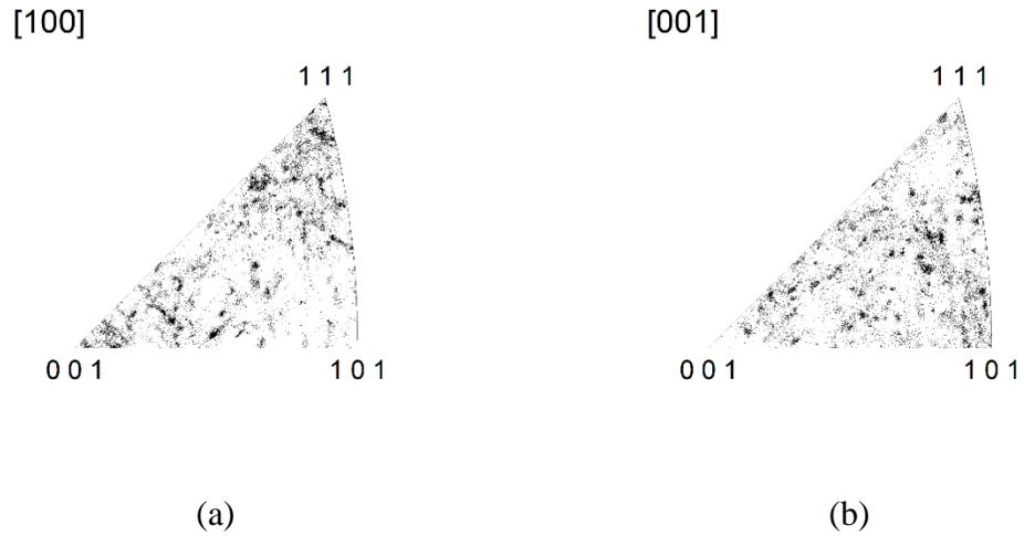
**Figure 6.24: Inverse pole figures for as-plated sample (a) parallel to the copper-plated silicon trench and (b) normal to the copper-plated silicon trench**
