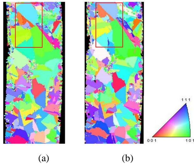
**Figure 5.18: EBSD images: (a) aged at room temperature for one year, and (b) annealed at 500 °C for 180 minutes**
