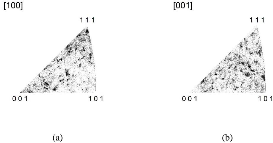
**Figure 6.28: Inverse pole figures for annealed at 450 °C for 35.5 hours (a) parallel to the copper-plated silicon trench and (b) normal to the copper-plated silicon trench**
