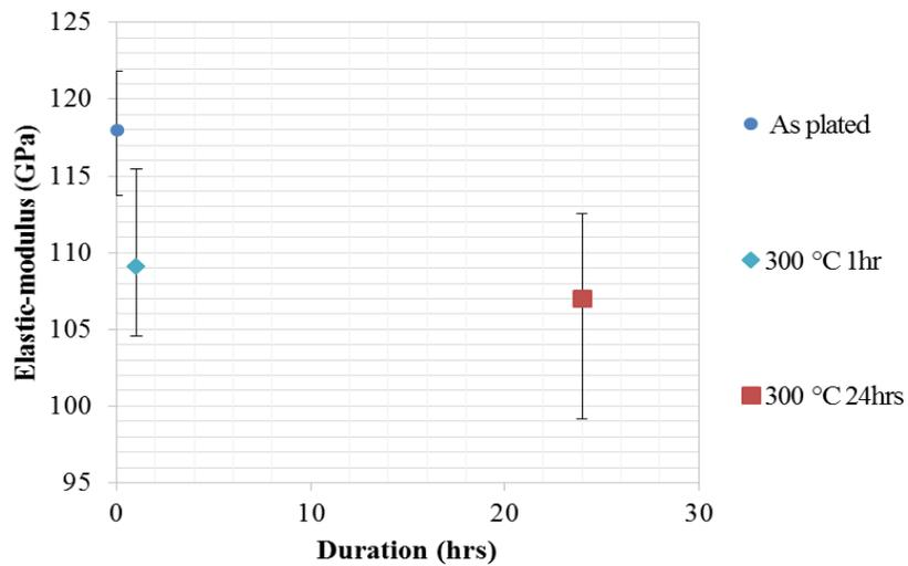
**Figure 6.13: Average elastic modulus values before and after 300 °C annealing of different durations**
