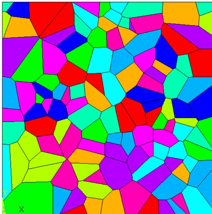
**Figure 7.13: Voronoi algorithm generated 125 grains**
