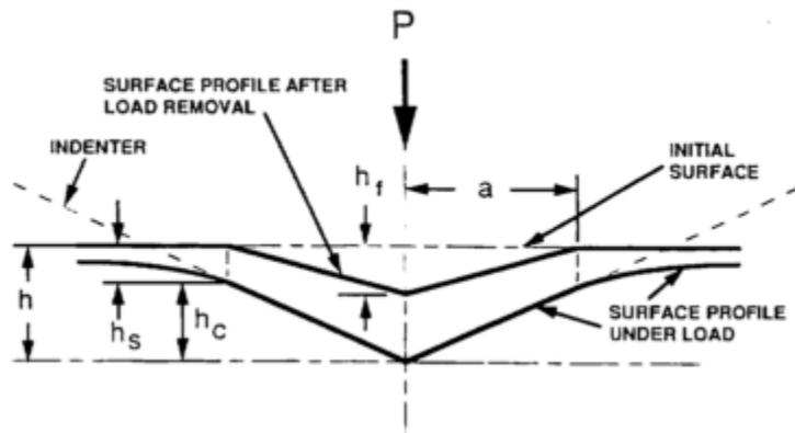
**Figure 5.8: A schematic representation of a section through an indentation showing various quantities used in the analysis [Source: Oliver] [85]**
