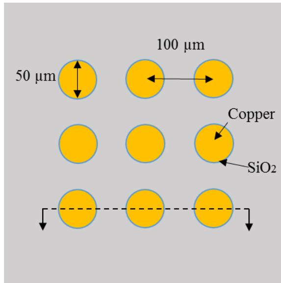
**Figure 4.1: Top view of copper filled TSVs**
