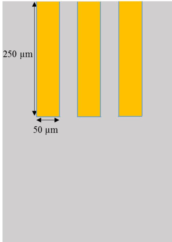
**Figure 4.2: Cross-section view of a copper filled TSVs**
