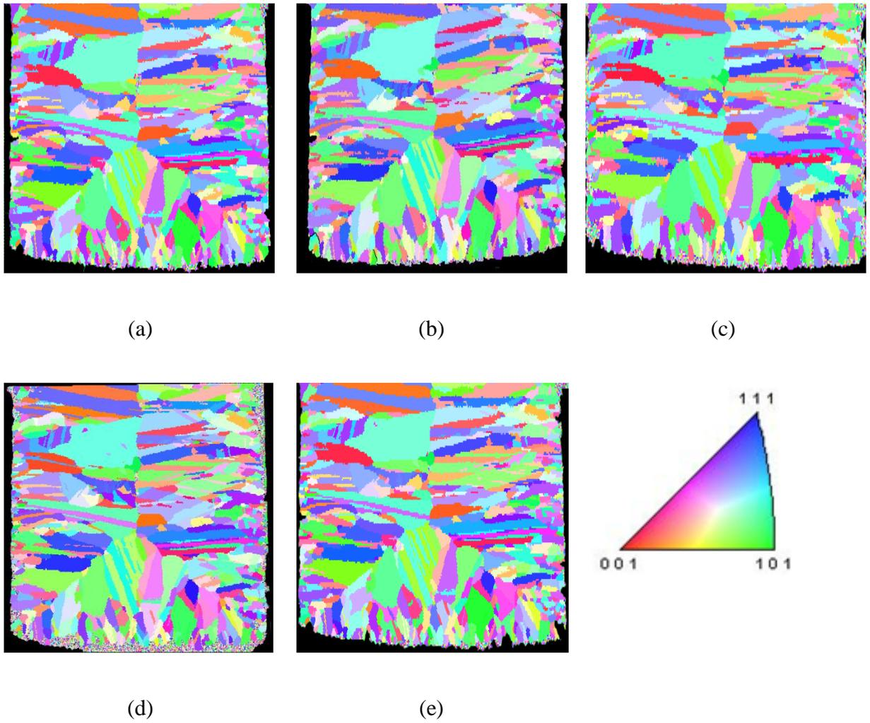
**Figure 6.18: EBSD images of annealing temperature is 300 °C (a) As-plated sample, (b) 30 minutes, (c) Additional 60 minutes, (d) Additional 10 hours, and (e) Additional 24 hours**
