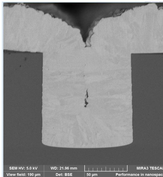
**Figure 4.10: Copper trench with a void in the center**
