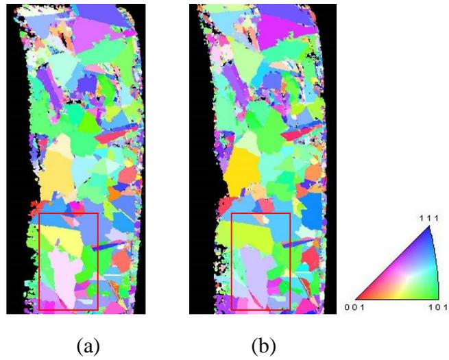
**Figure 5.16: EBSD images: (a) aged at room temperature for one year, and (b) annealed at 300 °C for 180 minutes**
