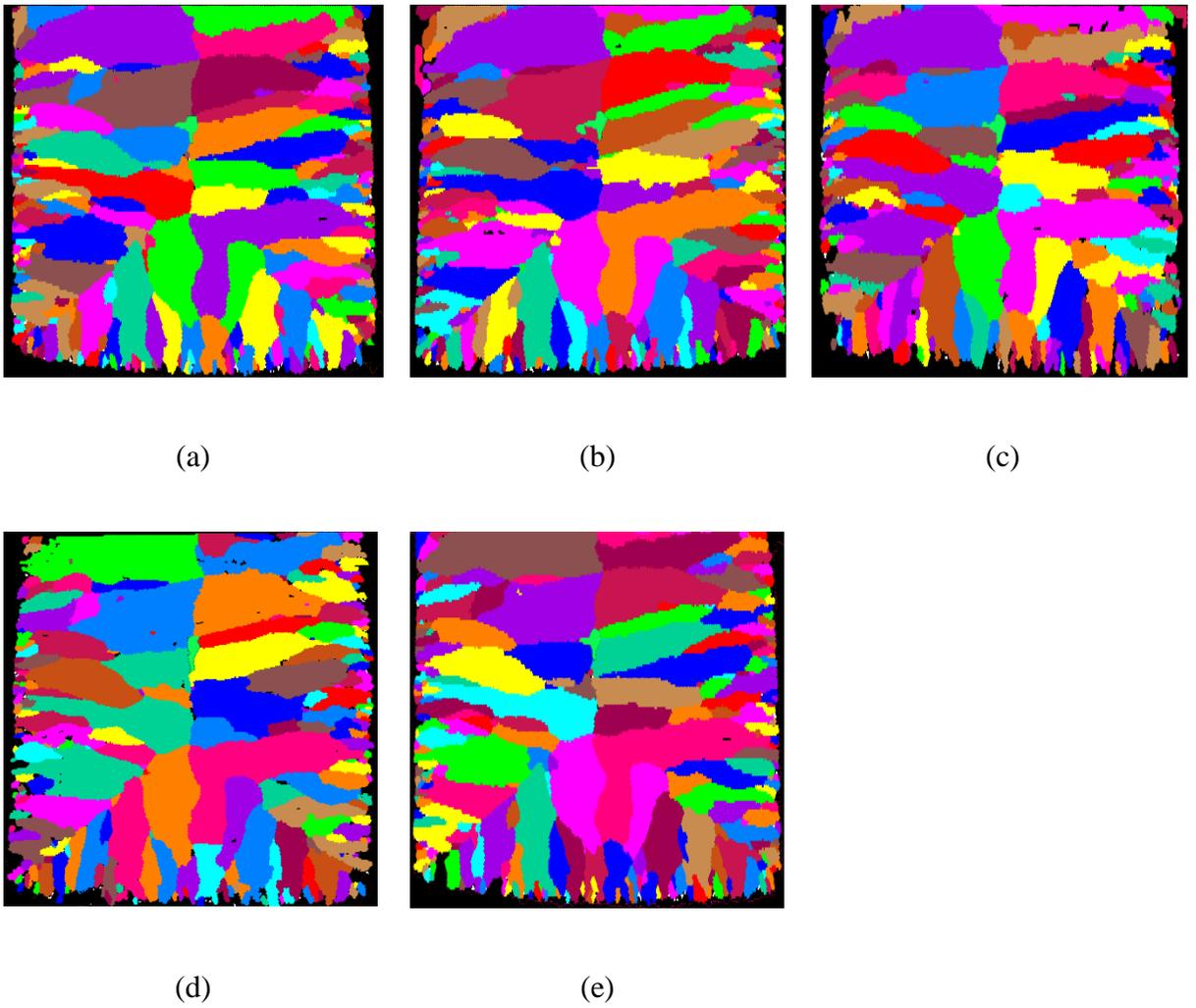
**Figure 6.19: Grain map of annealing temperature is 300 °C (a) As-plated sample, (b) 30 minutes, (c) Additional 60 minutes, (d) Additional 10 hours, and (e) Additional 24 hours**
