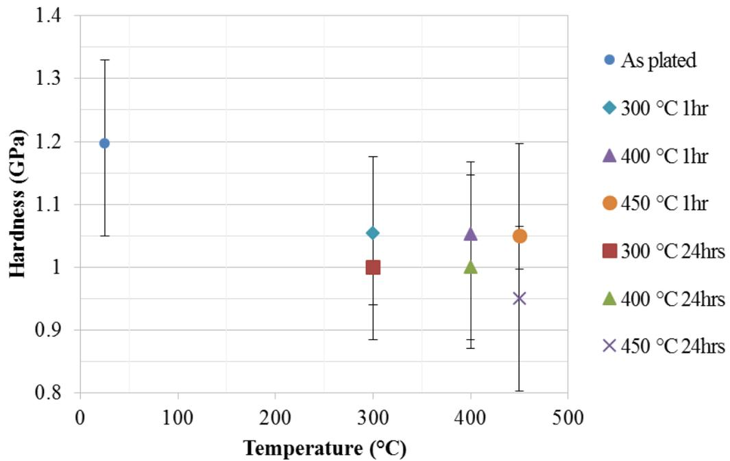
**Figure 6.8: Average hardness values before and after thermal annealing**
