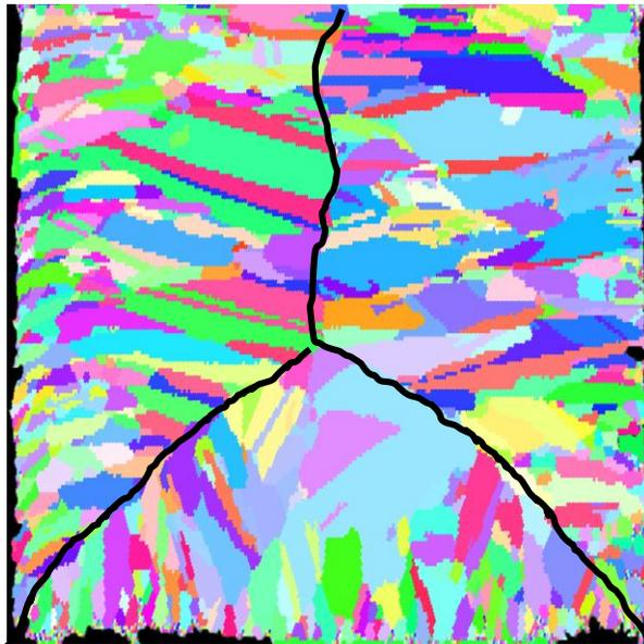
**Figure 6.16: EBSD images of as-plated sample shows grain orientation**
