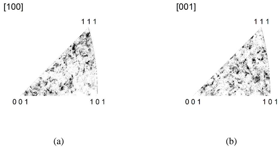
**Figure 6.25: Inverse pole figures for annealed at 450 °C for 30 minutes (a) parallel to the copper-plated silicon trench and (b) normal to the copper-plated silicon trench**
