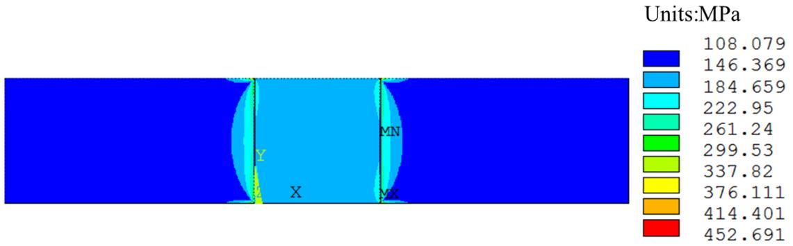
**Figure 7.3: von Mises stress in 2D model with 200 μm silicon**
