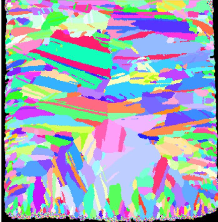
**Figure 7.8: EBSD image of the grain structure**
