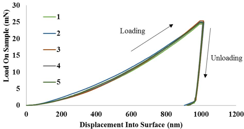
**Figure 6.7: Displacement into surface and load on sample of annealed sample for 1 hour at 450°C**
