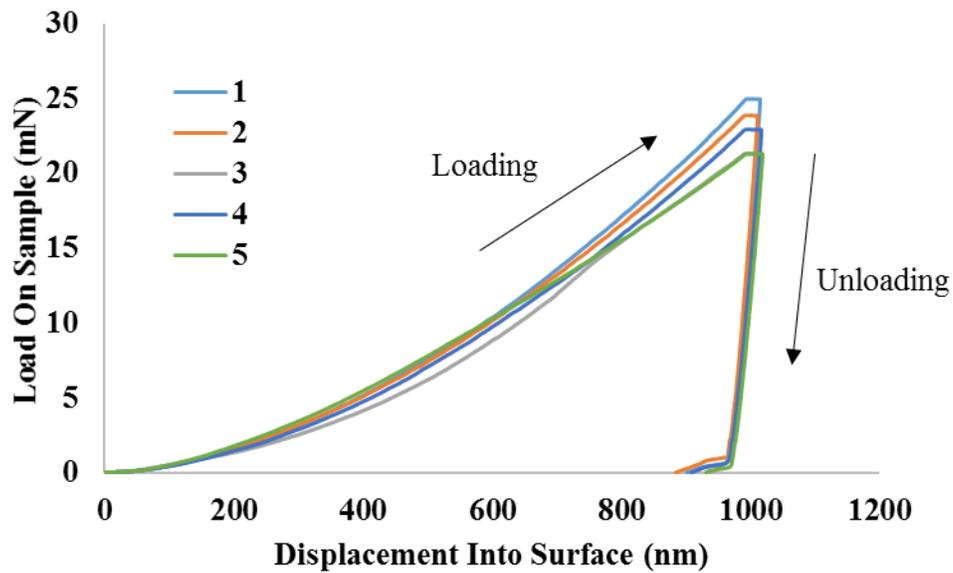
**Figure 6.6: Displacement into surface and load on sample of annealed sample for 1 hour at 400°C**
