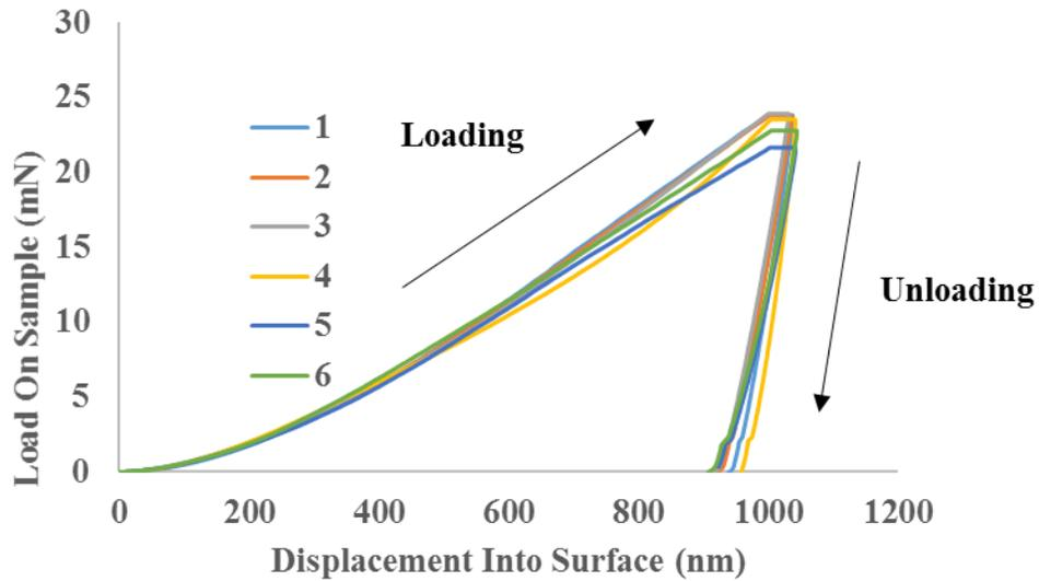
**Figure 5.10: Displacement into surface and load on sample**
