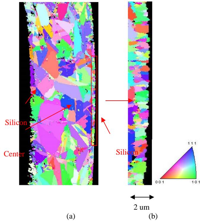
**Figure 5.20: EBSD images: (a) aged at room temperature for one year, and (b) detail of edge**
