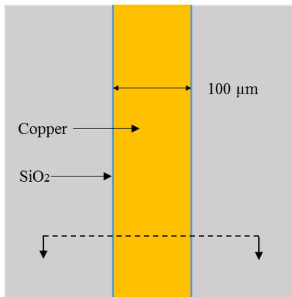
**Figure 4.3: Top-view of a copper trench**
