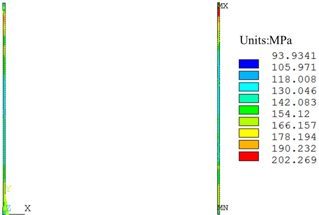
Figure 7.15: 1<sup>st</sup> principal stress in dielectric layer
