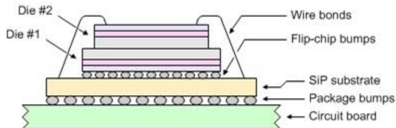
**Figure 1.4: 3D IC System in package (Source: Clive Maxfield)**
