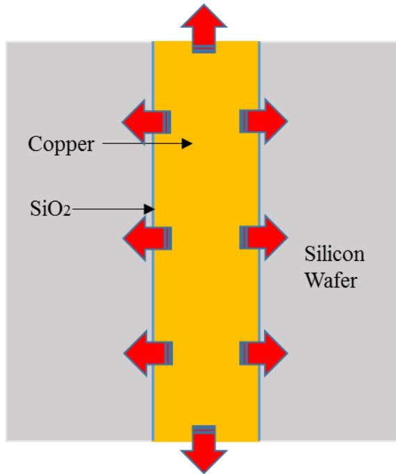
**Figure 1.9: CTE mismatch induced stress in TSV structure**
