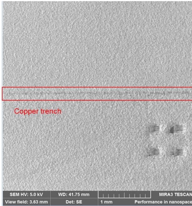
**Figure 4.8: Fabricated copper trench**
