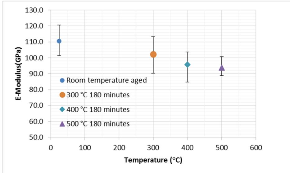
**Figure 5.12: Average elastic modulus values before and after high-temperature annealing**
