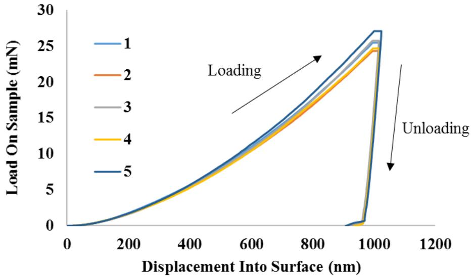
**Figure 6.5: Displacement into surface and load on sample of annealed sample for 1 hour at 300°C**
