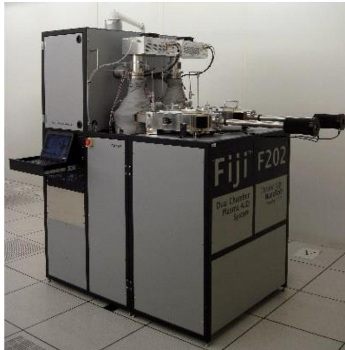
**Figure 5.5: Cambridge Fiji Plasma® atomic layer deposition (ALD) tool**
