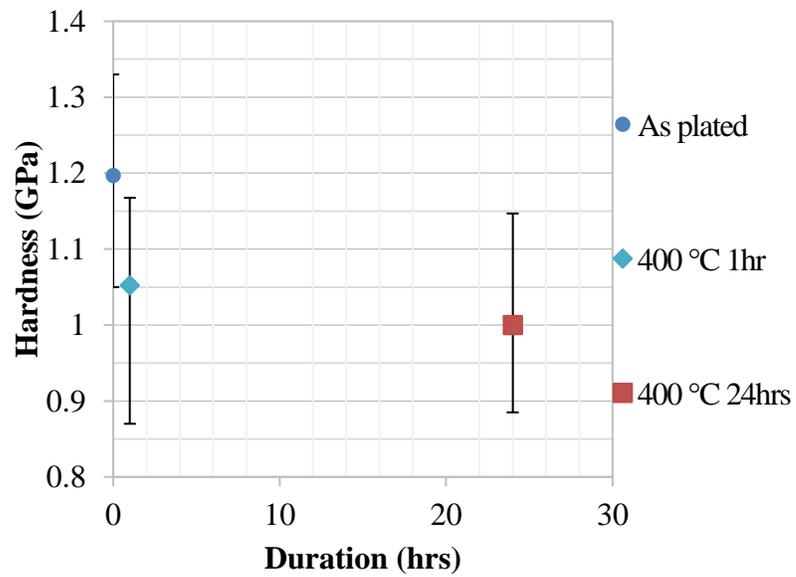
**Figure 6.10: Average hardness values before and after 400 °C annealing of different durations**
