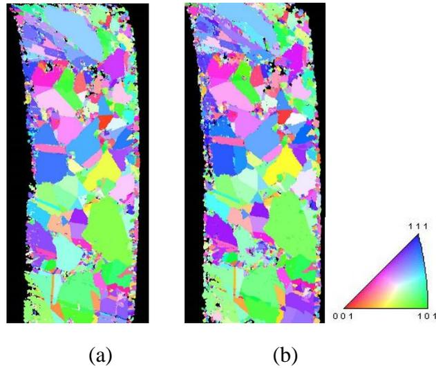
**Figure 5.19: EBSD images: (a) aged at room temperature for one year, and (b) annealed at 400 °C for 30 hours**
