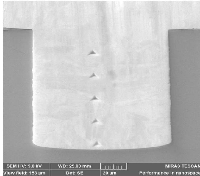
**Figure 6.3: SEM image showing the indentation spots along the axis of a polished copper plated silicon trench**
