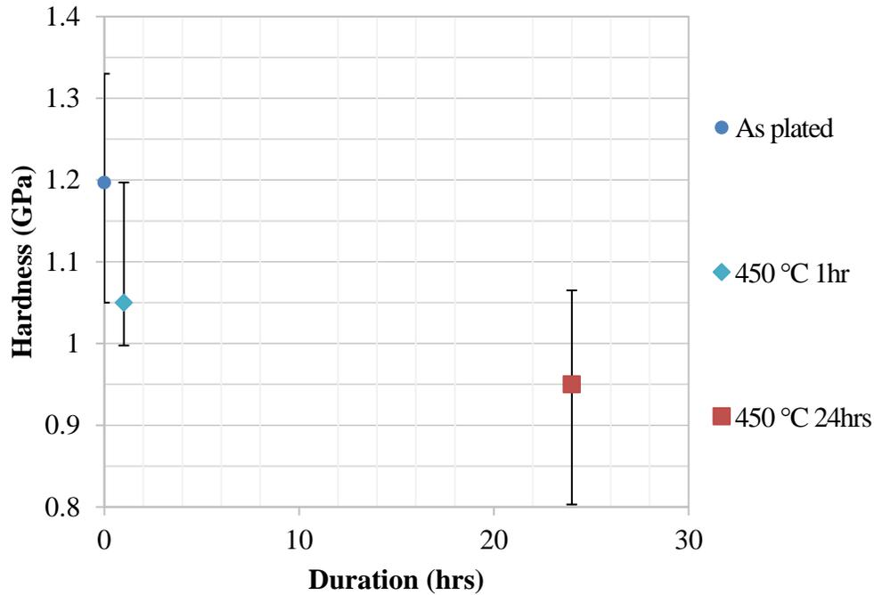
**Figure 6.11: Average hardness values before and after 450 °C annealing of different durations**
