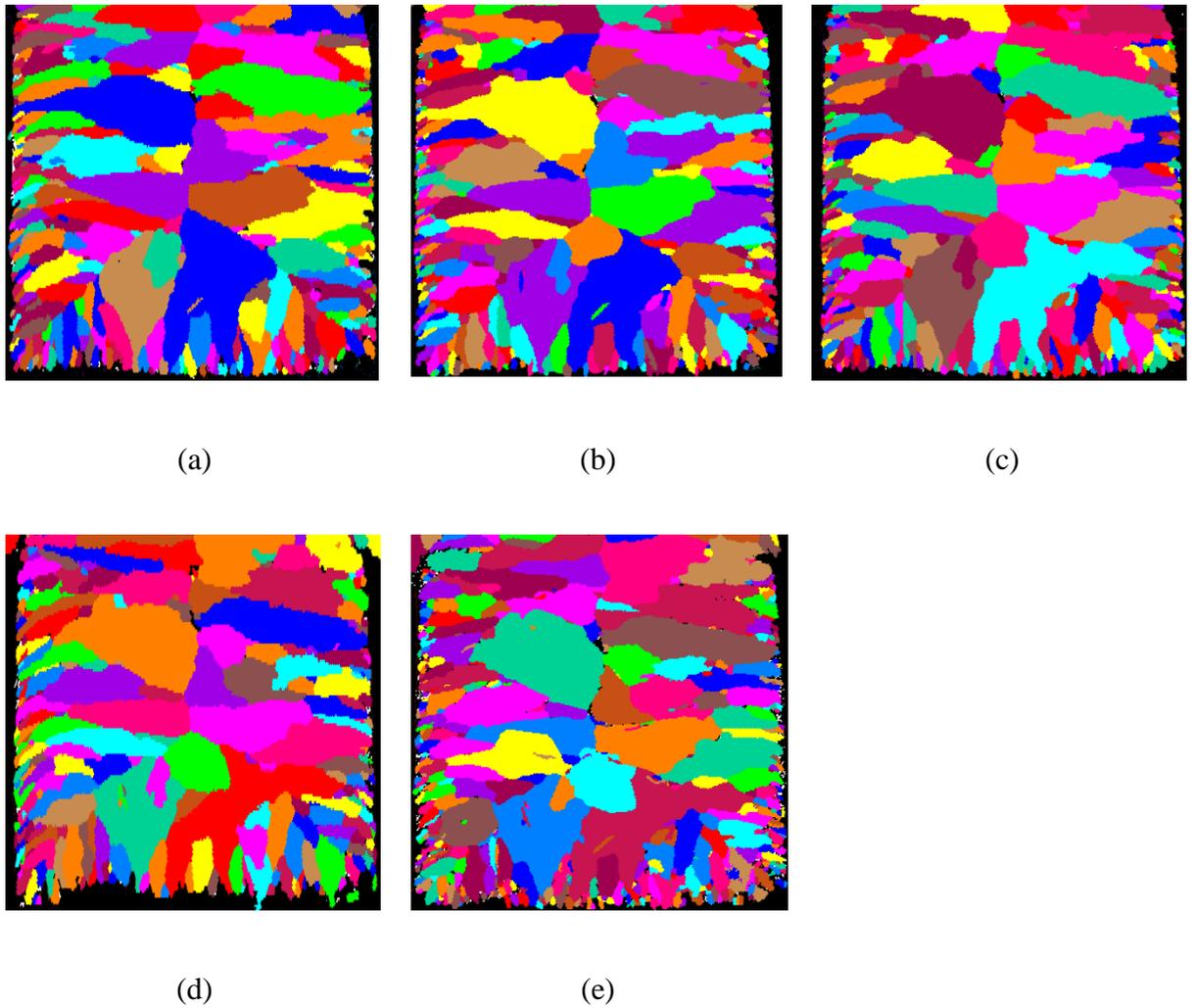
**Figure 6.23: Grain map of annealing temperature is 450 °C (a) As-plated sample, (b) 30 minutes, (c) Additional 60 minutes, (d) Additional 10 hours, and (e) Additional 24 hours**
