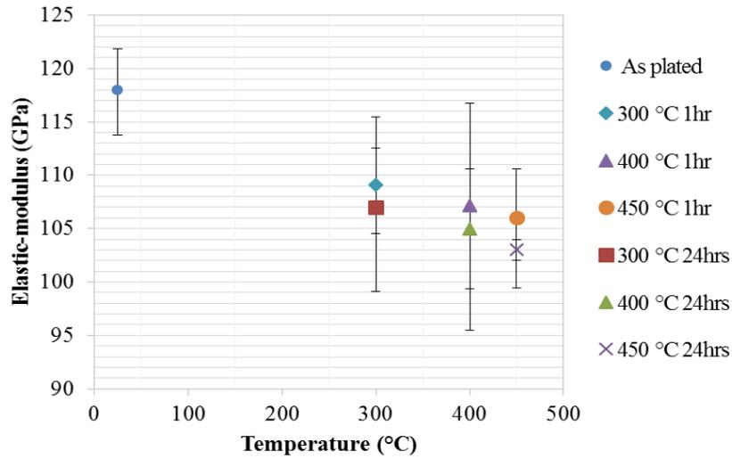
**Figure 6.12: Average elastic-modulus values before and after high-temperature annealing**
