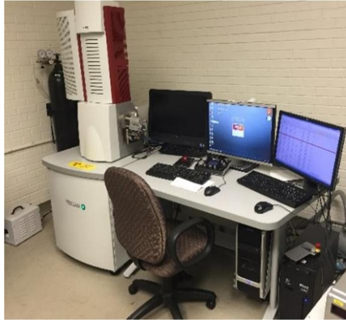
**Figure 5.13: TESCAN® SEM with an EBSD detector**
