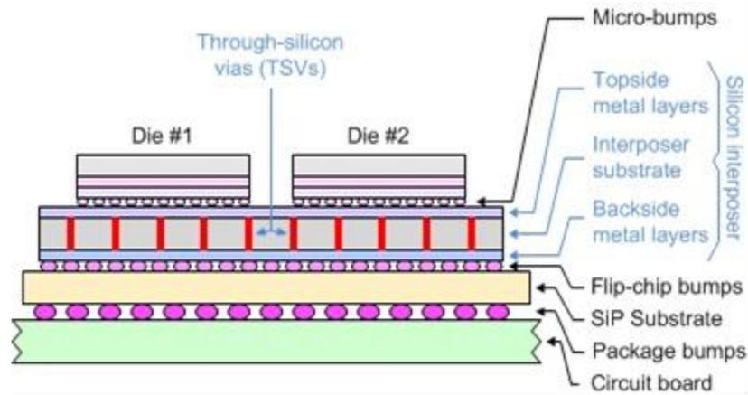
**Figure 1.3: 2.5D IC System in package (Source: Clive Maxfield)**
