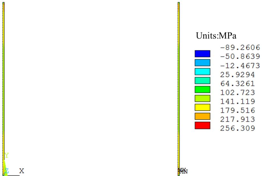
Figure 7.6: 1<sup>st</sup> principal stress in dielectric layer
