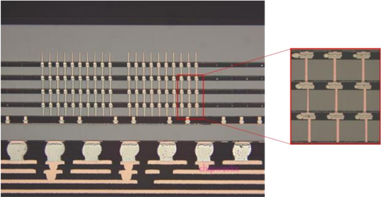
**Figure 1.5: Die stack with TSVs (Source: SK Hynix)**
