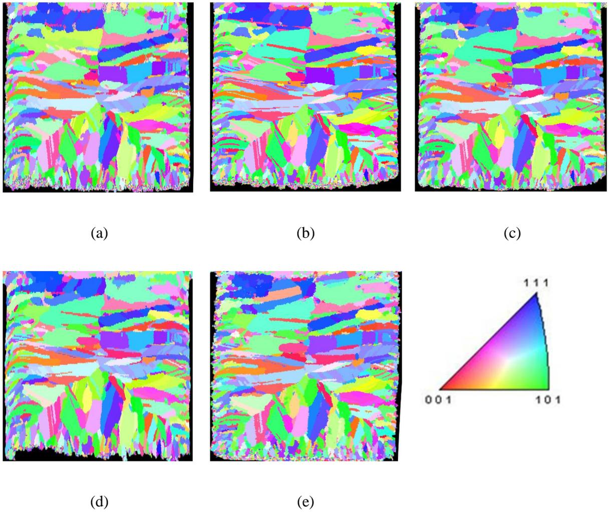
**Figure 6.20: EBSD images of annealing temperature is 400 °C (a) As-plated sample, (b) 30 minutes, (c) Additional 60 minutes, (d) Additional 10 hours, and (e) Additional 24 hours**
