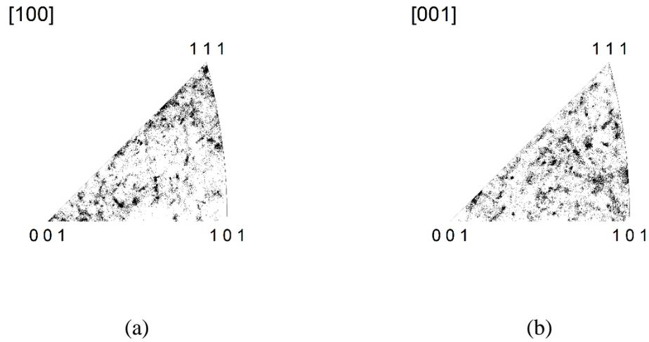
**Figure 6.26: Inverse pole figures for annealed at 450 °C for 1.5 hours (a) parallel to the copper-plated silicon trench and (b) normal to the copper-plated silicon trench**
