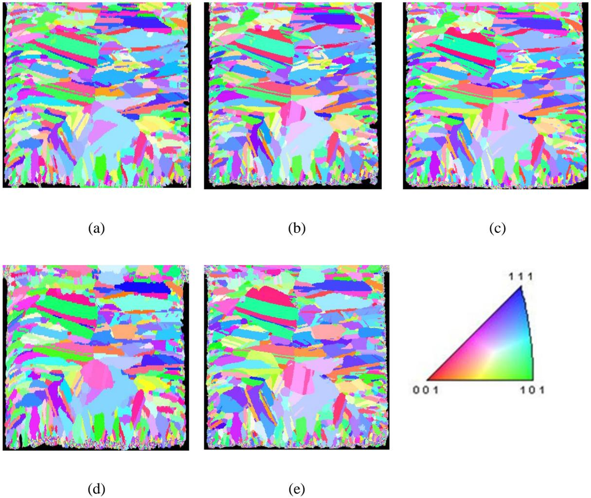
**Figure 6.22: EBSD images of annealing temperature is 450 °C (a) As-plated sample, (b) 30 minutes, (c) Additional 60 minutes, (d) Additional 10 hours, and (e) Additional 24 hours**
