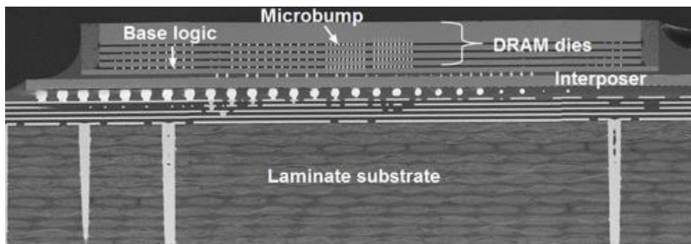
**Figure 1.8: Substrate and interposer layer and stacked DRAM of high bandwidth memory (Source: Hynix)**
