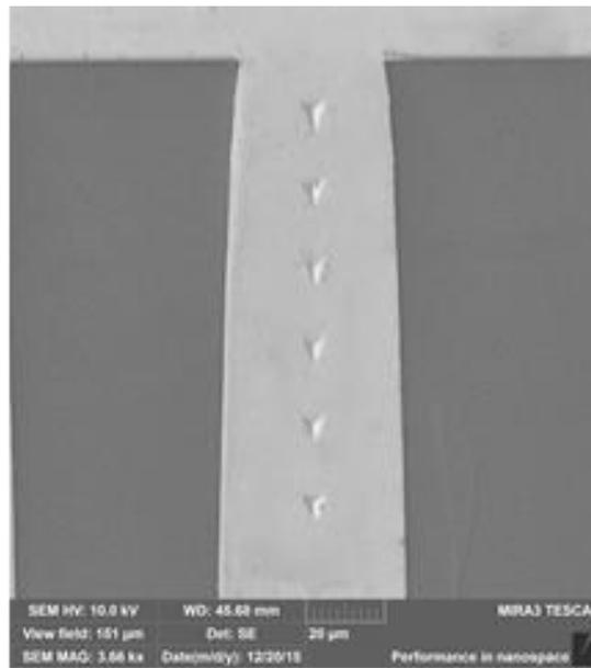
**Figure 5.7: SEM image showing the indentation spots along the axis of a polished blind TSV**
