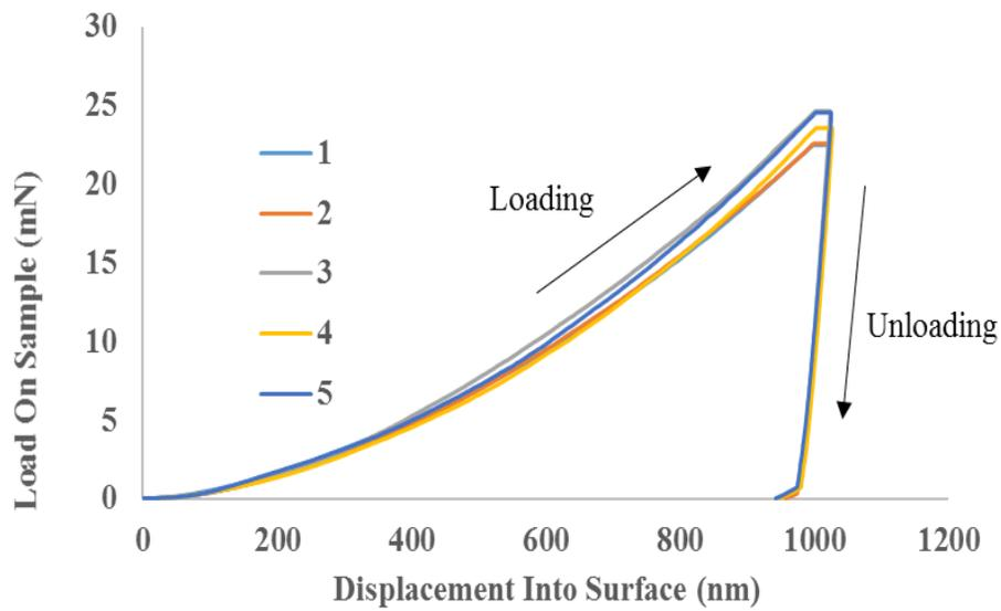
**Figure 6.4: Displacement into surface and load on sample of as-plated sample**
