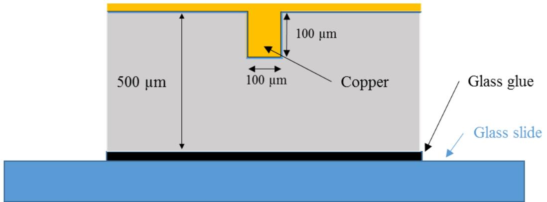
**Figure 6.1: Schematic of copper-plated silicon trench**
