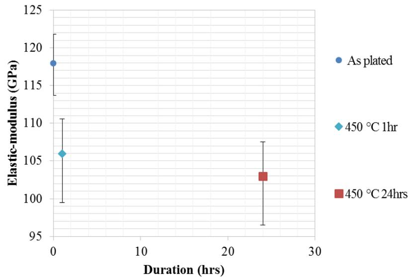
**Figure 6.15: Average elastic modulus values before and after 450 °C annealing of different durations**
