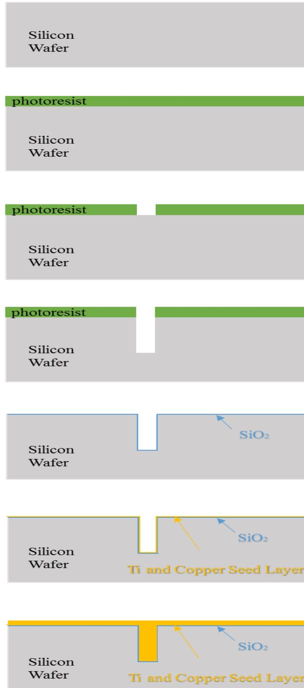
**Figure 4.5: Process flow to fabricate copper filled TSVs**
