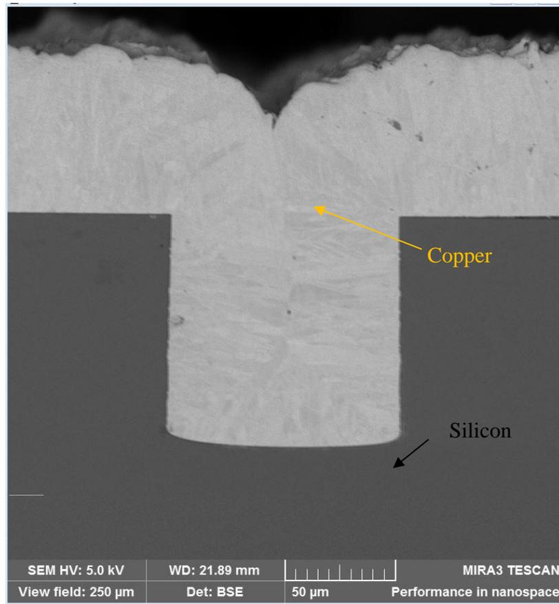
**Figure 6.2: SEM cross-section of a copper-plated silicon trench**
