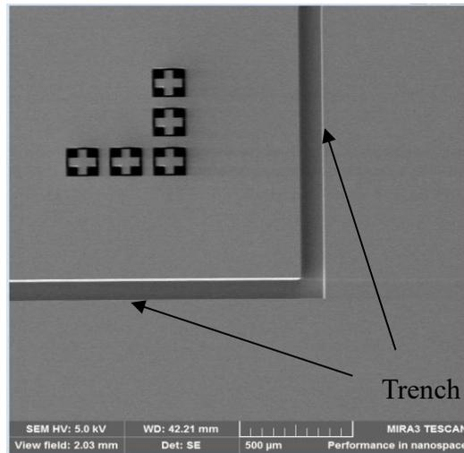
**Figure 4.7: Top-view of silicon trench**
