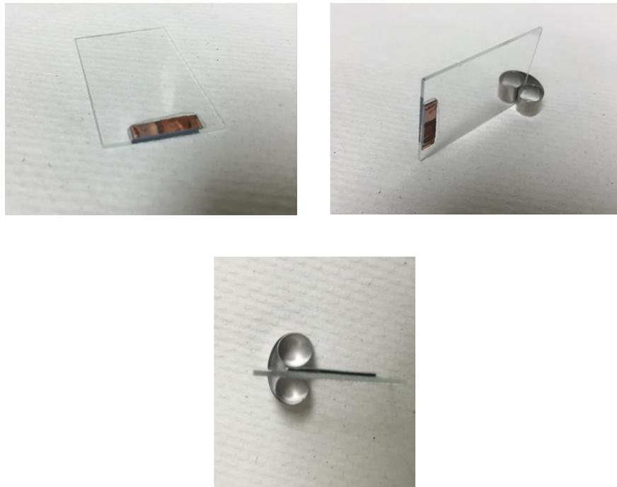
**Figure 5.2: Copper TSVs glued to glass slide**
