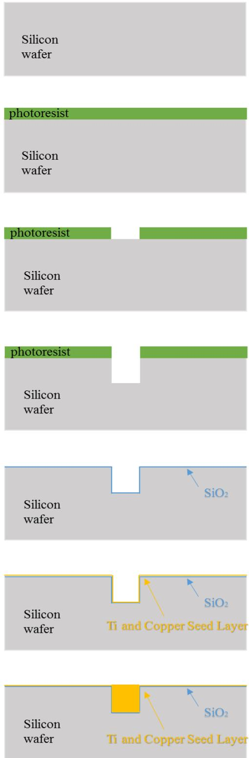
**Figure 4.6: Process flow to fabricate copper trenches**
