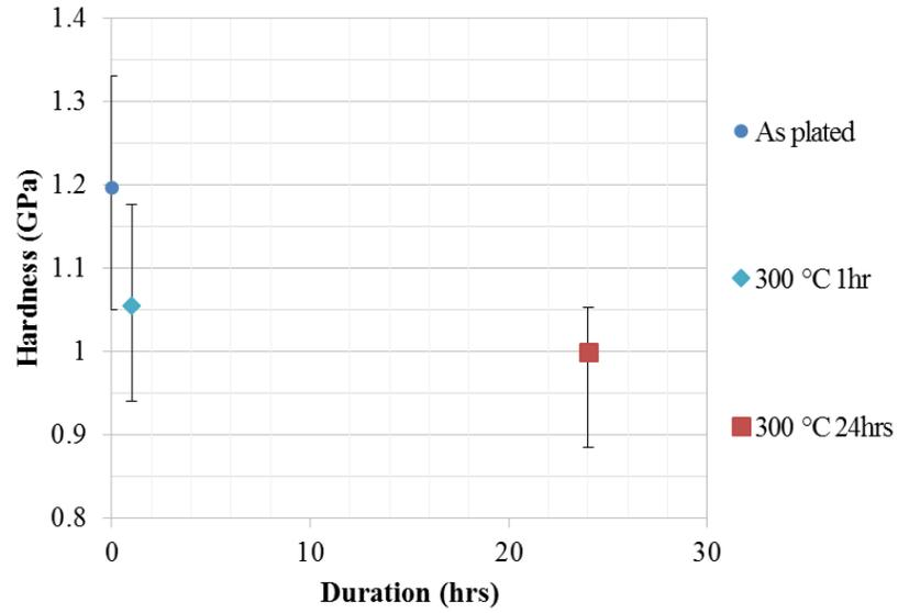
**Figure 6.9: Average hardness values before and after 300 °C annealing of different durations**
