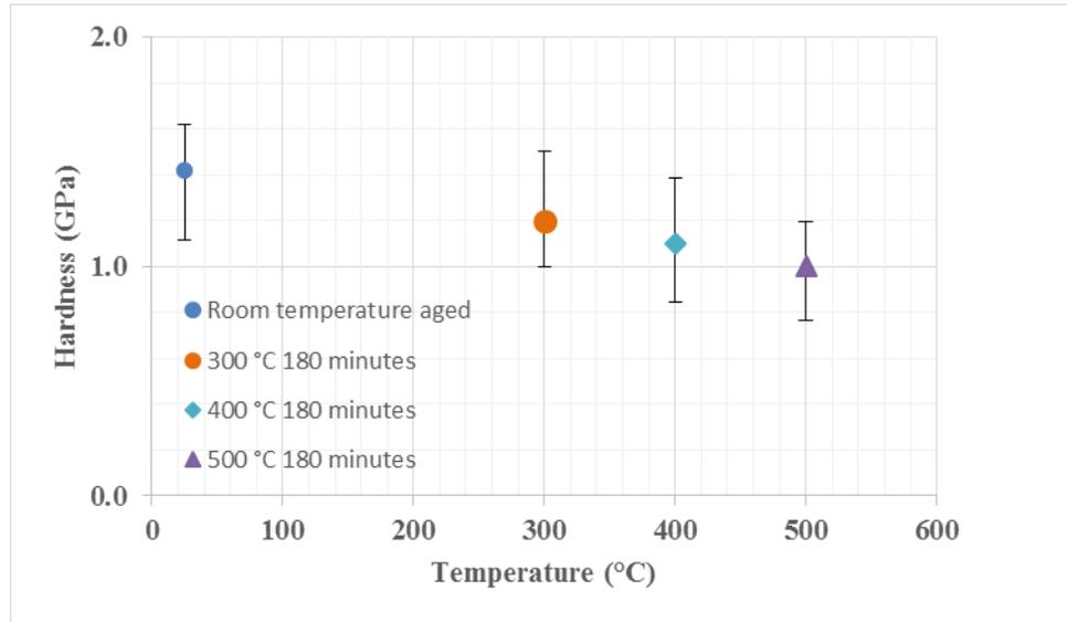
**Figure 5.11: Average hardness values before and after high-temperature annealing**
