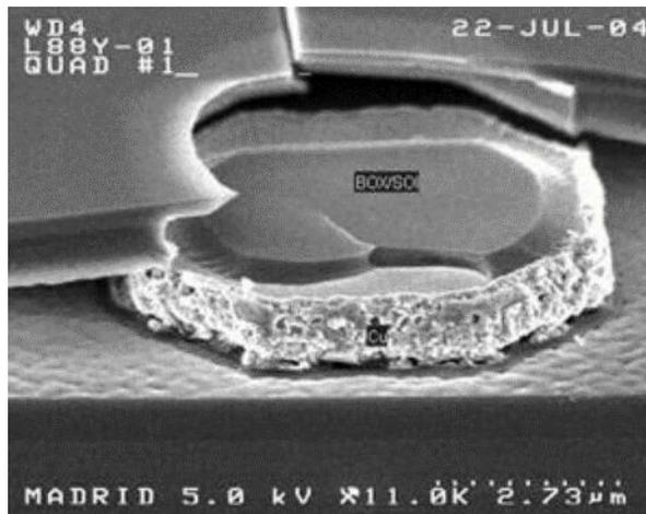
**Figure 1.10: CTE mismatch induced dielectric cracking (Source: Tezzaron)**
