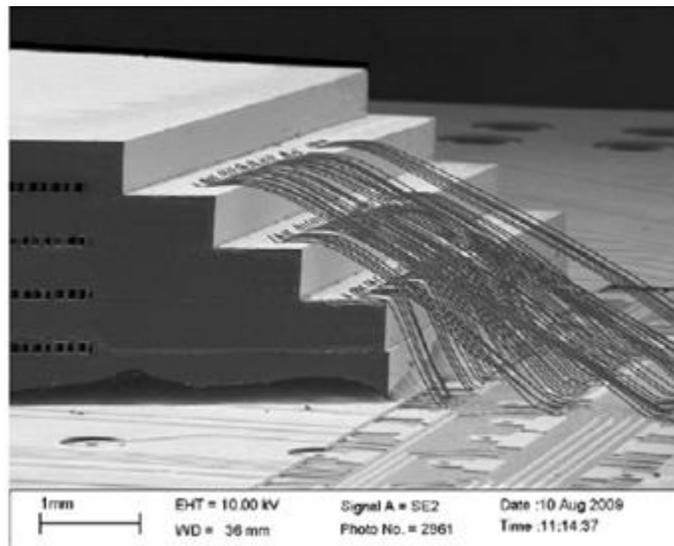
**Figure 1.6: Die stack with wire bonds (Sources: ESL)**
