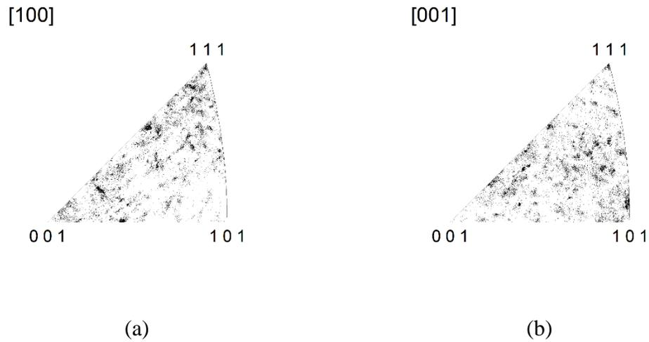
**Figure 6.27: Inverse pole figures for annealed at 450 °C for 11.5 hours (a) parallel to the copper-plated silicon trench and (b) normal to the copper-plated silicon trench**
