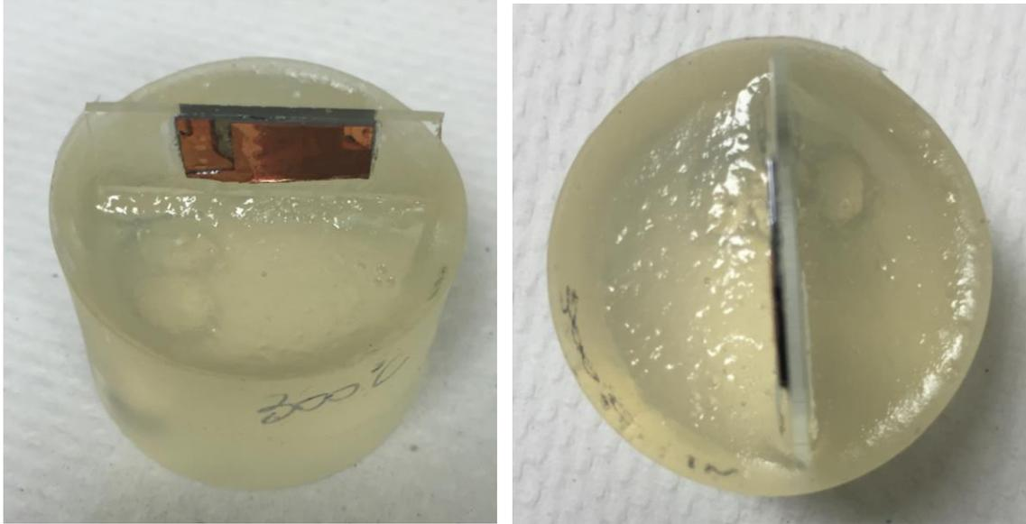
**Figure 5.6: Images showing the sample before indentation**
