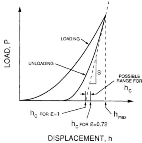
**Figure 5.9: A schematic representation of load versus indenter displacement showing quantities used in the analysis as well as a graphical interpretation of the contact depth [Source: Oliver] [85]**
