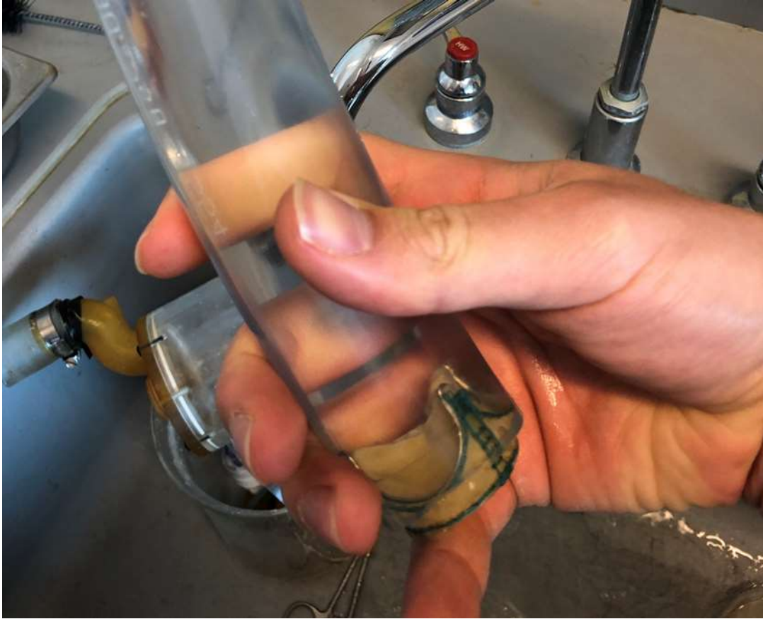
Figure C-7. Image of GT-TAV leak test with a plastic tube full of water and a 29 mm GT-TAV plugging the bottom. Note: the valve shows good coaptation.
