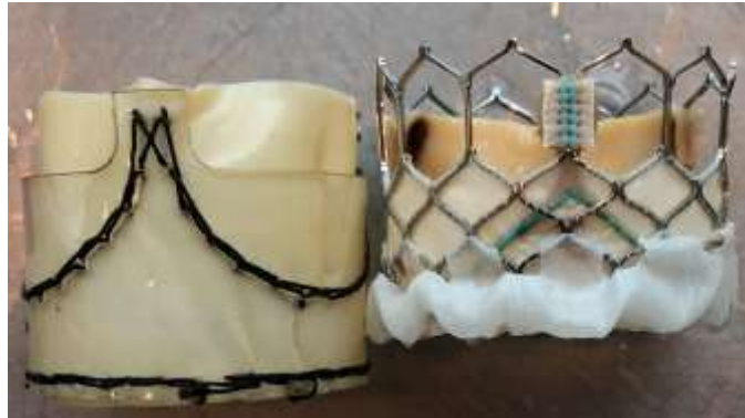
Figure 5-7. Open 29mm GT-TAV without retaining ring alongside closed 29mm SAPIEN 3. The extra length at the bottom of the GT-TAV is for assembly purposes and is accounted for with regards to deployment height.
