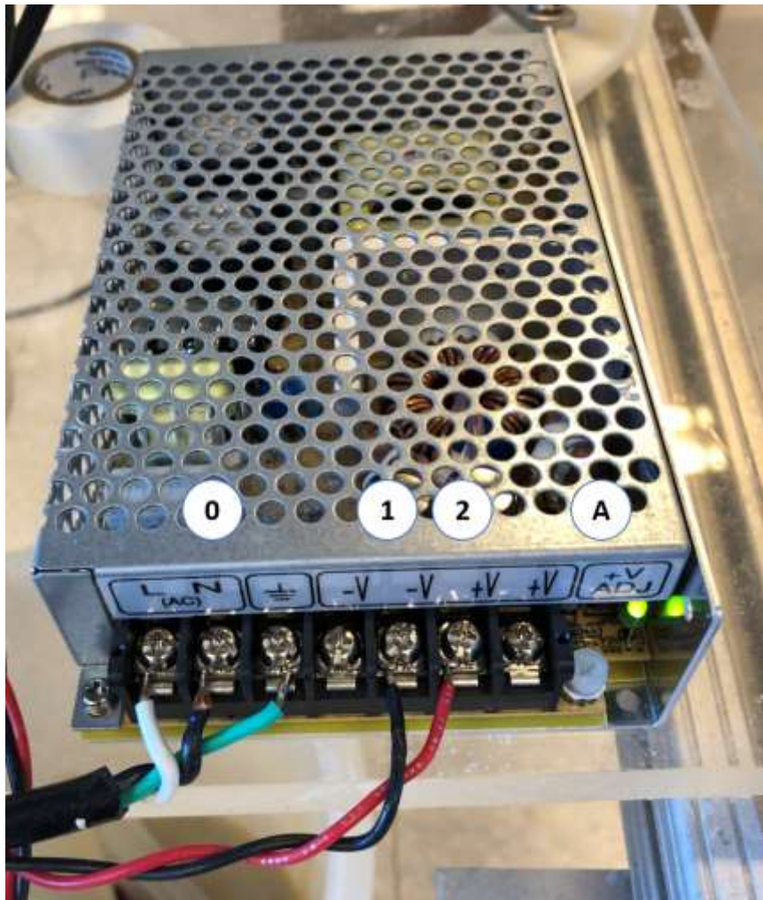
Figure A-2. Single power supply wiring figure. See for Table A-1 details.
