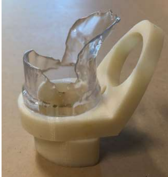
Figure 5-4. 3-D printed LV insert with Long AML, 0% LAMPOON 3-D printed MV glued in place.
