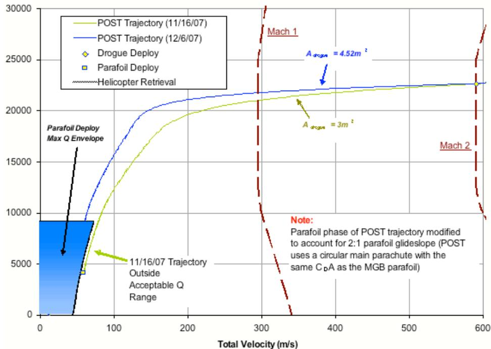
Figure 11. Trajectory Showing Parachute Deployment Conditions and Allowable Inflation Conditions
