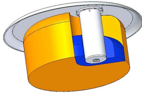
**Figure 13. Mortar and Parafoil Integrated into Aftbody**
