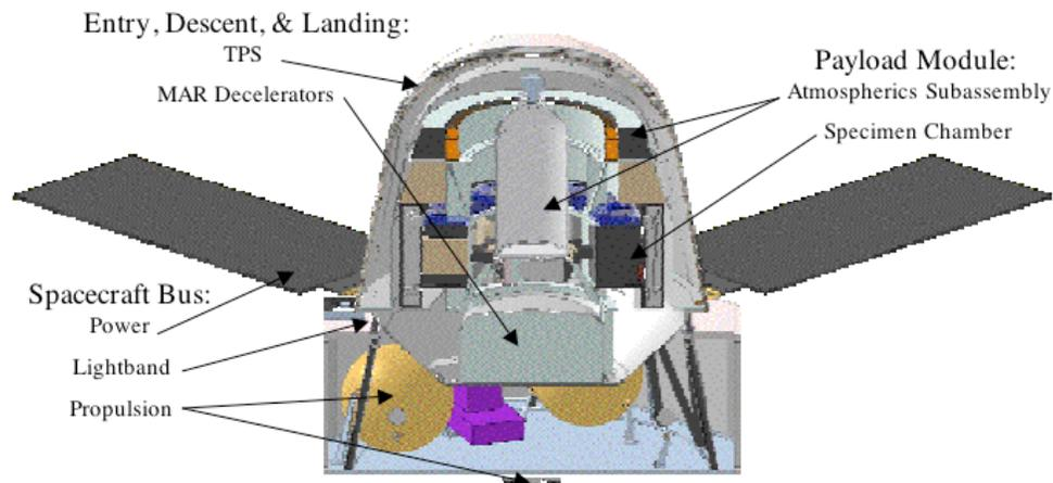
**Figure 1. Mars Gravity Biosatellite: Bus, Payload, EDL**
