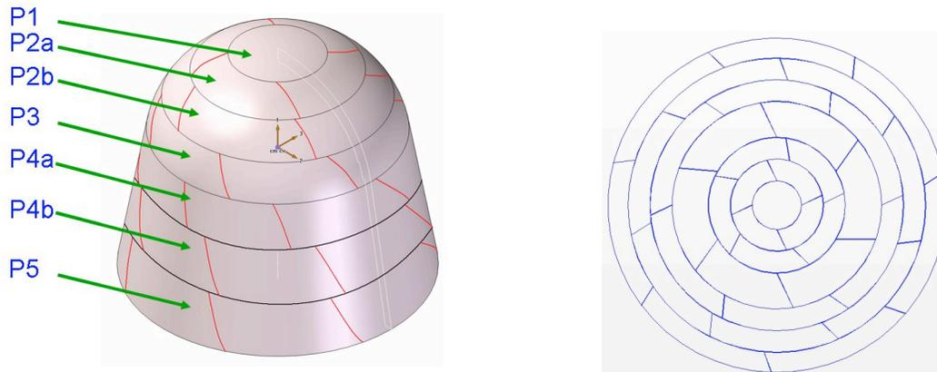
**Figure 9. Heatshield Tile Layout (3D View and Top View)**
