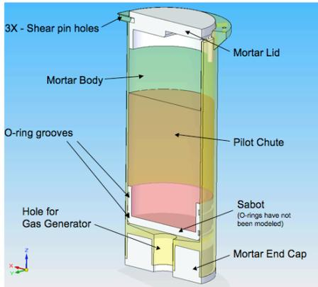
**Figure 12. Mortar Assembly with Pilot and Drogue**
