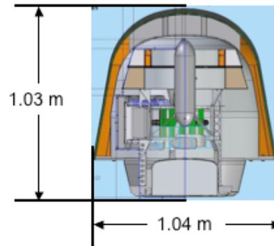
Figure 3. Entry Vehicle Cutaway
