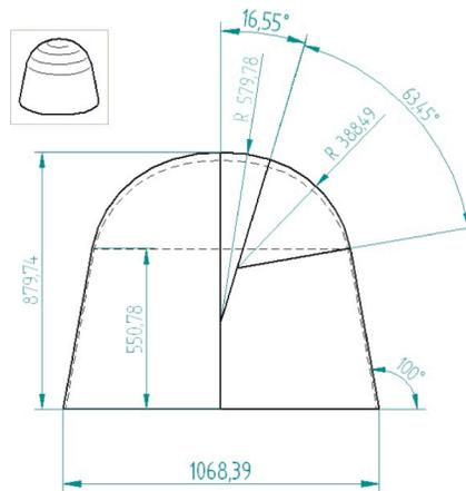
Figure 5. Discoverer Aeroshell Geometry (base dimensions in mm)
