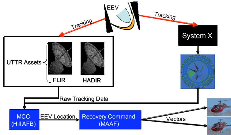
**Figure 14. Data Flow During Recovery Operations**
