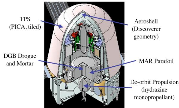
Figure 2. EDL Subsystems
