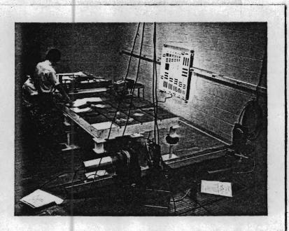
Figure 3. Modulation transfer function analyzer (foreground) and resolution chart experiments in the optical testing laboratory.
