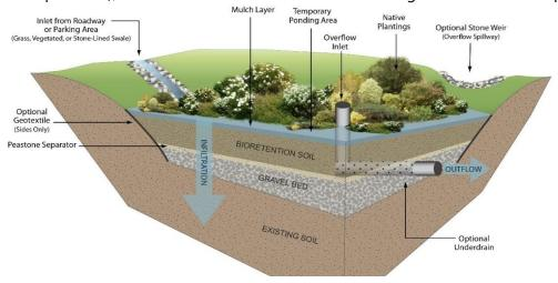
Diagram of Typical Bioretention Pond (Massachusetts DEP, n.d.)
