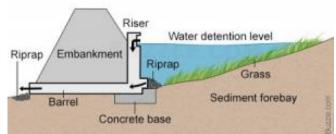
Diagram of Typical Stormwater Detention Pond (Hughes, 2016)
