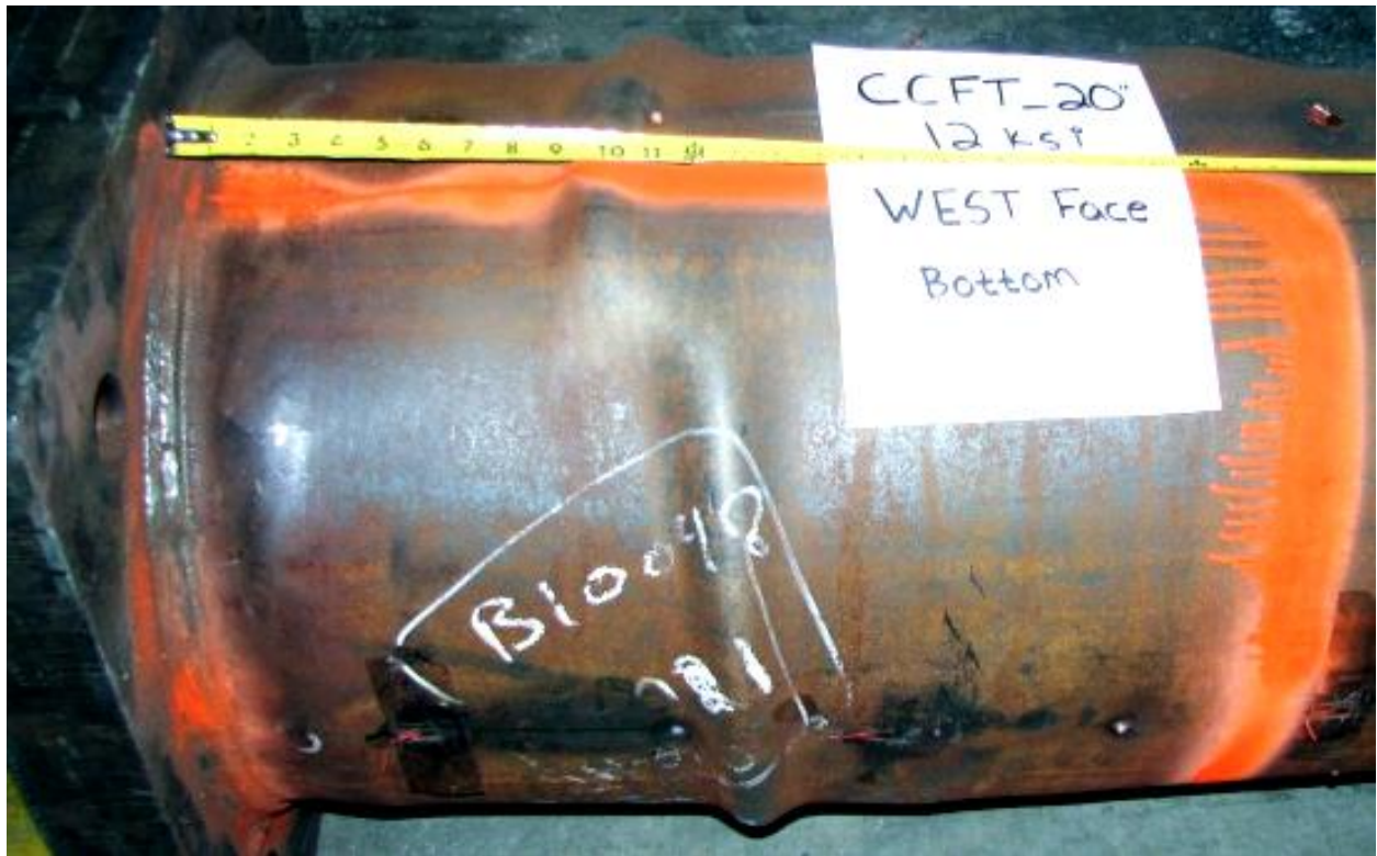
(a) Local buckling deformation in steel
