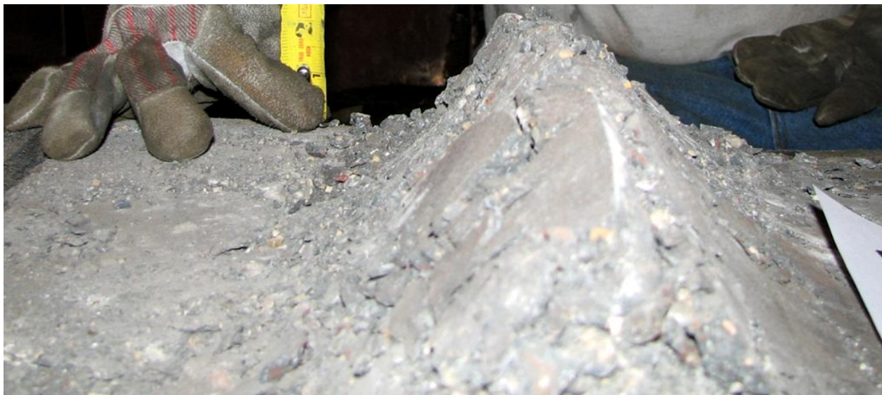
(c) Close up to the concrete deformed shape inside the steel local buckling
