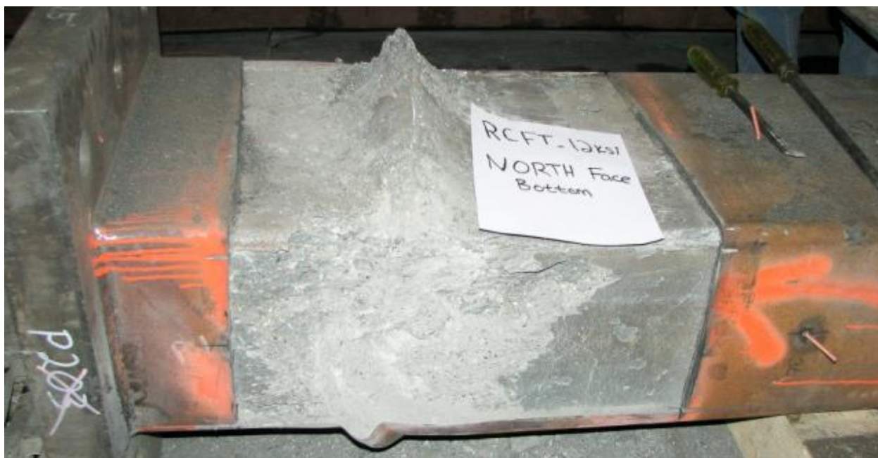
(d) Condition of the concrete in the external surface
