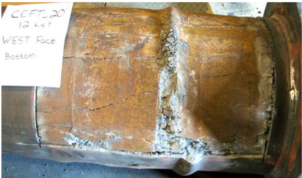
(b) Local buckling deformation spread by the concrete
