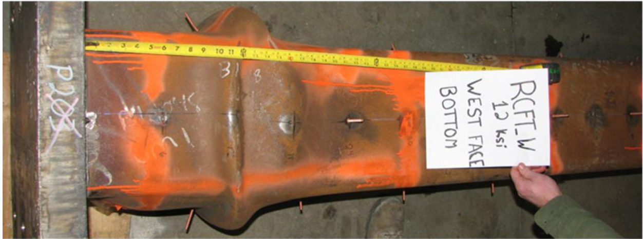
(a) Local buckling deformation in steel
