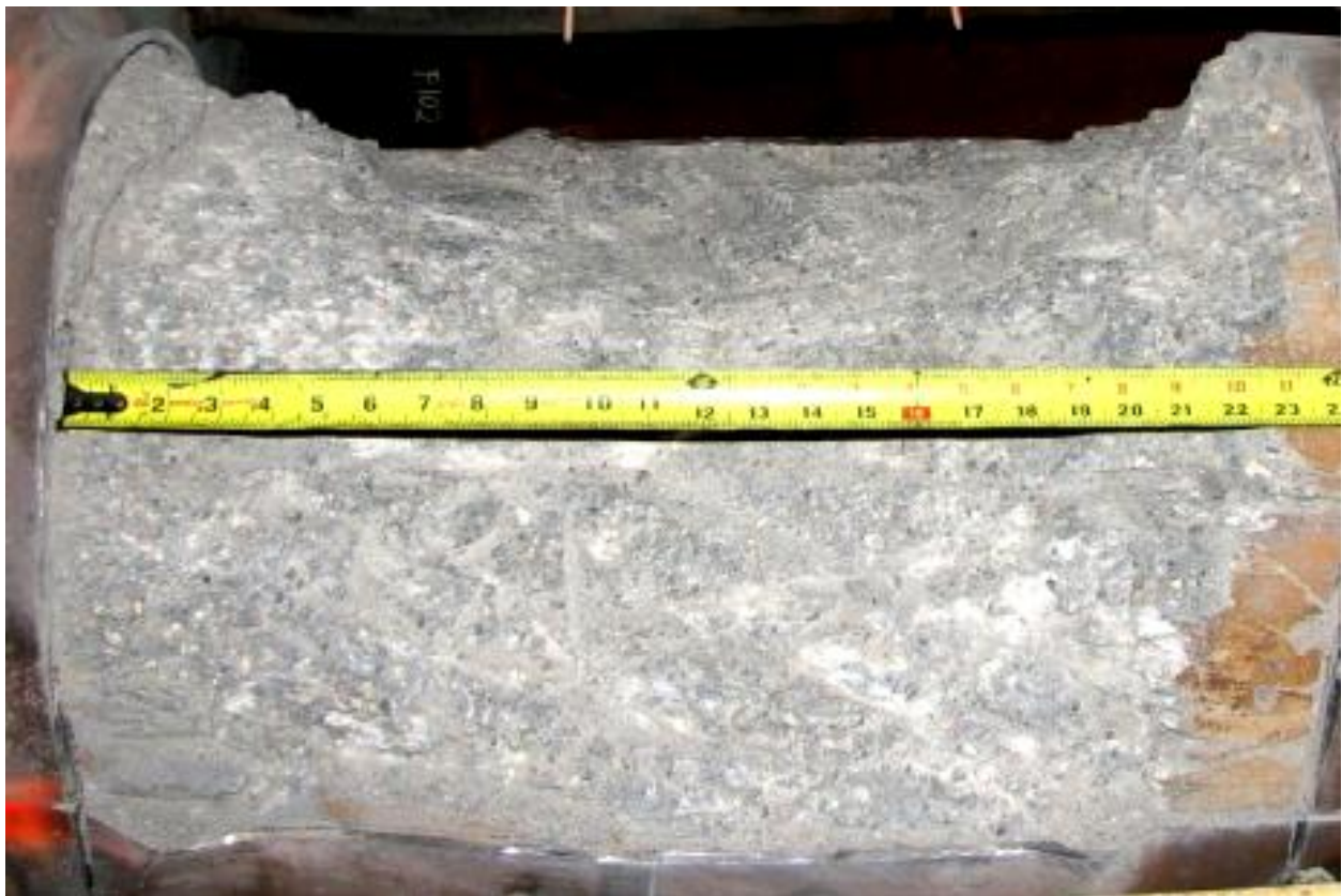
(d) Condition of the concrete in the interior core
