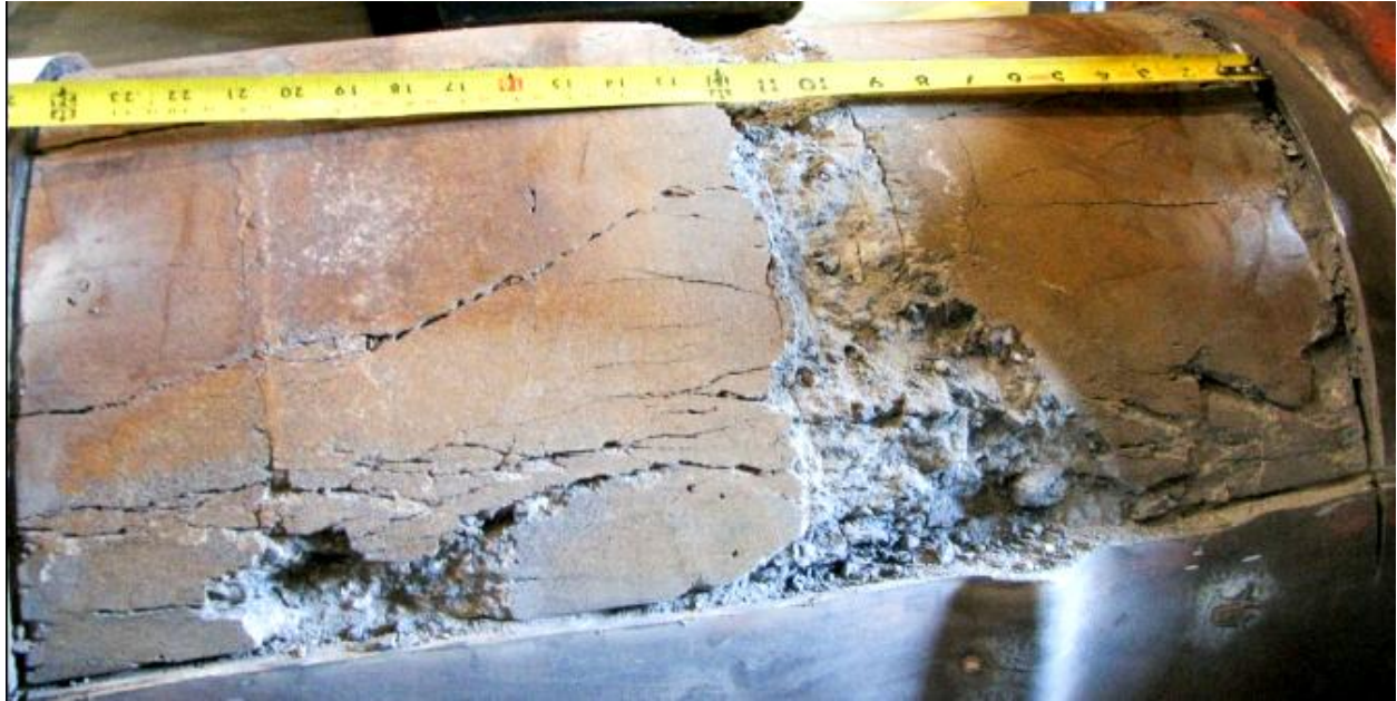
(c) Condition of the concrete in the external surface
