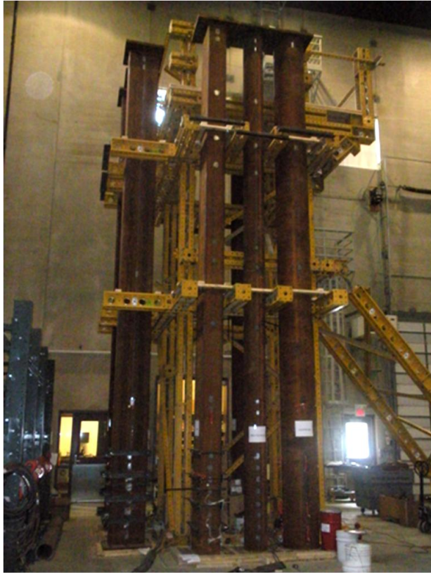
(a) Specimens stored ready for casting
