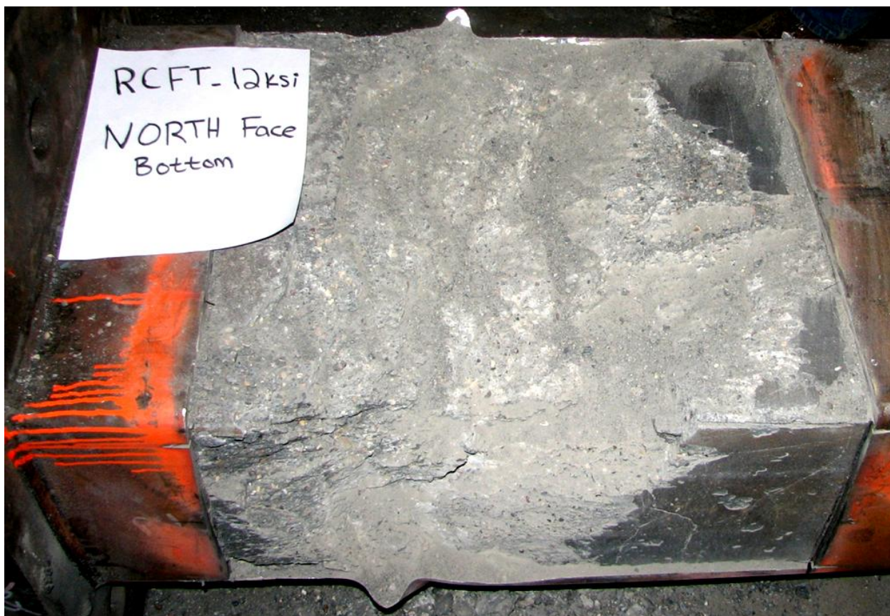
(e) Condition of the concrete in the interior core
