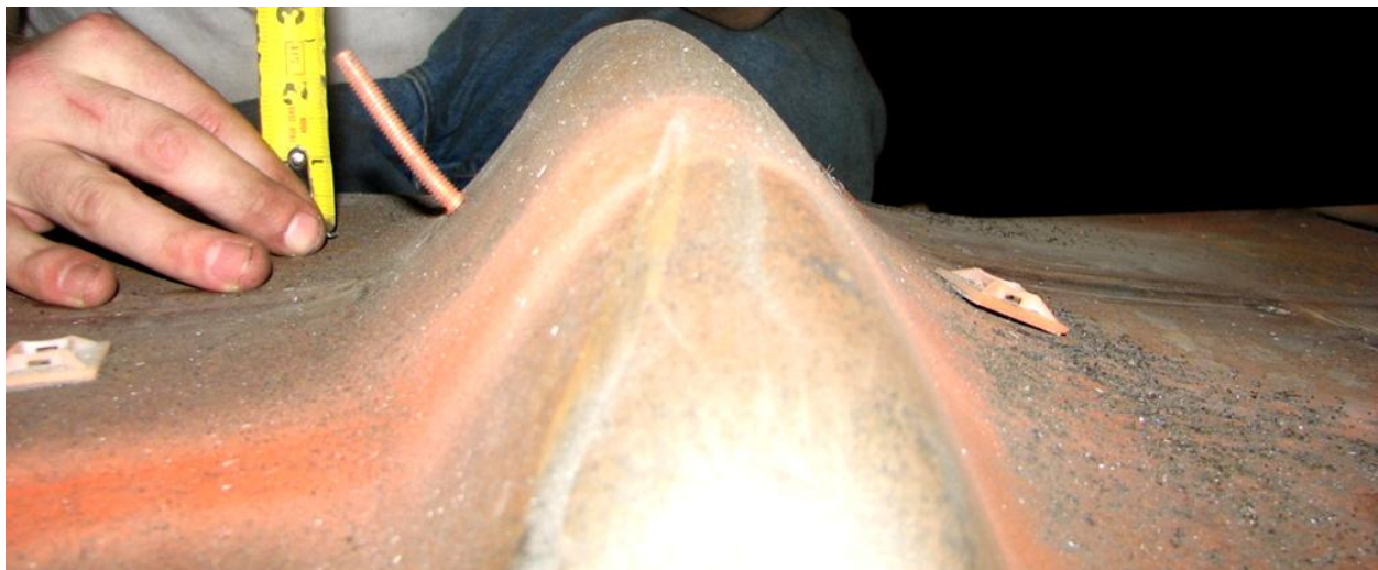
(b) Close up to the local buckling in steel
