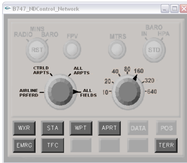
Figure 2.3: A modified Navigation Display Control Panel (NDCP) provides the major input interface to the APA, allowing the pilots to change the APA's configuration while monitoring the effects on the Navigation Display (ND), compare Fig. 2.2. A focus of the study is the effect of presence of the dial in the left, i.e. the newly introduced dial selecting the type of landing sites the pilot wants the APA to consider as alternates.
