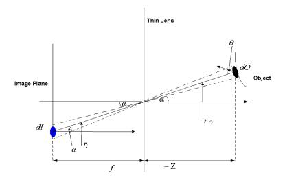
Figure C.1: Imaging geometry using a thin lens
