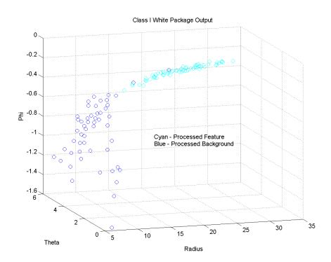
Figure 5.27: Scatter plots for Class I ouputs for defective seal in a white tray
