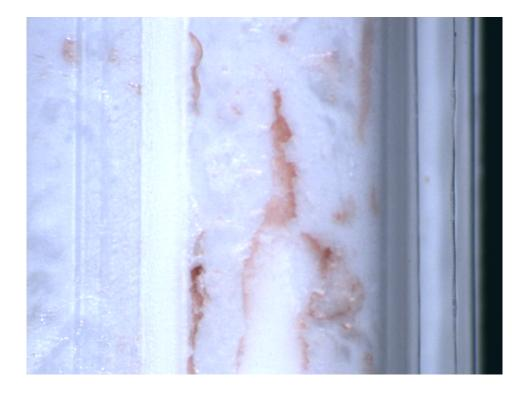
Figure 5.26: Package seal with contamination
