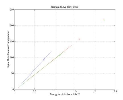
Figure D.3: Transformation Curves for the Sony 9000 Camera
