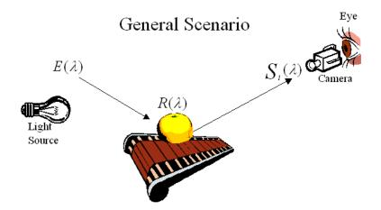
Figure 3.2: Common configuration for industrial imaging
