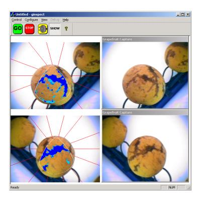
Figure 5.25: Sample input and output images for detecting scar on the surface of a grapefruit
