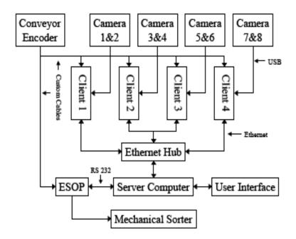
Figure 5.20: Block diagram of the grapefruit inspection cell illustrating its components
