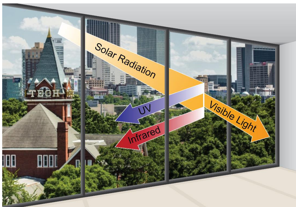
Figure 1.22 Heat Mirror Schematic for Passive Cooling DBRs can be designed to reflected near-IR radiation from the sun as well as UV-irradiation while maintaining visible transparency, thus reducing energy costs to cool via air-conditioning.
