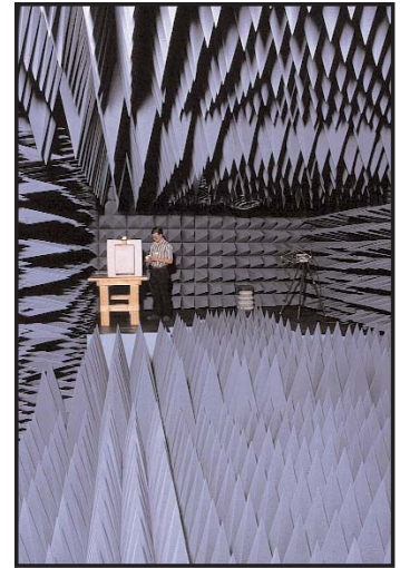
The anechoic chamber is multi-functional in design and configurable for many types of tests.
