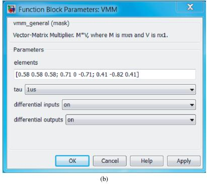
Figure 55: (a) Simulink block level design for a VMM system, including supporting blocks. The Sim2Spice tool is used to compile this block diagram down to object code ready to be programmed on the FPAA. (b) The Sim2Spice parameters for the VMM block. Rather than overwhelm the user with circuit specifics, the functionality has been abstracted for high-level system design.
