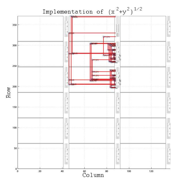
Figure 23: Visualization GUI for interfacing with the MITE FPAA. The GUI output is shown for a vector magnitude circuit.
