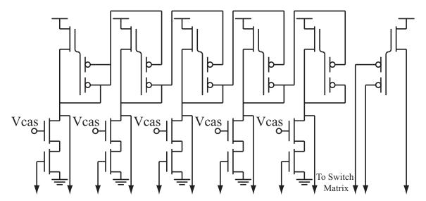
Figure 20: Basic MITE computation element of the MITE FPAA. The computation element consists of 5 input MITEs in a translinear loop configuration and 1 output MITE. The gates of the output MITE are sent into the switch matrix where they are connected to any of the input MITE gate voltages.
