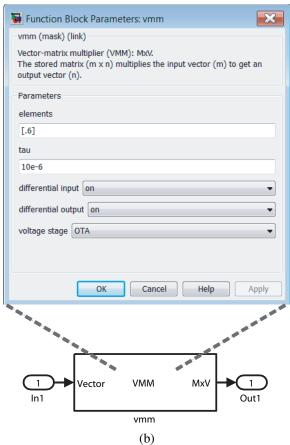
Figure 78: Design of the VMM Simulink block. (a) The conceptual-level diagram of the VMM shows that the output channels are sums of products of the input channels. The circuit implementation is very compact with FG elements performing the weights. (b) The input parameters for the VMM block, showing options for matrix elements, time constant, differential signals, and voltage structure. The final design is packaged into a single Simulink block.
