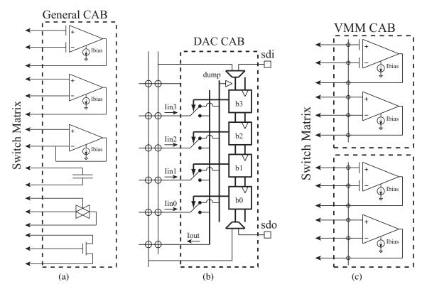
Figure 33: Structure of the RASP 2.9v CABs. (a) The General CAB consists of common analog elements: OTAs, MOSFETs, capacitors, and transmission-gates. (b) The DAC CAB contains an 8-bit register that toggles a bank of switches, allowing for multiple DAC topologies to be compiled. (c) The VMM CAB contains both regular and floating-gate-input OTAs, which are commonly used as the front end to the VMM: the FG-OTA for V/I conversion, and the OTA for the active feedback of the sense transistor.
