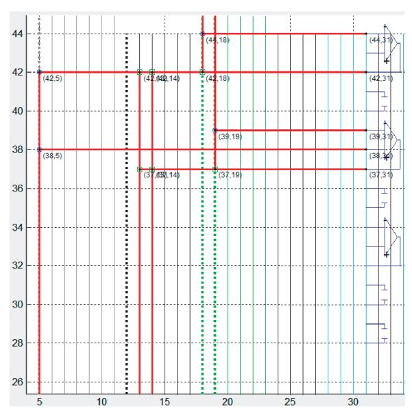
Figure 56: VMM visualization with the RAT tool. This tool allows the user to view and modify the switches that will be programmed on the FPAA.
