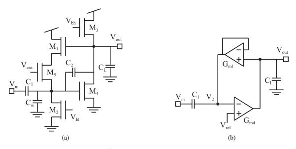
Figure 80: Schematics of the C<sup>4</sup> bandpass filter. (a) The schematic can be implemented either with transistors or (b) OTAs.
