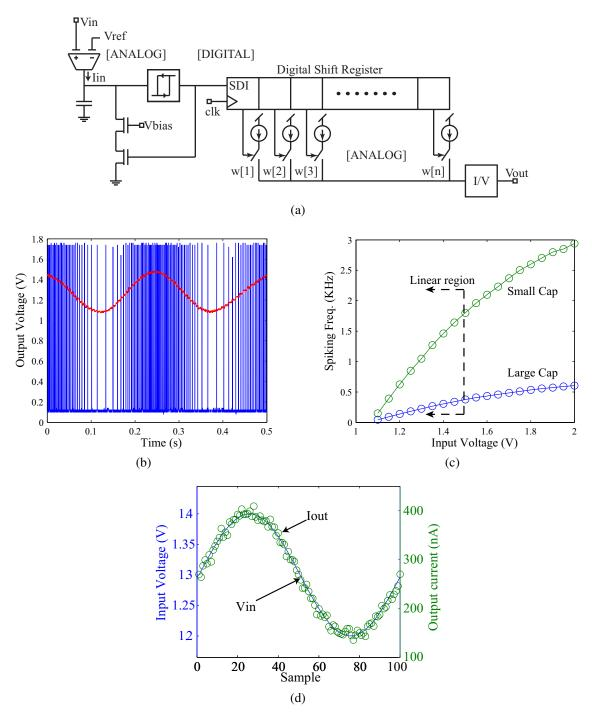
Figure 43: (a) Architecture for the mixed-signal FIR filter. (b) The integrate-and-fire spike generator produces digital pulses with a frequency based of the input current. (c) The integrating capacitor size can easily be reconfigured to tune the spiking frequency range. (d) The output of the mixed-signal system. The initial results show the output current correctly reconstructing a slow-moving input analog signal.
