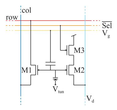
Figure 8: Indirect floating-gate switch cell.
