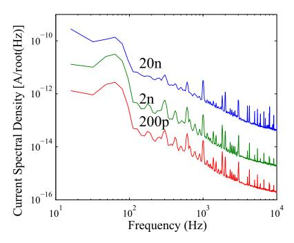
Figure 51: Current spectral density of the VMM noise. The lower bias current produces less current noise.
