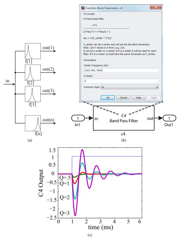
Figure 79: The  $C^4$  band-pass filter system. (a) The system implementation and (b) the Simulink block. (c) The Simulink step response for  $C^4$  filter vectorized with 4 outputs. Each tap is tuned for a center frequency of 1 kHz and a Q vector of [.5, 1, 2, 3].
