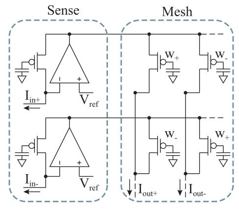
Figure 47: Schematic of the analog VMM circuit. The input floating-gate stage produces a log-compressed voltage representation of the input current. This voltage is broadcast to the source of each FG element in that row. These FGs produce an output current that is a scalar multiple of the input current, which are then summed along a column by KCL.
