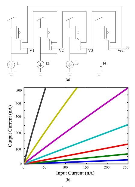
Figure 16: MITE implementation of a  $2^{nd}$ -order translinear loop. (a) Schematic of a  $2^{nd}$ -order translinear loop. (b) Simulation results of the translinear loop. The multiplication coefficients were chosen to be  $\frac{1}{10}$ ,  $\frac{1}{4}$ ,  $\frac{1}{2}$ , 1, 2, 4, and 10.
