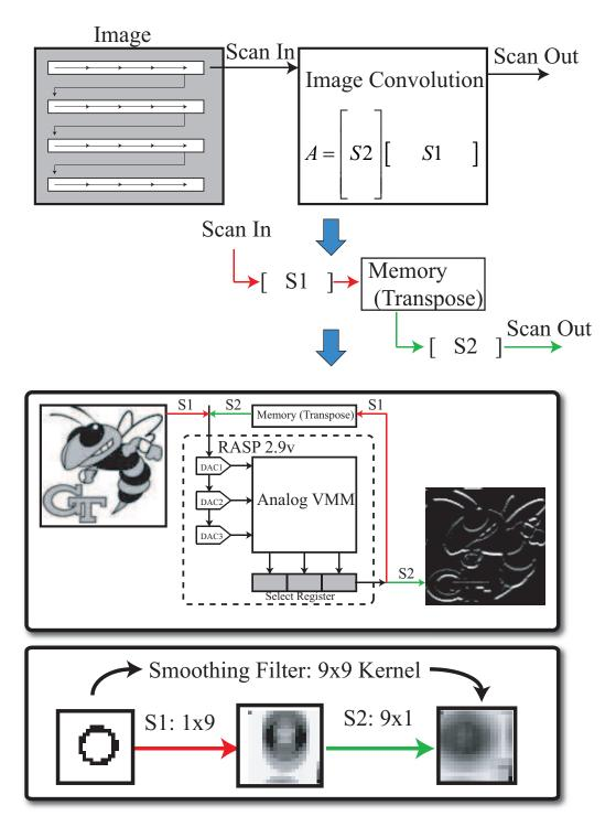
Figure 41: Application of the VMM in an image processing system. The image processor performs separable transforms scanning in the image and convolving by S1 and S2 in two passes. The kernels chosen for this test are a  $3\times3$  Sobel edge detector and a  $9\times9$  smoothing filter. The system schematic of the image processor front end shows the on-chip DAC components providing the signals to the VMM.
