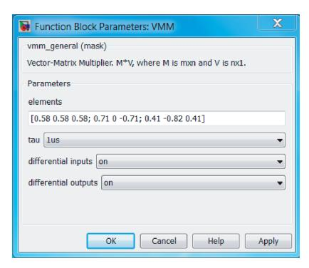
Figure 62: The block parameter window for the VMM provides a brief statement about the usage of the block, and asks the user to specify several needed parameters: the matrix elements, the desired time constant, and whether the inputs and outputs are to be single-ended or differential.
