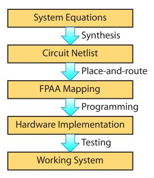
Figure 14: Design flow using a translinear FPAA. Using translinear circuits allows the user to enter a set of equations, which is then netlisted using existing synthesis procedures. The circuit is then place-and-routed, and the system is programmed onto the FPAA.
