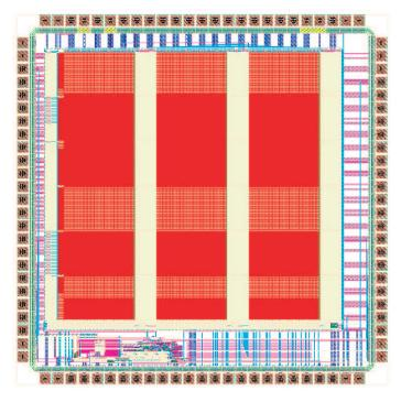
Figure 19: Layout of the MITE FPAA. The FPAA was fabricated in a 350 nm standard CMOS process on a 3 mm  $\times$  3 mm die.
