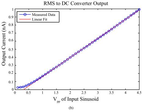
Figure 30: RMS-to-DC converter. (a) The RMS-to-DC converter as it is complied into a single MITE CAB. The three computational stages are: square, filter, and square-root. These three functions can each be performed by a single MCE. (b) The output characteristic of the RMS-to-DC converter. The amplitude of the input sinusoid was swept from 0.1 - 4.5 V. The frequency of the input was held at 500 Hz.
