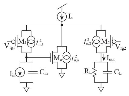
Figure 50: Schematic of the  $1 \times 1$  VMM noise model.
