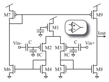
Figure 34: Schematic of the operational transconductance amplifier (OTA). Both the regular and FG-input OTAs use a 9-transistor structure. The bias current is set with an FG pFET and can be programmed from 100 nA to 30  $\mu$ A. The FG-input has an attenuation factor of 1:9 on the input stage for wider input linear range (with lower gain). The FG input elements can also be programmed to remove any input offset.
