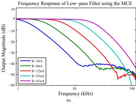
Figure 28: Log-domain filter of the MITE FPAA. (a) The MITE FPAA uses a standard first-order MITE log-domain filter in order to implement dynamic functions. (b) The transfer function of a first-order low-pass filter for various bias currents is shown. The bias currents used were logarithmically spaced between 3 nA and 41 nA. Note that the highest achievable corner frequency is 200 kHz.
