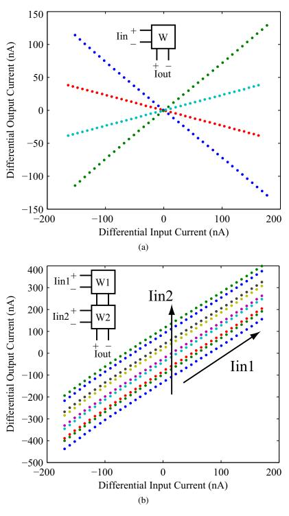
Figure 48: VMM current mode sweeps. (a) A  $1 \times 1$  VMM; the inputs are swept differentially, to create differential outputs. The multiplier coefficients for this sweep are  $\pm 1$  and  $\pm 0.5$ . (b) A  $2 \times 1$  VMM; this sweep demonstrates the summation of the two inputs. One input is swept differentially for each constant value of the second input, resulting in vertical offsets.
