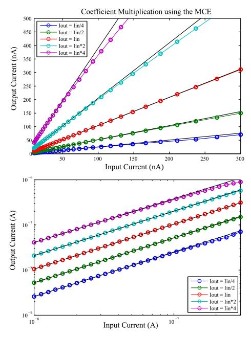
Figure 24: Results of a coefficient multiplication circuit implemented with the MITE FPAA. The results are shown in a linear plot (top) and a log plot (bottom) to show both the accuracy and the dynamic range of the computation.
