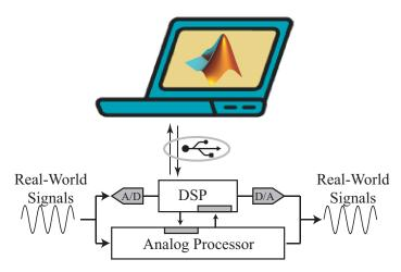
Figure 2: The analog processor embedded with a digital processor provides a power efficient platform. The incoming signal can be processed by the FPAA, the DSP, or by a combination of both. A custom Matlab toolbox is used to program and control the mixed-mode processor.
