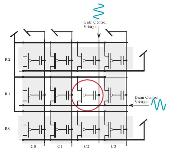
Figure 7: Floating-gate array isolation.
