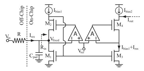
Figure 21: Voltage-to-current converter used in the MITE FPAA. The amplifier on the input side provides an extremely low input resistance allowing for high speed and good accuracy. The amplifier on the output side reduces mismatch between the input and output currents by matching the drain voltages of the mirror transistors. The bias currents are provided by floating gates.
