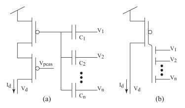
Figure 15: Subthreshold pFET realization of a MITE. (a) Components used to realize a MITE in a standard CMOS process. (b) Symbol used to represent a MITE.
