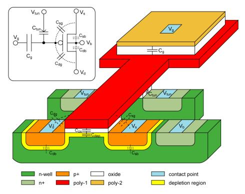
Figure 4: Floating-gate transistor technology. The distinguishing feature is that the polysilicon gate is completely insulated by oxide. The input gate voltage is coupled in through a poly capacitor and the tunneling voltage through a MOS capacitor.
