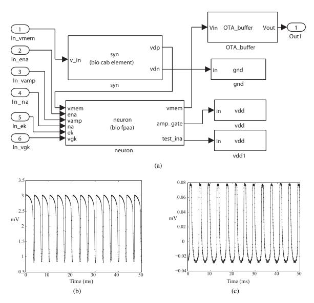
Figure 68: (a) Simulink model of the spiking neuron system. (b) Simulink simulation of the spiking. (c) Spiking as compiled on FPAA. The complete example is a spiking Hodgkin-Huxley neuron, input block, and output buffer.
