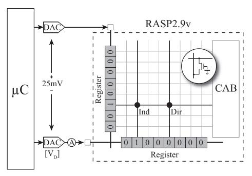
Figure 37: The volatile switches can be leveraged to dynamically select which FG switch to read from in a measurement test.
