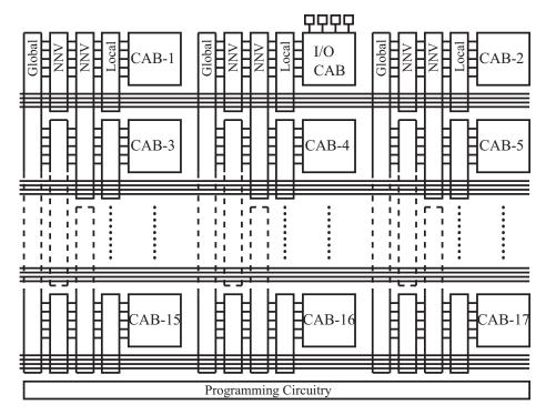
Figure 18: Architecture of the MITE FPAA. The FPAA consists of 17 MITE CABs and a single IO CAB. The vertical routing between CABs is organized into local, nearest-neighbor vertical (NNV), and global. The horizontal routing is only global.
