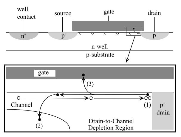
Figure 6: Channel diagram of hot-electron injection.
