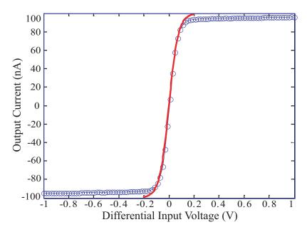
Figure 63: OTA tanh model and FPAA data. The smooth curve is a tanh function, which can be used to model the OTA. The bubbles are data taken from the FPAA hardware.
