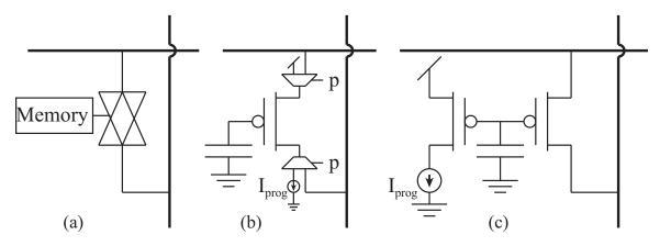
Figure 9: The three types of FPAA switches. (a) The traditional switch with a separate memory element. (b) Floating gate switch elements store their programmed value, allowing for a very area efficient design. (c) Indirect programming reduces the switches in the signal path.
