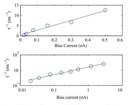
Figure 49: Linear and log plot of the inverse VMM time constant. The inverse of the time constant increases linearly with an increase in bias current. The slope of the linear plot corresponds to an input capacitance of 1.62 pF. The slope of the log plot is 0.99.
