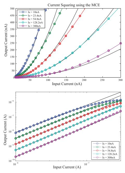
Figure 25: Results of a squaring circuit implemented with the MITE FPAA. The results are shown in a linear plot (top) and a log plot (bottom) to show both the accuracy and the dynamic range of the computation. Note that the inaccuracy at high output currents is due to devices leaving subthreshold operation.
