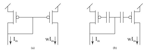
Figure 45: Two implementations of a current-scaling mirror. (a) Traditional current mirrors scale current based on the fabricated aspect ratio. Although this can perform a fixed coefficient multiplication, it is not reconfigurable post fabrication. (b) By introducing floating gates into the current mirror, we can set the scaling weight based on the amount of charge on the floating node.
