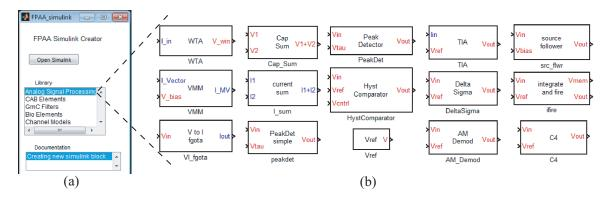
Figure 61: The Simulink component library. (a) The Matlab GUI presents the user with all of the available component libraries. (b) Expansion of the Analog Signal Processing library. Blocks are continuously being added to the library as other users share their functional blocks.
