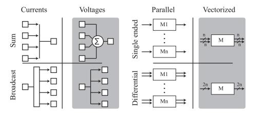
Figure 73: The system abstraction first involves defining our signal protocol. Custom analog design is free to take advantage of current-mode signals, which are easily summed. However, we constrain the analog processing tool to use only voltage-mode between blocks because it is more similar to digital design and fits into the Simulink framework. Vectorized signals are also important because they take advantage of the analog processor's parallel processing capabilities.
