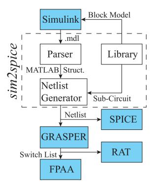
Figure 59: The complete tool set is comprised of Sim2Spice, which converts a Simulink design to a SPICE netlist, and GRASPER, which converts a SPICE netlist to a set of switches for programming on the FPAA.
