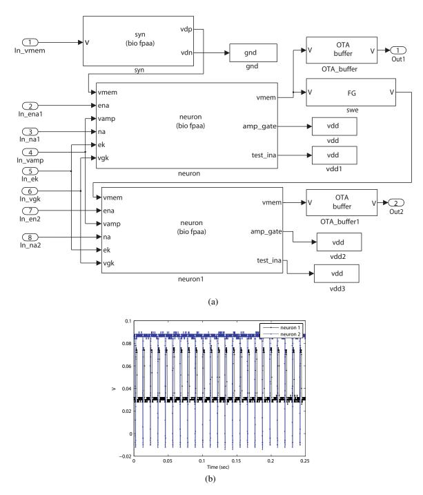
Figure 69: (a) Simulink model of two neurons and a synapse. (b) Spiking activity of the two neurons. The pair of neurons demonstrates synchronized spiking due to the coupling through the synapse circuit element.
