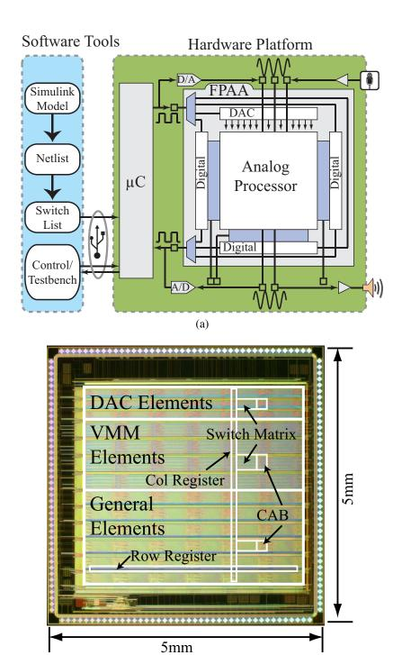
Figure 32: Architecture and layout of the RASP 2.9v FPAA. (a) The system-level diagram shows the analog core and surrounding digital control and interfacing. The analog processor communicates directly with the microcontroller via an SPI interface. A complete software tool chain is available for analog synthesis in Simulink and connects to the hardware platform with USB. (b) The RASP 2.9v IC was fabricated in 350 nm CMOS and consumes 25 mm<sup>2</sup> of area.
