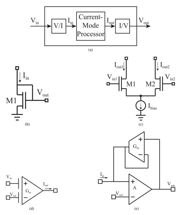
Figure 77: (a) Embedding V/I and I/V stages into the analog blocks allows the system interconnects to be voltage-mode. There are multiple implementations of the V/I and I/V stages, such as the (b) diode-connected FET, (c) differential pair, (d) wide-range OTA, and (e) transimpedance amplifier.
