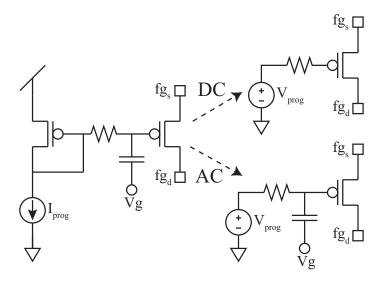
Figure 65: Floating gate SPICE model. This model is needed because SPICE cannot implement a true floating-gate transistor. The model closely resembles the indirect programming structure used on the FPAA. Under DC circumstances, the floating gate model resembles the upper equivalent circuit: a normal pFET with a fixed potential on the gate. Under AC conditions, the circuit will act as the lower circuit; the gate programming voltage will be coupled onto the floating node.
