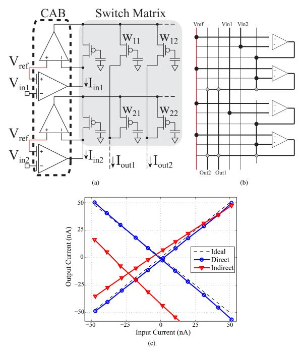
Figure 40: (a) The schematic and (b) FPAA implementation of a  $2 \times 2$  VMM. (c) Data from a differential  $1 \times 1$  VMM. The directly programmed devices in the VMM cab allow accurate multiplication (to 4.5 bits) on the first programming pass, eliminating the calibration needed in earlier RASP designs for linear processing. The one-pass programmed indirect-switch VMM shows significant gain and offset error. Calibration can be used, however, to increase the accuracy to 6 bits.
