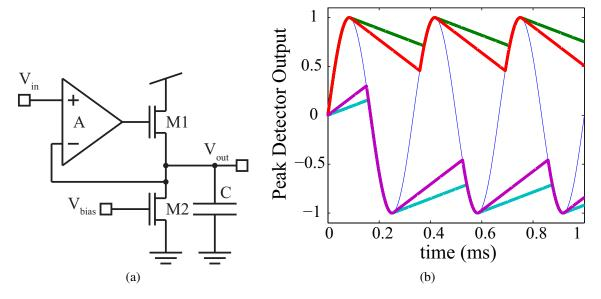
Figure 81: The Peak Detector. (a) Schematic and (b) Simulink simulation. The output shows the block vectorized for four outputs with a common sine input. Of the four signals, two are MAX followers and two are MIN followers, each shows with decay rates of 1e3 and 2e3.
