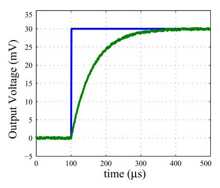
Figure 76: Simulink simulation of the first-order filter with noise enabled.
