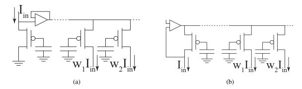
Figure 46: Two implementations of a source-coupled floating-gate current mirror. (a) Buffered input stage. The source voltage is buffered with an OTA follower. (b) Log-amp input stage. A logarithmic amplifier is used to compress the input current.
