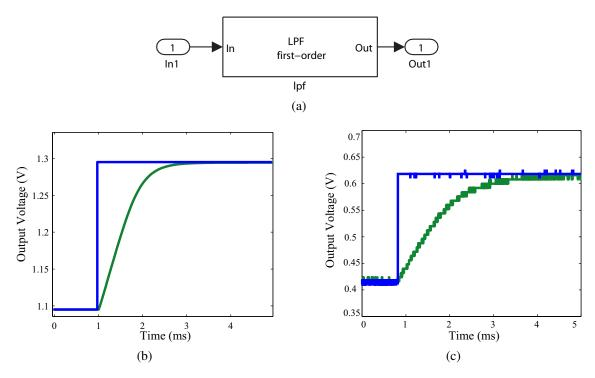
Figure 67: (a) Simulink model of the low-pass filter. (b) Step response in SPICE simulation. (c) Step response on FPAA.
