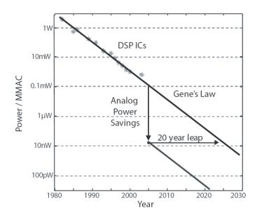
Figure 1: Gene's law shows the power efficiency trend for digital signal processors. Analog signal processing poses a 20-year leap in efficiency.
