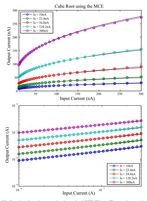
Figure 27: Results of a cube root circuit on the MITE FPAA. The results are shown in a linear plot (top) and a log plot (bottom) to show both the accuracy and the dynamic range of the computation.
