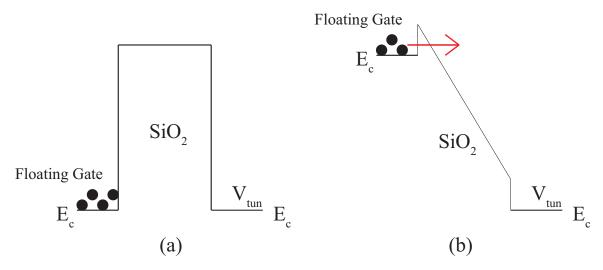
Figure 5: Band diagram of electron tunneling.
