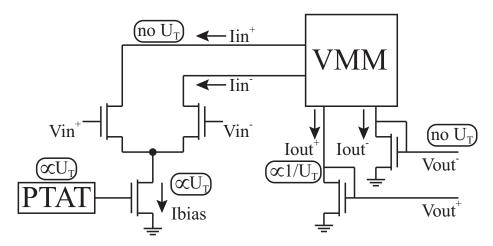
Figure 53: Schematic of the VMM temperature compensation circuitry. The diode-connected nFETs at the output cancel the temperature dependence of the multiplier weight. The input differential pair with PTAT current source will have no temperature dependence.
