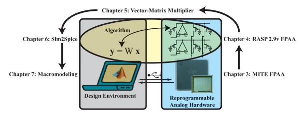
Figure 3: Diagram of the coordinated approach to FPAA design.
