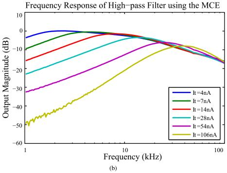
Figure 29: Log-domain high-pass filter. (a) The log-domain high-pass filter can easily be complied into a single MITE CAB. To implement the high-pass filter a low-pass version of the signal is subtracted from the original signal using the current mirror. (b) The transfer function of the filter for various bias currents is shown. The bias currents used were logarithmically spaced between 4 nA and 106 nA.
