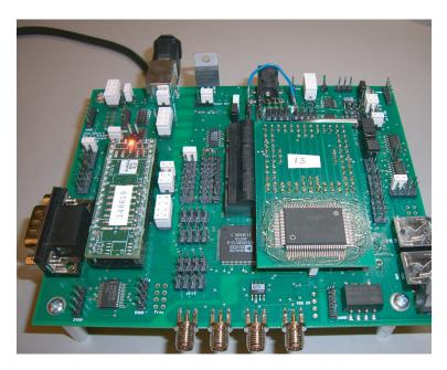
Figure 66: The Program & Evaluation board. This board communicates with MATLAB over a USB connection. The board contains a microcontroller for controlling the programming algorithms, a 40-channel DAC and a 4-channel ADC for creating and reading test signals, and all necessary power management circuitry.
