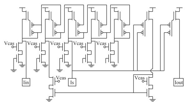
Figure 26: Circuit that implements a cube root on the MITE FPAA. A second output MITE, from the other MCE in the CAB, is used to gain access to the output current. In addition, a current mirror is used to feed back the output current to create the cube root.
