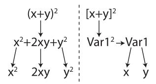
Figure 22: A representation of equation parsing for the MITE FPAA. Equations are split at addition and subtraction signs to create units that will be implemented by MCEs. The user's expression is expanded first in order to create a simple parsing tree (left). However, the user can define sub-blocks by using brackets to replace an expression with an intermediate variable [right].
