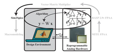
Figure 58: The coordinated approach to FPAA design: Sim2Spice.
