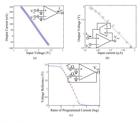
Figure 57: Supporting blocks for the VMM. (a) Input stage V-to-I converter, (b) output stage I-to-V converter, and (c) programmable voltage reference. The design for these blocks was highly motivated by the available components in the FPAA, in this case OTAs.
