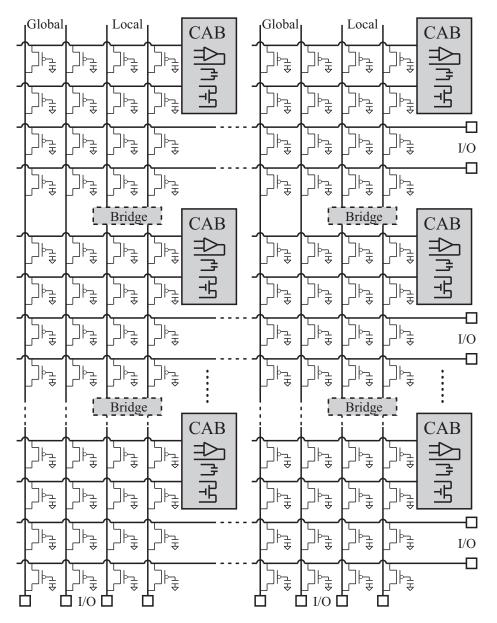
Figure 10: The architecture of the RASP 2.8 FPAA. The routing is a full crossbar switch matrix with floating-gate switches. The FG switches can be used for computation, such as for vector-matrix multiplier (VMM) weights.
