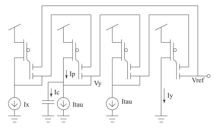
Figure 17: MITE implementation of a 1<sup>st</sup>-order low-pass log-domain filter. The  $I_{\tau}$  bias current connected to the capacitor is used to set the corner frequency of the filter. The second bias current is set to  $I_{\tau}$  in order to maintain unity gain.
