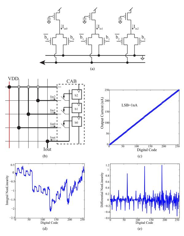
Figure 39: The on-chip compilable DAC. (a) The schematic and (b) FPAA implementation of the floating-gate current-source DAC. (c) The measured results from a compiled 8-bit current DAC shows an LSB of 0.98 nA. (d) The INL and (e) DNL plots from the 8-bit current DAC.
