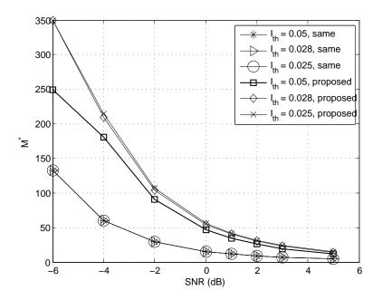
Figure 3.2. Optimum sensing block length for different  $\gamma$ .
