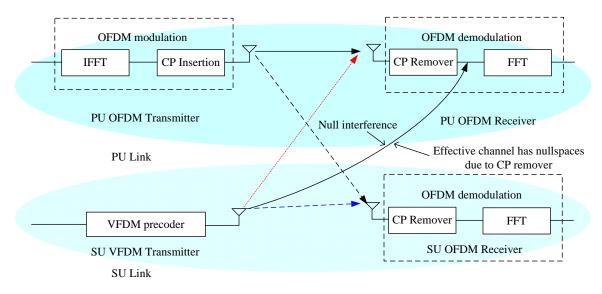
Figure 1.1. Basic concept of the VFDM.
