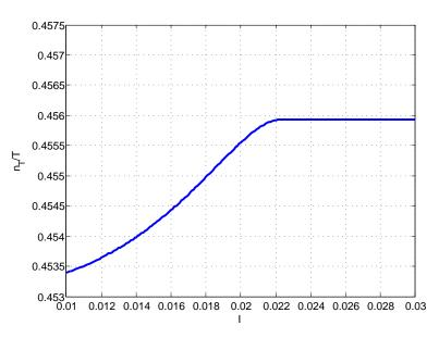
(a) Optimal throughput versus interference threshold, where  $\gamma = 0.04$  and  $P_d = 0.9$ .
