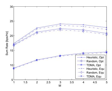
Figure 5.5. Sum rate of two cells for different number of SUs in each cell, M, with K = 64 and L = 16.
