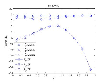
Figure 6.3. Optimized power solution for different relay locations.
