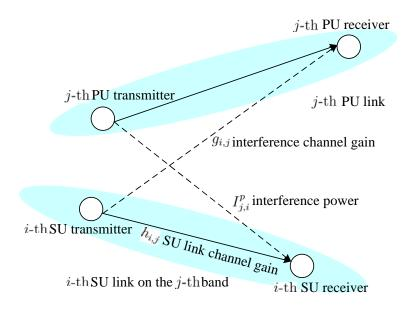
Figure 7.1. Spectrum underlay system model.
