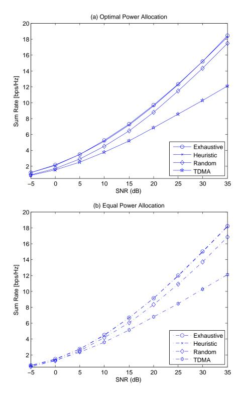
Figure 5.3. Sum rate of two cells for the partially-aligned transmission with K = 16, L = 2, M = 2 and  $M_t = M_r = 2$ .
