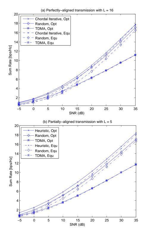
Figure 5.4. Sum rate of two cells for the perfectly- and partially-aligned transmission with K = 64, M = 2 and  $M_t = M_r = 2$ .
