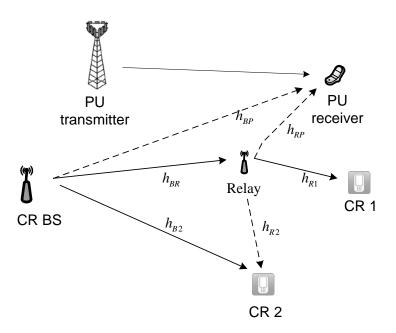
Figure 6.1. The structure of a CR network with direct and relay-aided transmissions.
