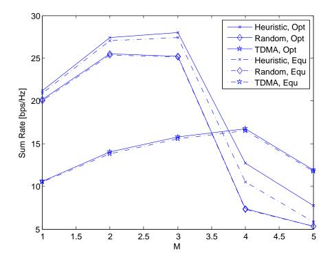
Figure 5.6. Sum rate of two cells for different number of SUs in each cell, M, with K = 64 and L = 5.
