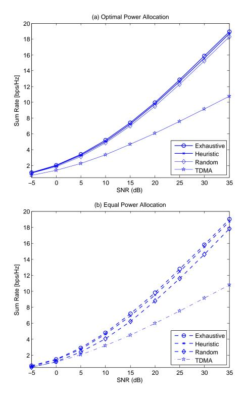
Figure 5.2. Sum rate of two cells for the perfectly-aligned transmission with K = 16, L = 4, M = 2 and  $M_t = M_r = 2$ .
