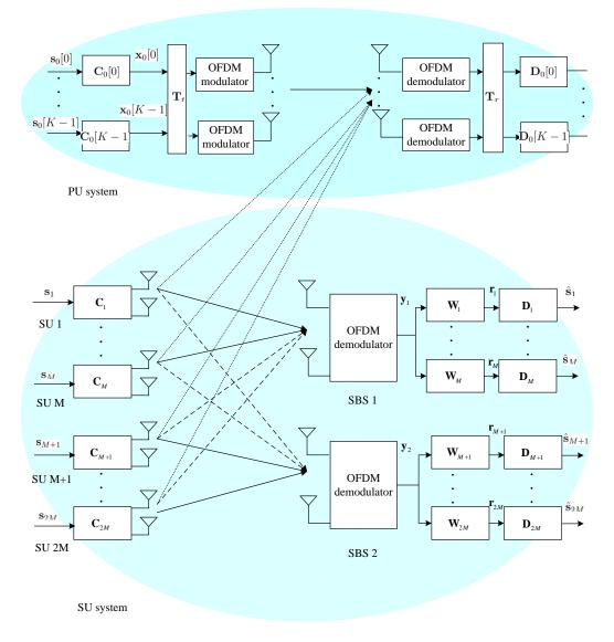
Figure 5.1. System model of a two-cell secondary network where solid lines and dashed lines denote the intended signals and interference signals, respectively.
