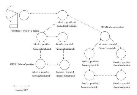
Figure 2: Graphical Illustration of a typical host file
