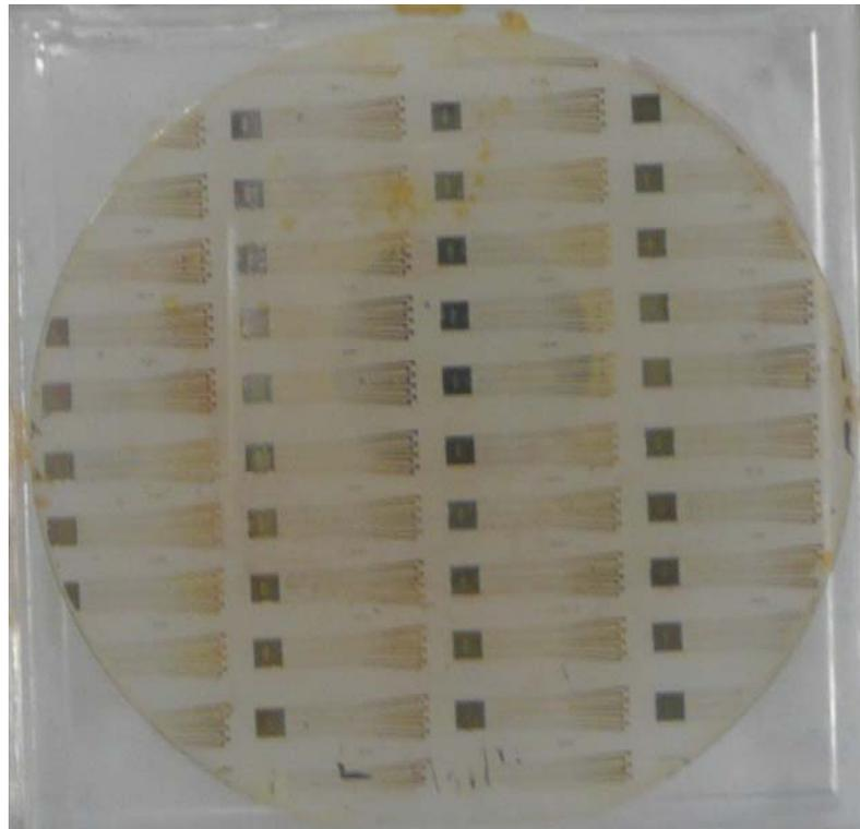
**Figure 31.** Photograph of a completed wafer. The devices are clearly visible. Since the photograph was taken prior to shipment for dicing, the yellowish color is due to the protective photoresist layer.
