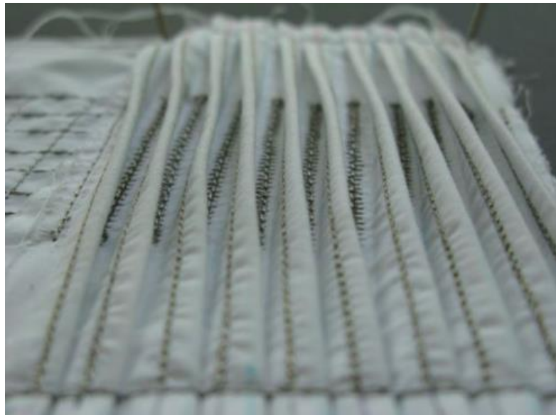
Figure 15 - Pleat: This knife-edge pleat is constructed with three electrodes. Depending on in which direction the pleat is crushed, different circuits are completed [32]
