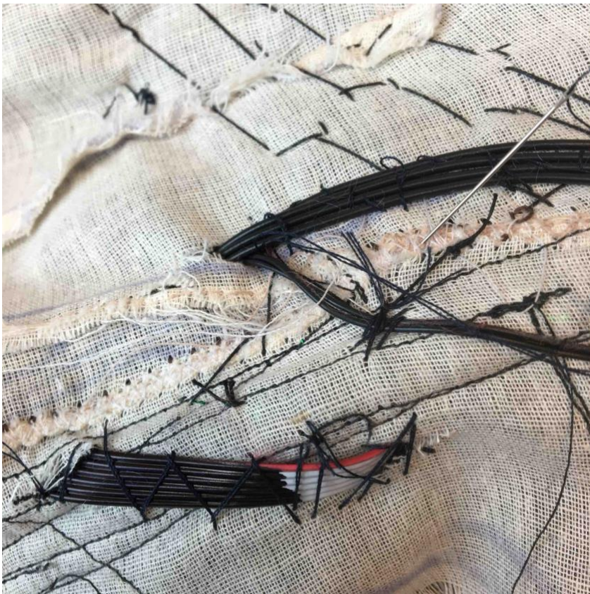
Figure 4 – With proper diagonal and vertical placement, wires like these (sometimes necessary in early prototypes) can act as structural support for the garment and the components they service.
