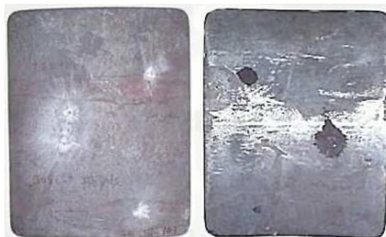
Figure 7.6 Steel armor plates for hard body armor
