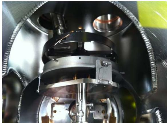
**Figure 2.** Block approaching STM sample acceptor
