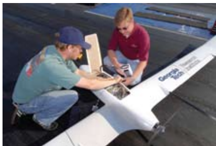
Thomas Bradley (left), a doctoral student in Mechanical Engineering, and Reid Thomas starting the fuel cell aircraft during a test flight at the Atlanta Dragway.
