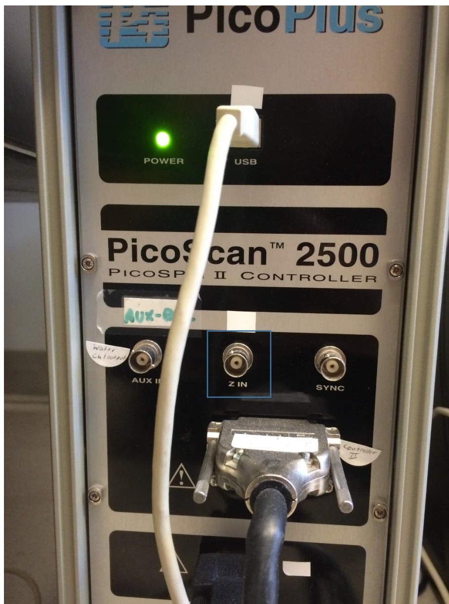
Figure 3.2.5: The front face of the PicoPlus AFM controller. The Aux portal indicated with blue box is the input of the small oscillation.
