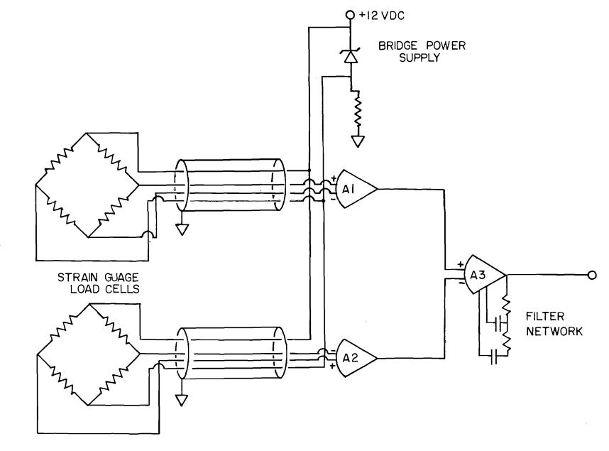
Fig. 4. Amplifier and Load Cell Circuitry for One Weigh Station
