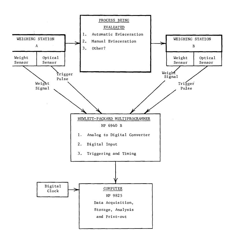
Fig. 2. Schematic of Data Acquisition System
