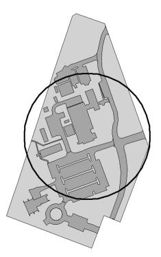
Figure 2 Facility map showing impervious surfaces (darker shaded areas) and equivalent impervious footprint (5.24 acres circle).
