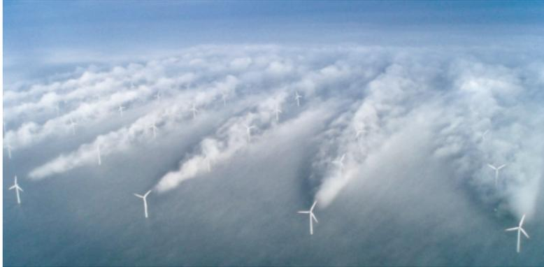
Figure 1: Aerial photograph of offshore wind farm wake interaction (Horns Rev, Denmark)
