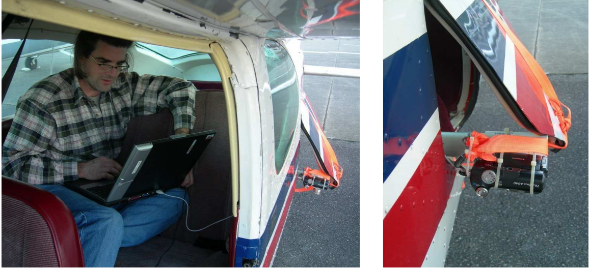
Figure 61: Our operation: a consumer camera zip-tied to a PVC pipe protruding from a hand-flown Cessna 177.
