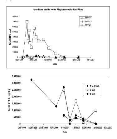
Figure 1. Change in concentration of COCs in groundwater wells (above) and soils (below).
