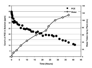
Figure 2. Results of bench scale treatability tests to confirm uptake of chlorinated solvents from groundwater by the trees used in Case Study #2.
