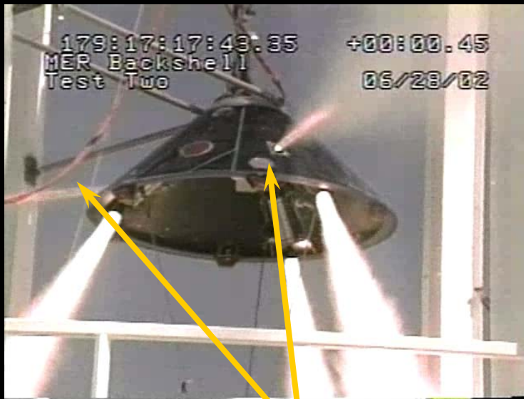
Two of 3 Transverse Impulse Rocket Subsystems (TIRS)
