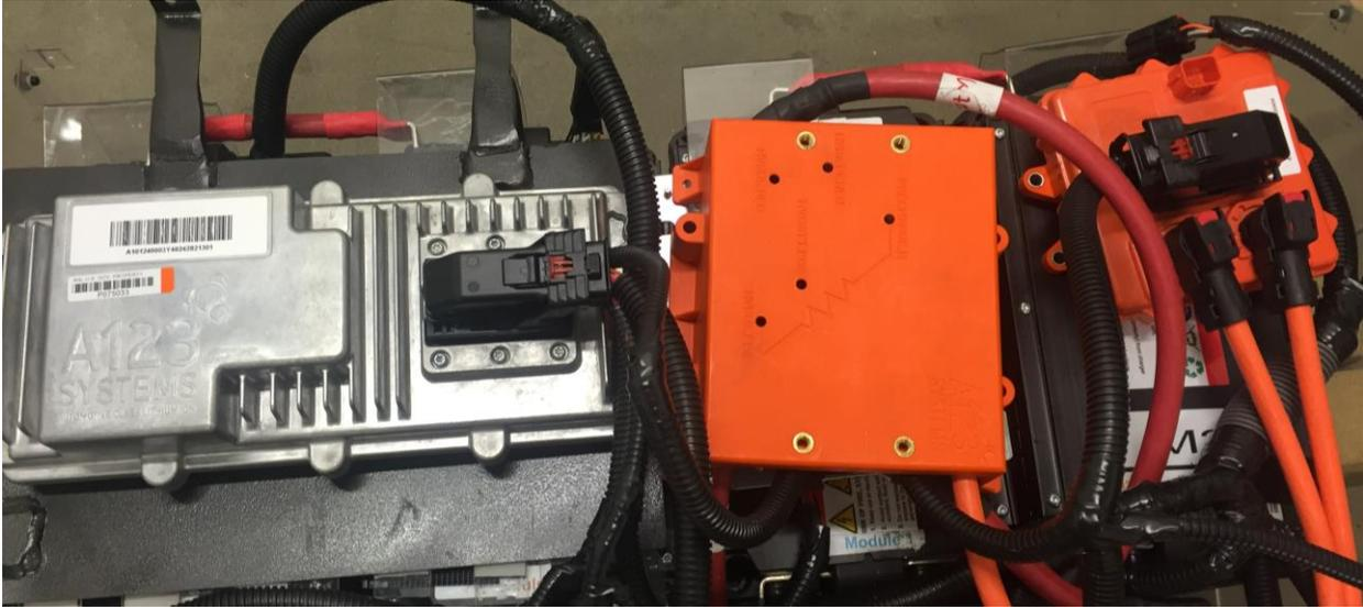
**Figure 17: BCM (grey), EDM (orange), and CSM (orange) from left to right**
