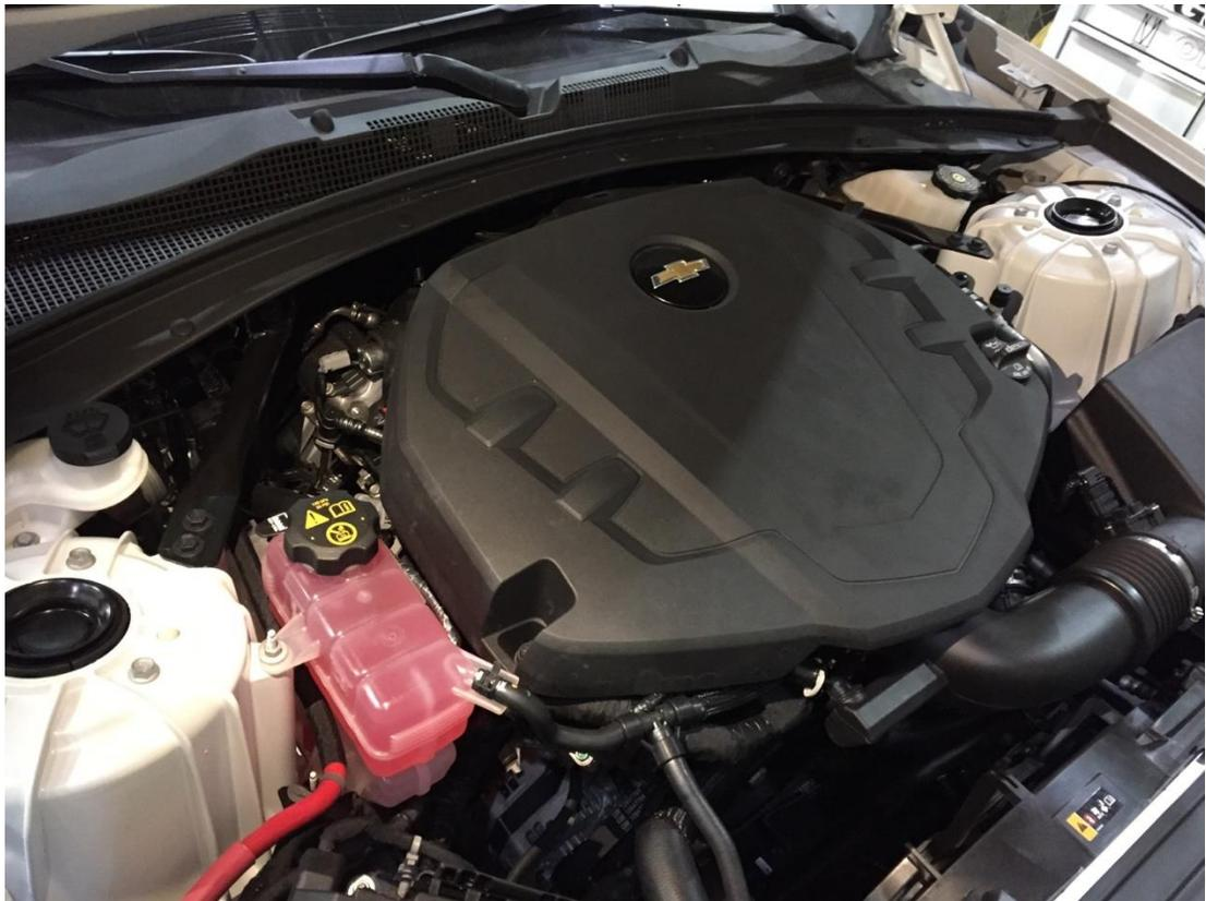
**Figure 4: Stock LGX engine, to be removed**
