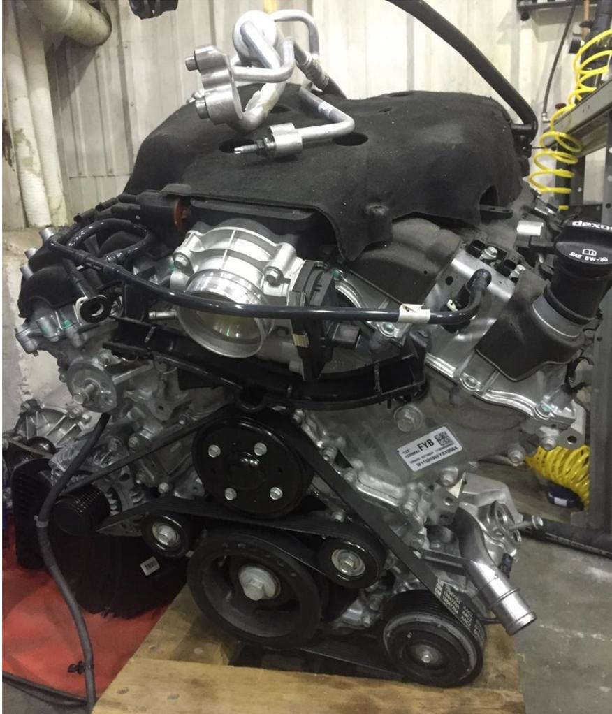
**Figure 57: Stock LGX Engine removed from Camaro**
