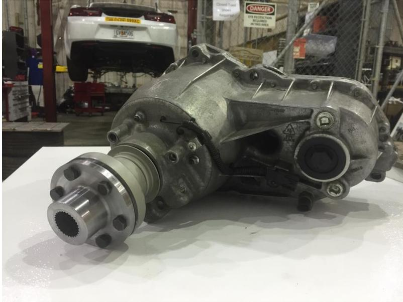
**Figure 7: Transfer Case, showing front driveshaft connection**
