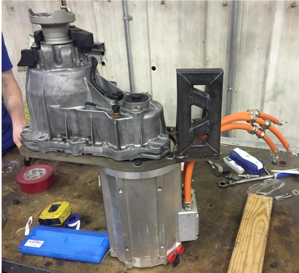
**Figure 65: Motor (bottom) plugged into Transfer Case (top) and attached with middle MTC mount**
