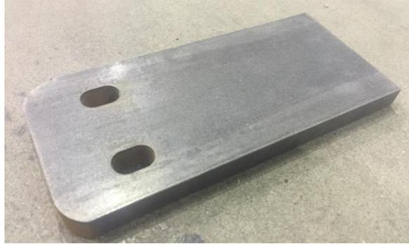
**Figure 21: Battery Pack Mounting Block**
