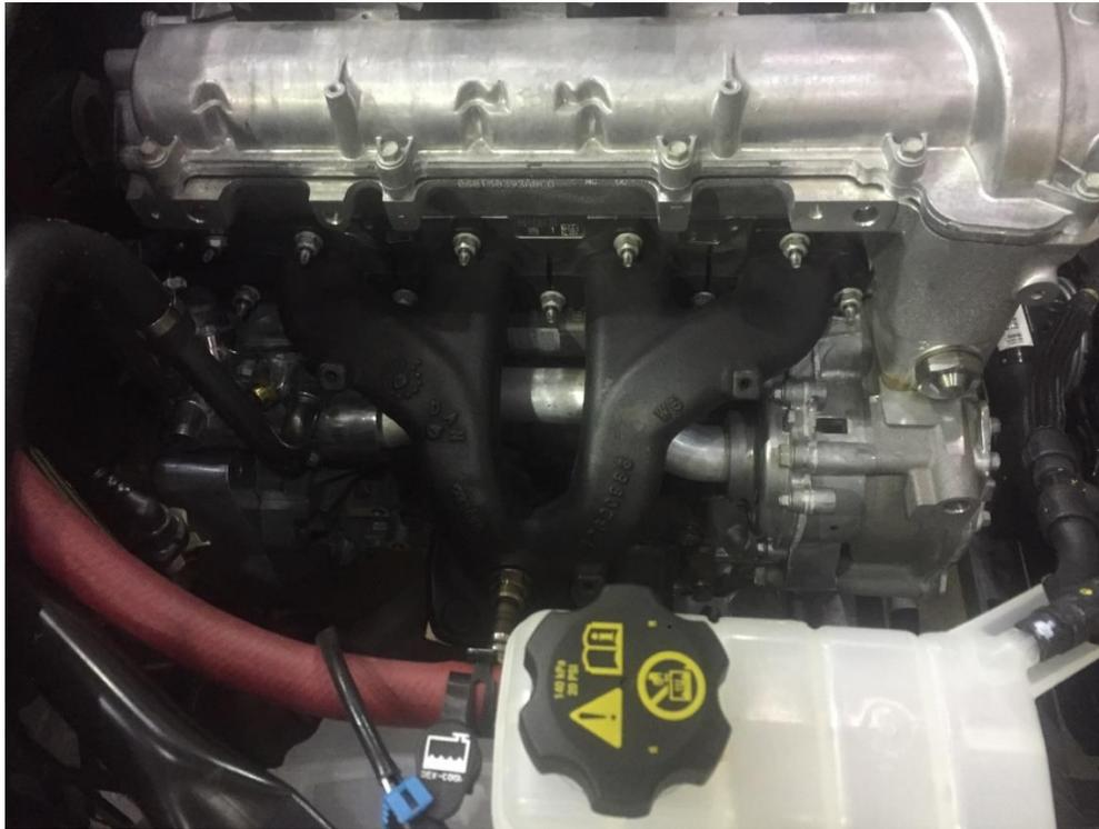
**Figure 61: Exhaust manifold and routing as installed**
