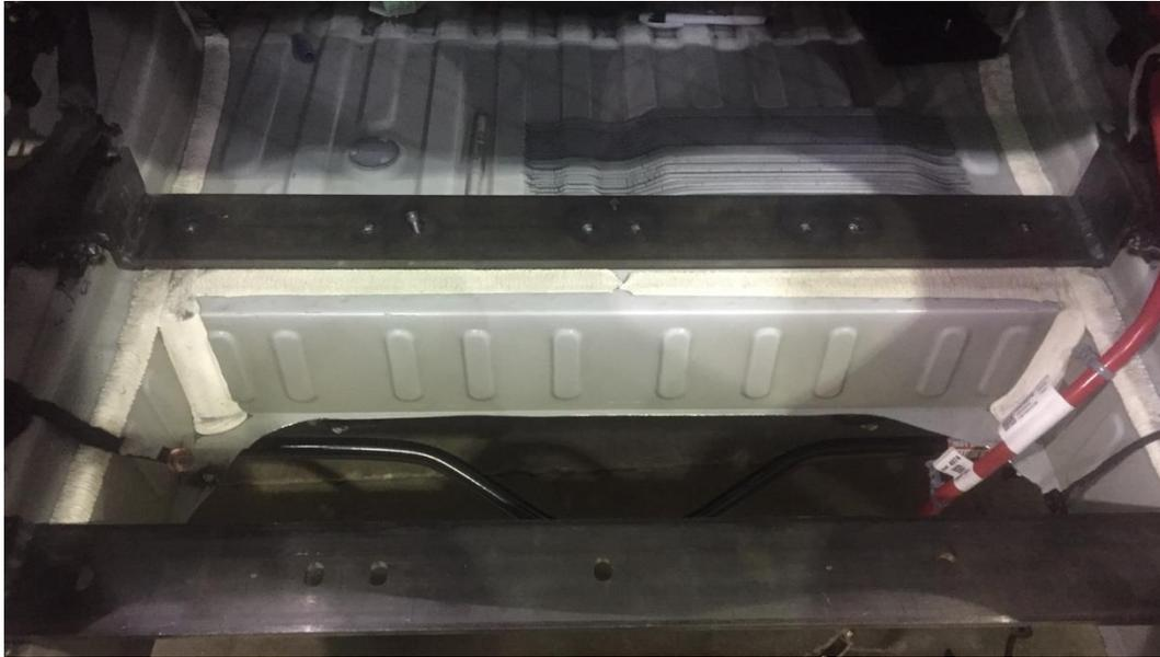
**Figure 20: Straps across trunk frame rails**
