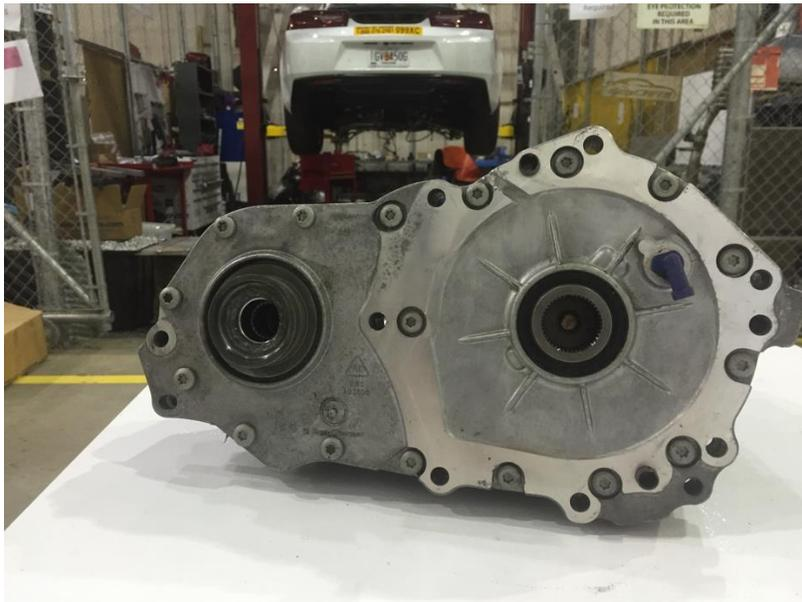
**Figure 8: Transfer Case, showing rear driveshaft and motor connections**
