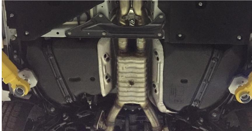
**Figure 5: Camaro stock underbody with saddle tank spanning exhaust routing**
