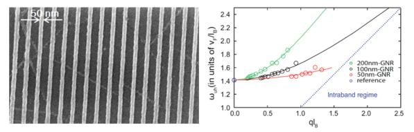
**Figure 1:** (Left panel) Scanning electron microscopy image of a 50nm-wide GNR array sample. (Right panel) Dispersion relation of the UHM,  $\omega_{uh}(ql_B)$ , in units of  $v_F/l_B$ , where  $\omega_{uh}$  is the UHM frequency, q is the in-plane wave vector,  $v_F$  is the Fermi velocity, and  $l_B$  is the magnetic length.
