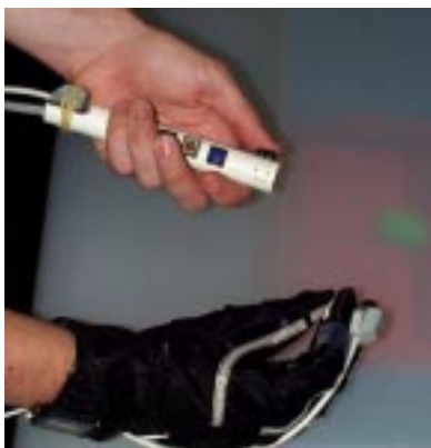
Fig. 1 Pinch Glove and Button Chord input devices showing placement of trackers.
