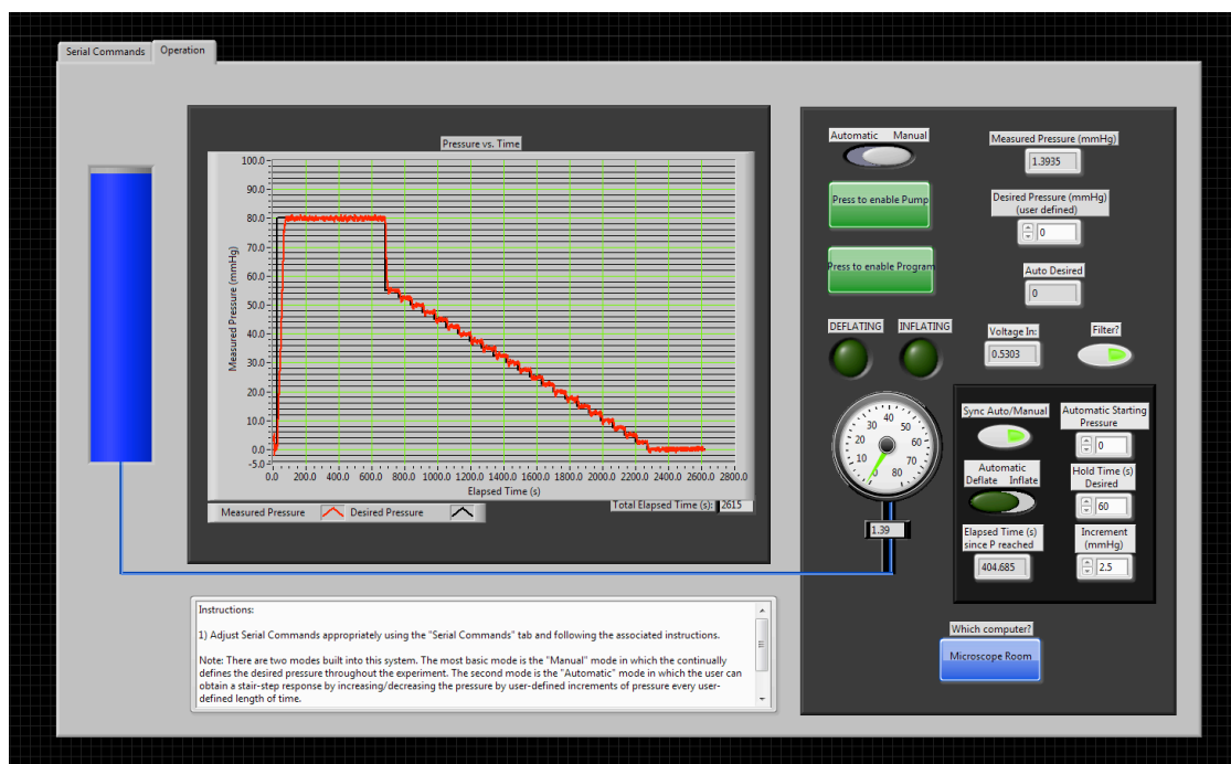
Figure B.1 Pressure Cuff Program GUI. This is a screenshot of the pressure cuff program graphical user interface (GUI) after completion one representative experiment. It shows the standard pressure curve used for all of the subsequent experiments for which the Intensity plots are shown.
