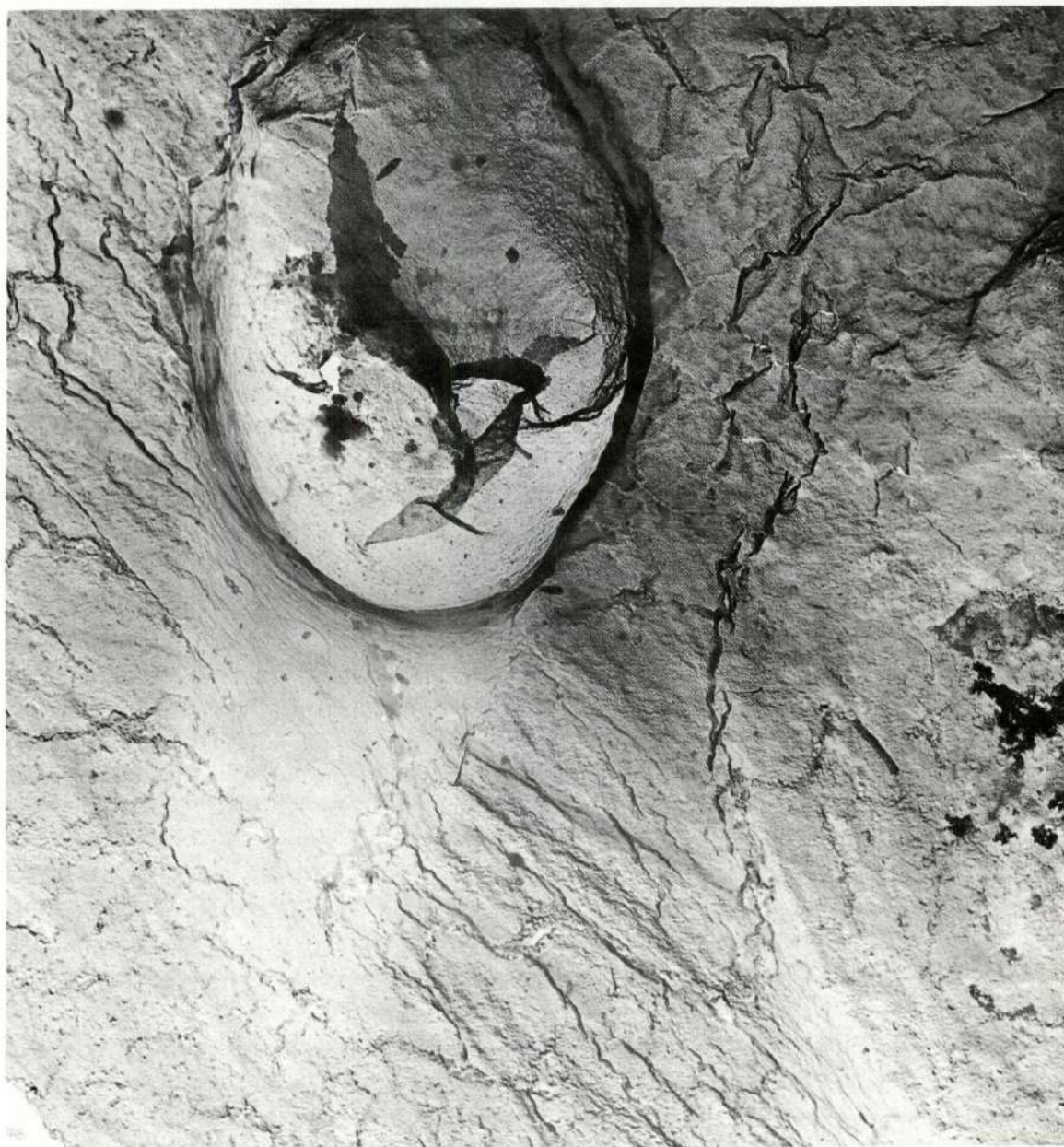
Figure 24. Electron Micrograph of the Outer Area of a Carborundum Co. Polycrystalline Alumina Sample. (Large numbers of microcracks radiate at random over the entire field (23,000X).)
