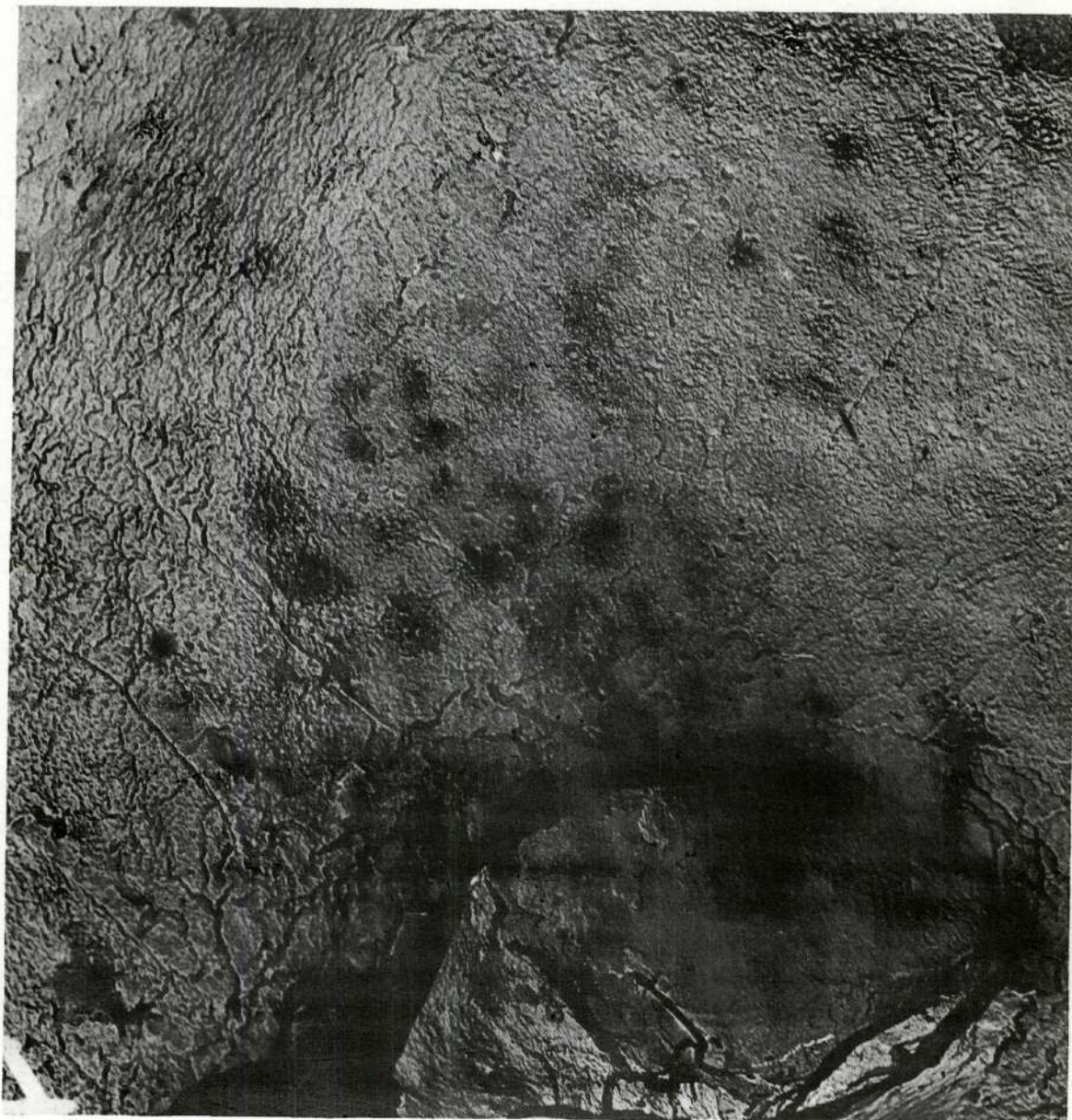
Figure 23. Electron Micrograph of the Area to One Side of the Barrier of a Carborundum Co. Polycrystalline Alumina Sample. (What appear to be microcracks radiate from the depression at the lower right (23,000X).)
