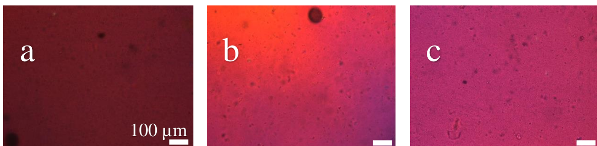
Figure 4.13 - POM images of melt-phase (a) 1 wt.% CNC/48EVOH, (b) 2.5 wt.% CNC/48EVOH, and (c) 5 wt.% CNC/EVOH nanocomposites produced by the STM technique.
