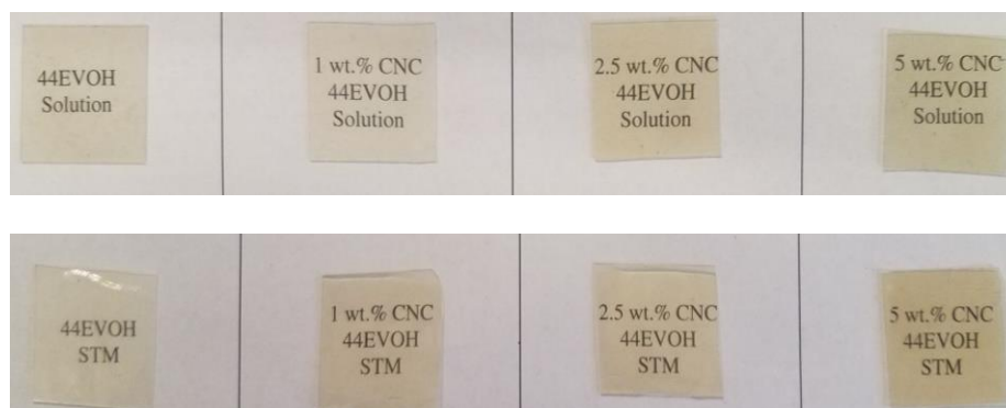
Figure 4.14 - Images of neat 44EVOH, 1 wt.% CNC/44EVOH, 2.5 wt.% CNC/44EVOH, and 5 wt.% CNC/44EVOH samples produced by solution casting and STM methods.
