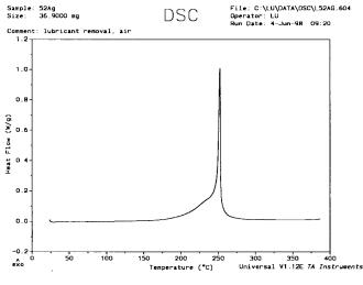
Fig. 5. DSC curve of a Ag flake in air.
