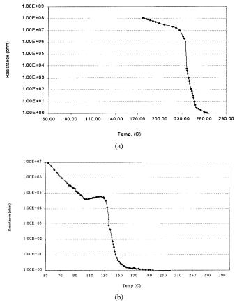
Fig. 4. Resistance change during heating of (a) an Ag flake and (b) an ICA.
