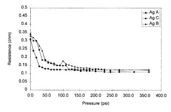
Fig. 7. Resistance changes of some Ag particles with external pressures.
