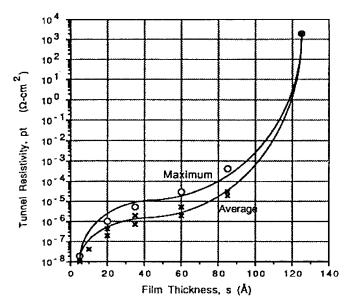
Fig. 8. Tunnel resistivity for thin films as a functions of film thickness [10].
