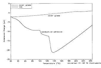
Fig. 6. Dimension changes of an ICA measured using a TMA.
