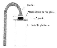
Fig. 2. Measurement setup of dimension changes using a TMA.
