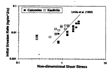
Figure 5. Variation of initial erosion rates with non-dimensional shear stress.
