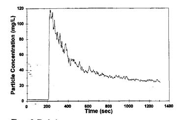
Figure 3. Typical concentration profile for erosion event.
