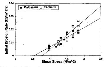
Figure 4. Initial erosion rates.
