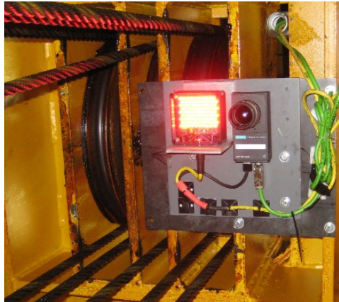
Figure 6.6: Camera and LED Array Mounting Configuration.
