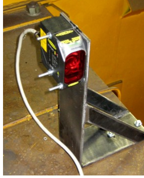
Figure 6.8: Banner LT7 Laser for Measuring the Position of the Bridge.
