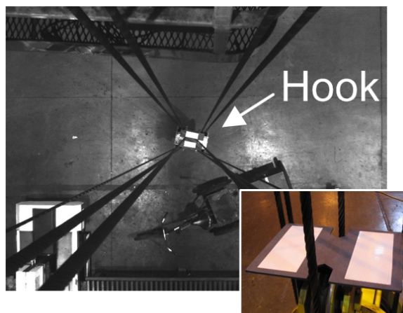
Figure 6.7: Image captured and processed by the machine vision system (large photo). Close up photograph of the fiducials mounted on the hook (sub photo).
