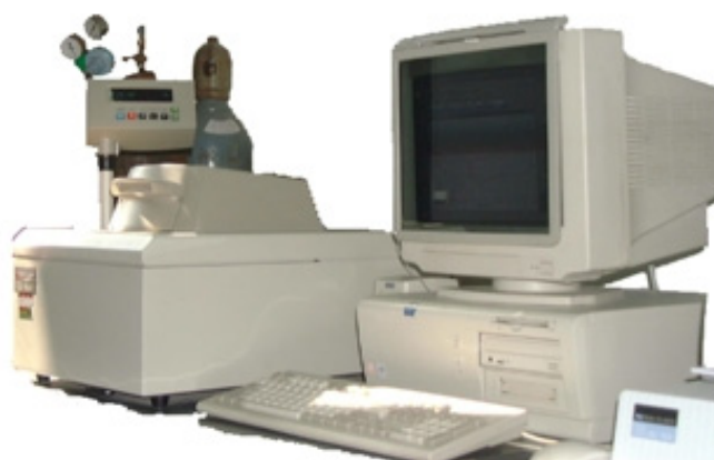
Figure 3.2.2 DSC Pyris 1 from PerkinElmer
