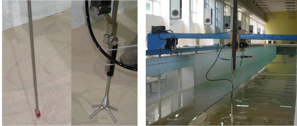
(a) Wave gauge (left) and ADV probe (right). (b) Carriage that moved along the flume with sensors.
