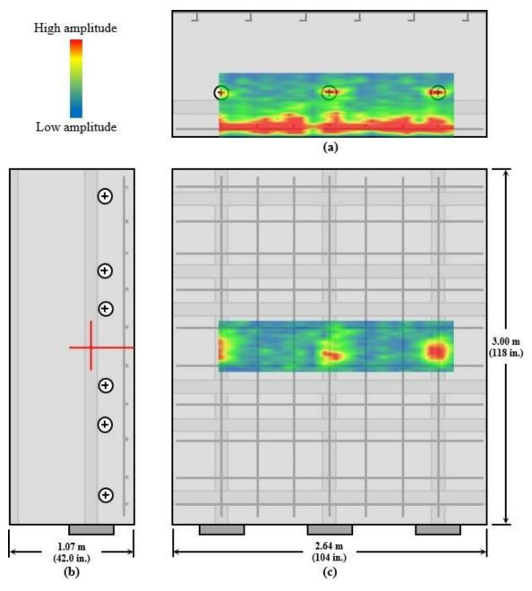
Figure 7.8: MIRA tomograms along path between middle horizontal ducts; (a) plan view with D-scan, (b) side elevation, and (c) front elevation with C-scan at depth of vertical ducts
