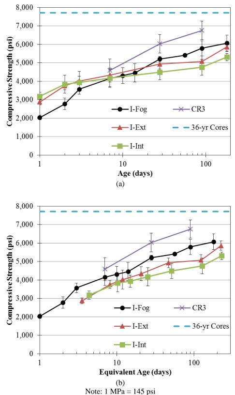
Figure 4.10: Compressive strength of first mock-up concrete as function of (a) chronological age and (b) equivalent age
