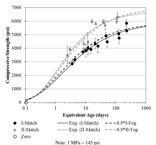
Figure 4.15: Compressive strength as a function of equivalent age of match-cured specimens with comparison to 90% relationship
