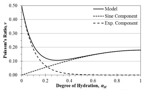
Figure 4.1: De Schutter and Taerwe (1996) Poisson's ratio model for concrete
