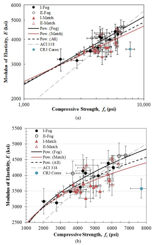
Figure 4.28: Modulus of elasticity with respect to compressive strength of all specimens with combined power law regressions shown on (a) log-log plot and (b) linear plot
