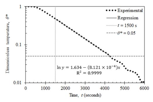
Figure 4.35: Dimensionless temperature history at center of specimen during thermal diffusivity testing
