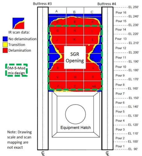
Figure 2.8: Diagram (Progress Energy, 2009) of delaminated region of CR3 PCC with outline of portion of bay in which mix design DM-5-Mod was used as indicated by Performance Improvement International (2010)
