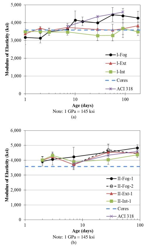
Figure 3.27: Modulus of elasticity of (a) first and (b) second mock-up concrete
