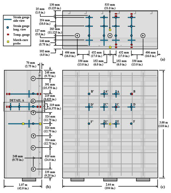
Figure 3.5: Drawings of gauge location and orientation: (a) plan, (b) side elevation, (c) front elevation
