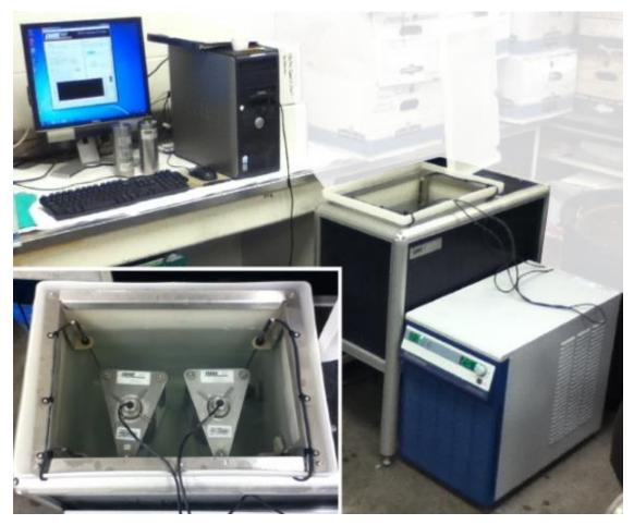
Figure 3.19: Set-up for AASHTO T 336 and Tex-428-A CTE testing
