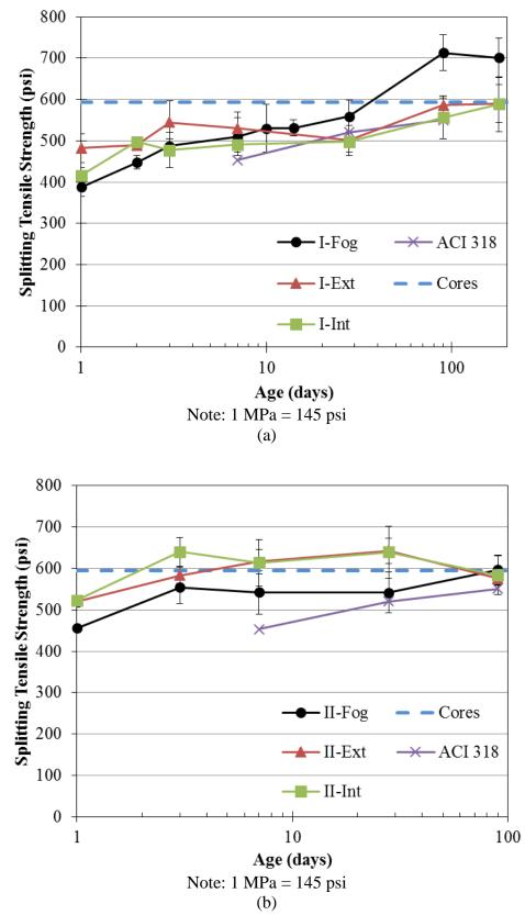
Figure 3.25: Splitting tensile strength of (a) first and (b) second mock-up concrete
