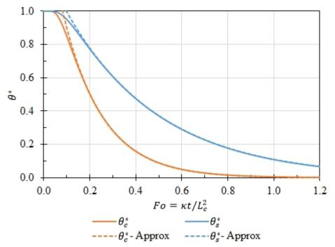
Figure 2.21: Convergence of first-term approximations with theoretical solutions for dimensionless temperature at the axis of an infinite right cylinder and midplane of an infinite plane slab
