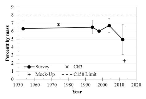
Figure 3.13: C<sub>3</sub>A content of cements produced in different years
