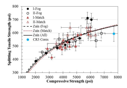
Figure 4.22: Splitting tensile strength with respect to compressive strength with Zain regressions
