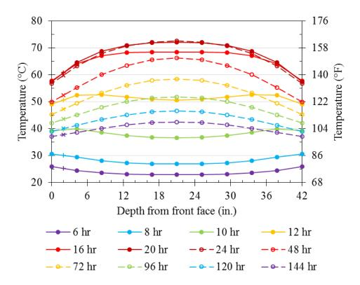
Note: 1 in. = 25.4 mm; interpolated points are indicated by + or × Figure 5.3: Temperature variation modeled by ConcreteWorks along line of symmetry through thickness of mock-up between 6 and 144 hours after concrete placement and linearly interpolated values at a depth of 51 mm (2 in.)
