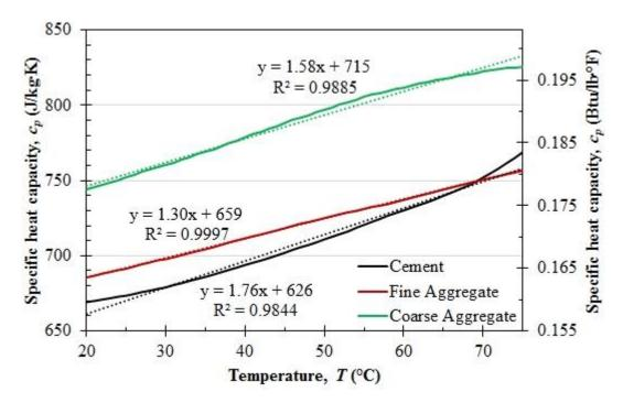
Figure 4.33: Specific heat capacities and linear regressions with respect to temperature
