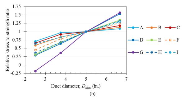
Figure 6.5: Influence of duct diameter on the (a)  $\sigma_1/f_{tsp}$  values at each point and (b) relative  $\sigma_1/f_{tsp}$  values at each point
