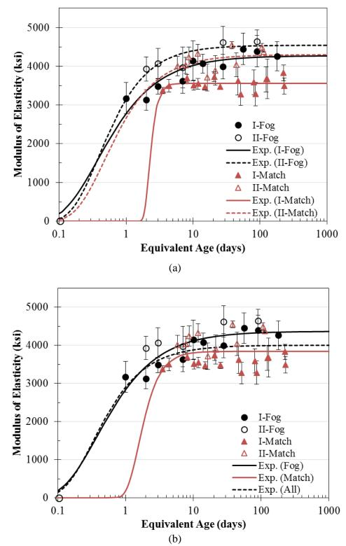
Figure 4.29: Modulus of elasticity with respect to equivalent age of all specimens with (a) individual and (b) combined exponential regressions
