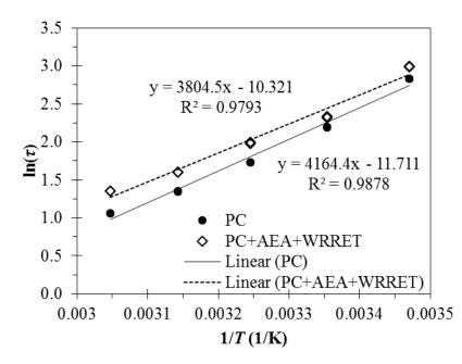
Figure 4.7: Variation of the natural logarithm of the hydration time parameter  $[\ln(\tau)]$  as a function of the reciprocal of the absolute temperature (1/T)
