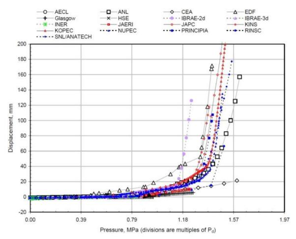
Figure 2.14: Predictions of radial displacement at mid-height of cylinder wall vs. internal pressure (Luk, 2000).
