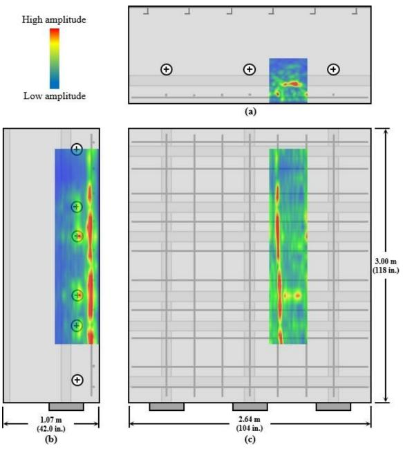
Figure 7.4: MIRA tomograms along path between vertical ducts; (a) plan view with Bscan, (b) side elevation with D-scan, and (c) front elevation with C-scan at depth of rebar cage
