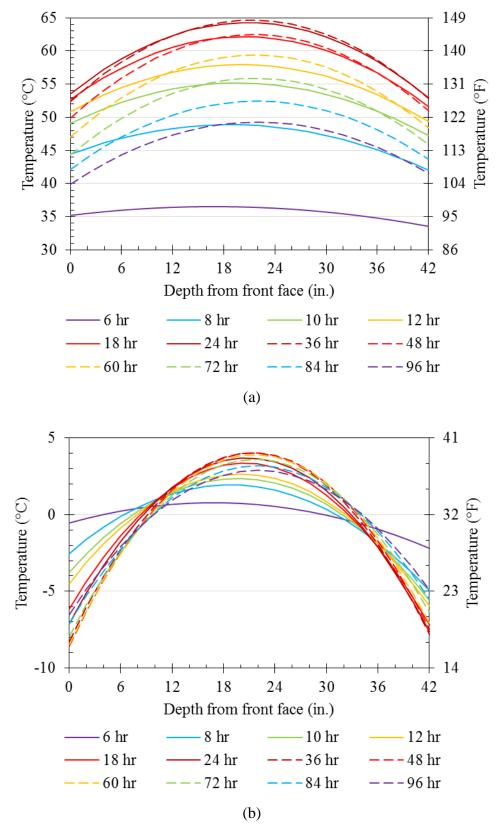
Figure 3.22: Quadratic regressions of temperature profiles through thickness of second mock-up shown with (a) actual magnitudes and (b) balance lines shifted to 0  $^{\circ}$ C (32  $^{\circ}$ F)
