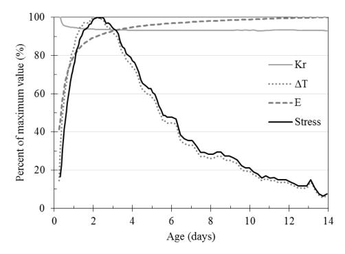
Figure 3.36: Degree of restraint, maximum temperature difference, modulus of elasticity, and tensile thermal stress of second mock-up normalized by maximum value during first 14 days
