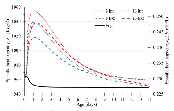
Figure 4.34: Specific heat capacity of mock-up concrete as function of age
