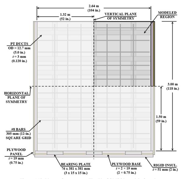
Figure 5.10: Planes of symmetry utilized in COMSOL model of mock-up
