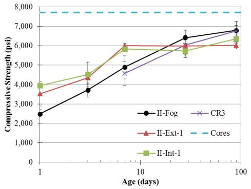
Figure B.2: Compressive strength results for second mock-up
