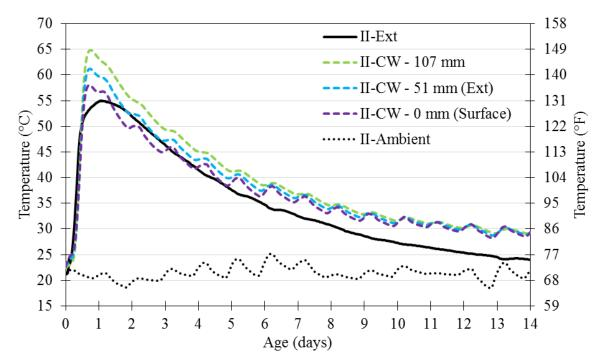
Figure 5.5: Second mock-up Ext temperatures and ConcreteWorks (CW) near-surface temperatures during first 14 days
