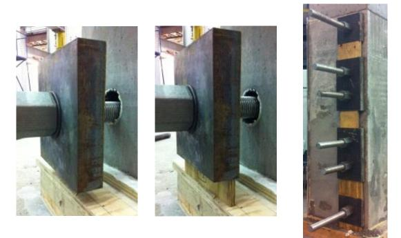
(a) (b) (c) Figure 3.8: (a) Post-tensioning rod resting on duct embedded in concrete, (b) plywood spacer beneath bearing plate lifting rod to center of duct, and (c) full stack of plates and plywood spacers against the concrete
