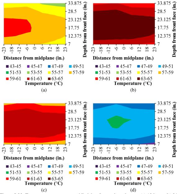
Figure 3.23: Temperature contours at midheight of second mock-up at (a) 12 hours (b) 24 hours (c) 48 hours, and (d) 96 hours after concrete placement began
