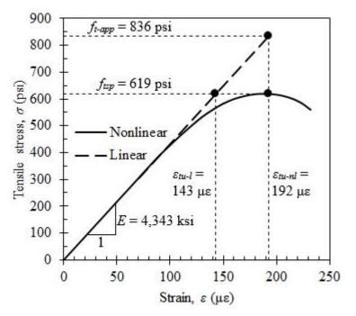
Note: 1 MPa = 145 psi Figure 3.43: Hypothetical stress-strain curve fitting mock-up concrete properties
