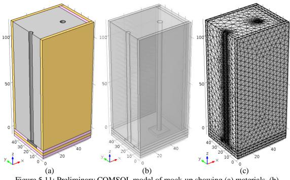
Figure 5.11: Preliminary COMSOL model of mock-up showing (a) materials, (b) embedded components, and (c) finite element mesh
