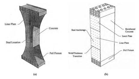
Figure 2.12: Uniaxial specimens for strain concentration and liner tear studies (Hessheimer and Dameron, 2006)
