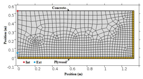
Note: 1 m = 39.37 in.; using symmetry, front right quarter of mock-up modeled, whereas front left quarter was modeled in ConcreteWorks (Figure 5.1) Figure 5.8: Geometry, mesh, and materials for COMSOL model replicating ConcreteWorks
