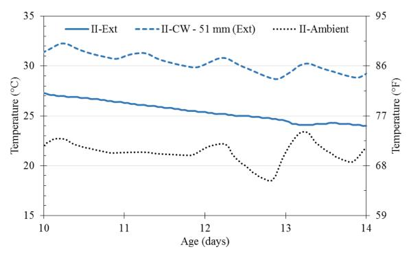
Figure 5.6: Comparison of experimental and modeled Ext temperature variation with ambient temperatures
