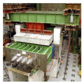
Figure 2.16: Experimental setup for PACE 1450 (Herrmann et al., 2008).
