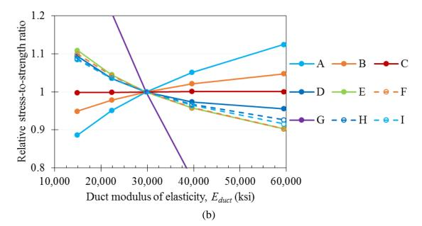
Figure 6.7: Influence of duct modulus of elasticity on the (a)  $\sigma_1/f_{tsp}$  values at each point and (b) relative  $\sigma_1/f_{tsp}$  values at each point
