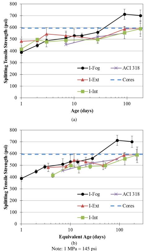
Figure 4.16: Splitting tensile strength of first mock-up concrete as function of (a) chronological age and (b) equivalent age
