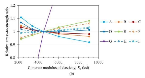
Figure 6.3: Influence of concrete modulus of elasticity on the (a)  $\sigma_1/f_{tsp}$  values at each point and (b) relative  $\sigma_1/f_{tsp}$  values at each point
