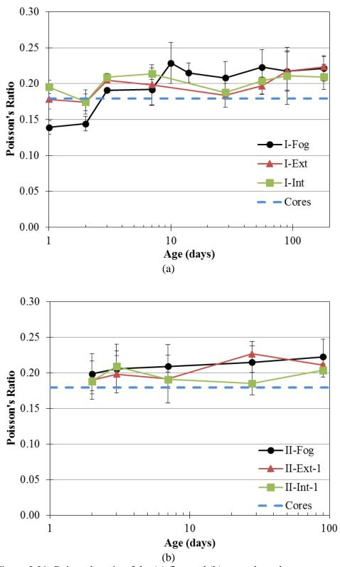
Figure 3.29: Poisson's ratio of the (a) first and (b) second mock-up concrete
