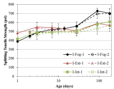
Figure B.3: Splitting tensile strength results for first mock-up sorted by truck and curing condition
