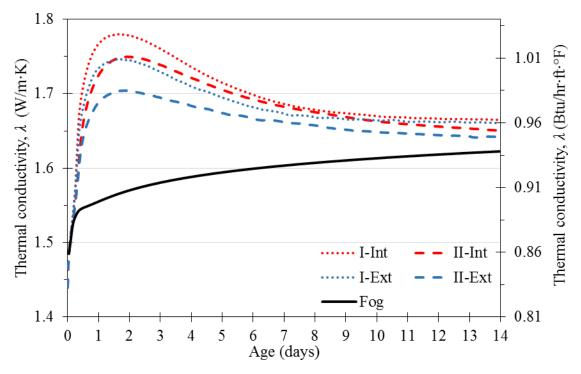
Figure 4.39: Calculated thermal conductivity values for mock-up concrete
