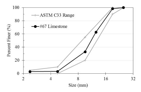
Figure 3.15: Gradation curve of limerock coarse aggregate (1 in. = 25.4 mm)
