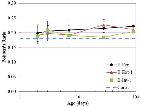
Figure B.8: Poisson's ratio results for second mock-up sorted by truck and curing condition
