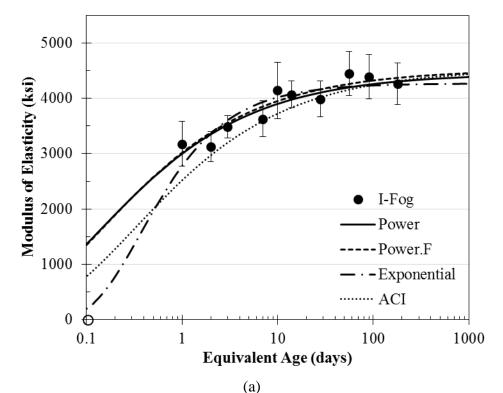
Figure 4.30: Modulus of elasticity with respect to equivalent age of (a) I-Fog, (b) II-Fog, (c) I-Match, and (d) II-Match specimens
