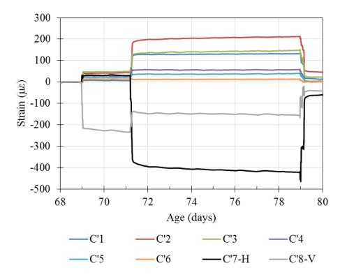
Figure 3.42: Post-tensioning strains measured in C' gauges of second mock-up
