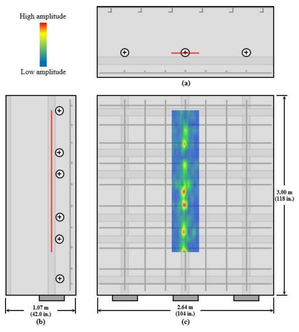
Figure 7.7: MIRA tomogram along middle vertical duct; (a) plan view, (b) side elevation, and (c) front elevation with C-scan at depth of vertical ducts
