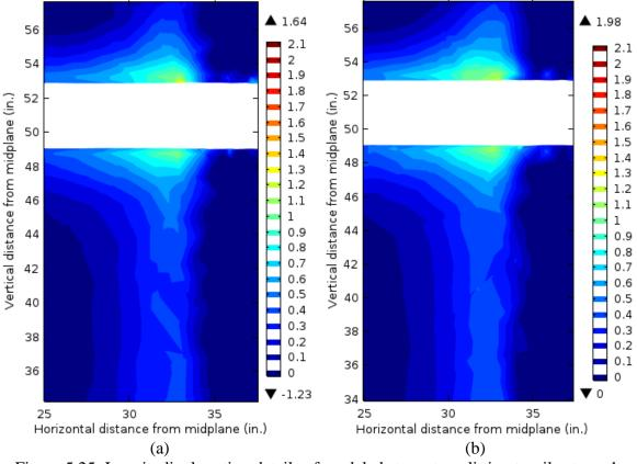
Figure 5.25: Longitudinal section details of modeled stress-to-splitting tensile strength ratio in plane of horizontal ducts (a) without accounting for curing history and (b) accounting for curing history
