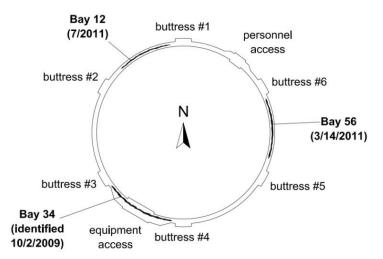
Note: Delaminations are not drawn to scae Figure 2.7: Plan diagram showing locations and date of occurrence or identification of CR3 wall delaminations
