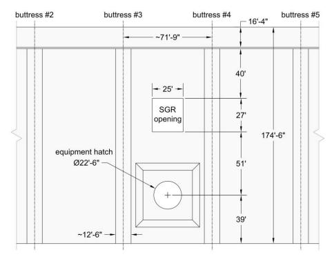
Note: Horizontal dimensions are approximate due to unfolding of curved surface Figure 2.4: Diagram of unfolded elevation showing the SGR opening location
