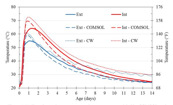
Figure 5.15: Experimental temperatures and temperatures modeled by COMSOL and ConcreteWorks (CW)
