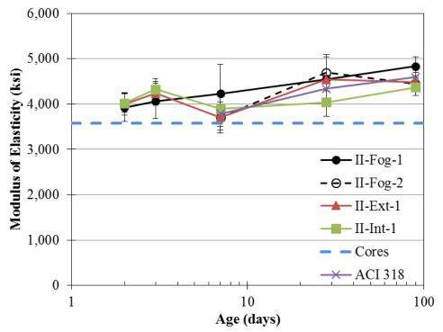
Figure B.6: Modulus of elasticity results for second mock-up sorted by truck and curing condition
