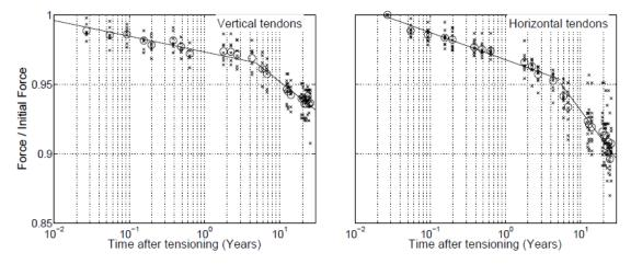
Figure 2.10: Remaining force from gauges normalized by initial force (logarithmic timescale) (Anderson, 2007).
