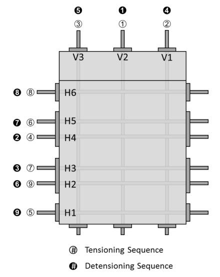
Figure 3.10: Identification of post-tensioning rods and post-tensioning and detensioning sequences
