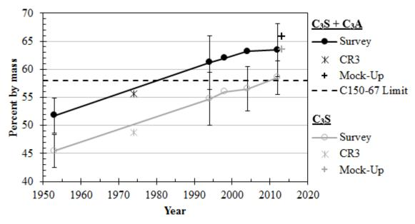
Figure 3.12: C<sub>3</sub>S and C<sub>3</sub>S plus C<sub>3</sub>A contents of cements produced in different years
