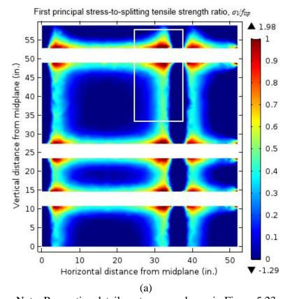
Note: Respective detail contours are shown in Figure 5.23 Figure 5.22: Longitudinal section views of modeled stress-to-splitting tensile strength ratio in post-tensioned mock-up concrete in (a) plane of horizontal ducts, (b) plane of contact between horizontal and vertical ducts, and (c) plane of the vertical ducts
