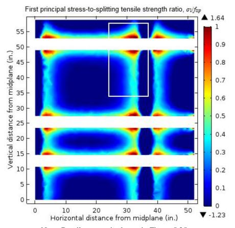
Note: Detail contour is shown in Figure 5.25a Figure 5.24: Ratio of modeled stress to splitting tensile strength in plane of horizontal ducts without accounting for curing history
