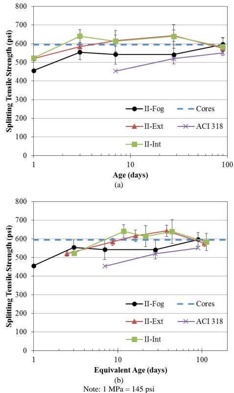
Figure 4.17: Splitting tensile strength of second mock-up concrete as function of (a) chronological age and (b) equivalent age
