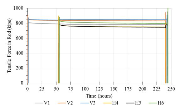
Figure 3.11: Tensile forces in post-tensioning rods
