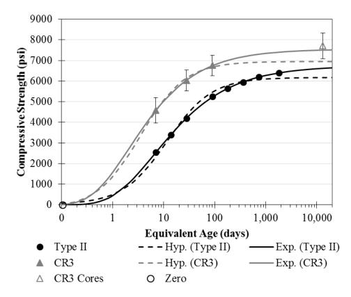
Figure 4.13: Compressive strength development of CR3 PCC concrete and typical concrete made with Type II cement (U.S. Bureau of Reclamation, 1981)
