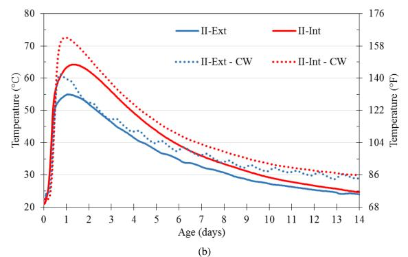
Figure 5.4: Experimental temperatures and corresponding ConcreteWorks (CW) results for (a) first and (b) second mock-up
