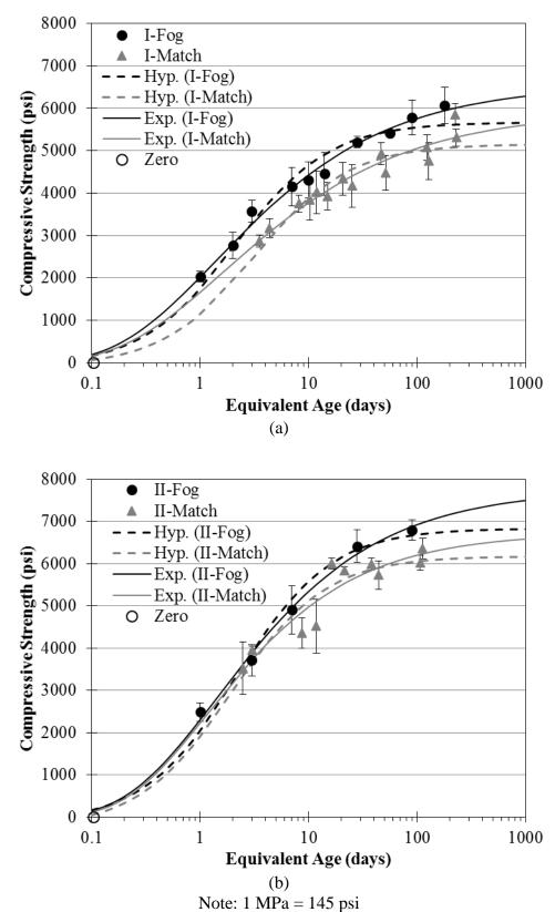
Figure 4.12: Compressive strength as a function of equivalent age of fog- and matchcured specimens from (a) first and (b) second mock-up
