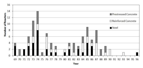
Figure 2.1: Containment types of currently licensed U.S. commercial nuclear power reactors by year of issuance of initial operating license. Data from NRC Information Digest 2010-2011 (U.S. Nuclear Regulatory Commission, 2010).
