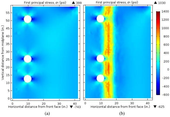
Figure 5.19: Transverse section view of modeled stresses in post-tensioned mock-up concrete (a) between vertical ducts and (b) at edge of vertical duct
