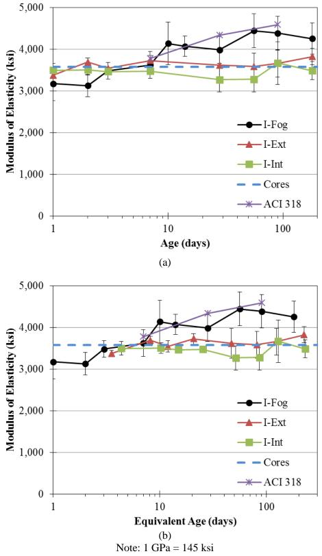
Figure 4.25: Modulus of elasticity of first mock-up concrete as function of (a) chronological age and (b) equivalent age
