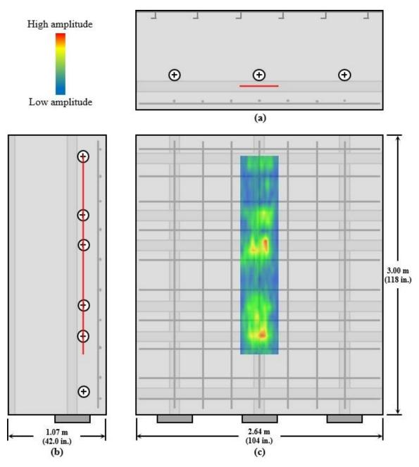
Figure 7.6: MIRA tomogram along middle vertical duct; (a) plan view, (b) side elevation, and (c) front elevation with C-scan at depth of horizontal ducts
