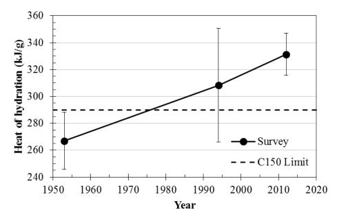
Figure 3.14: Cumulative 7-day heat of hydration of cements produced in different years
