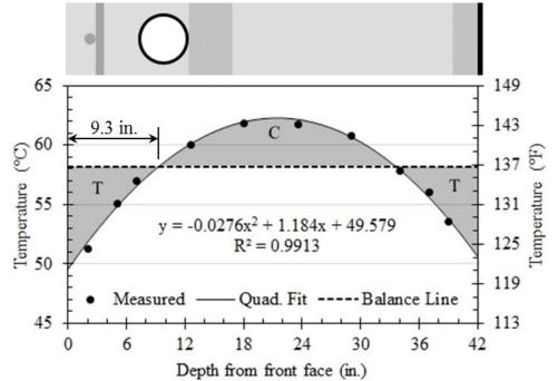
Figure 3.21: Section detail and temperature profile through thickness of second mock-up measured by C gauges at time of maximum temperature differential
