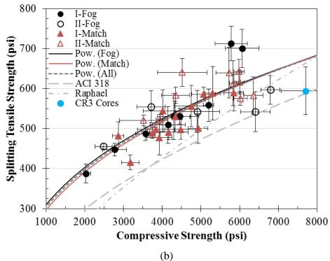
Note: 1 MPa = 145 psi Figure 4.20: Splitting tensile strength with respect to compressive strength of all specimens shown on (a) log-log plot and (b) linear plot
