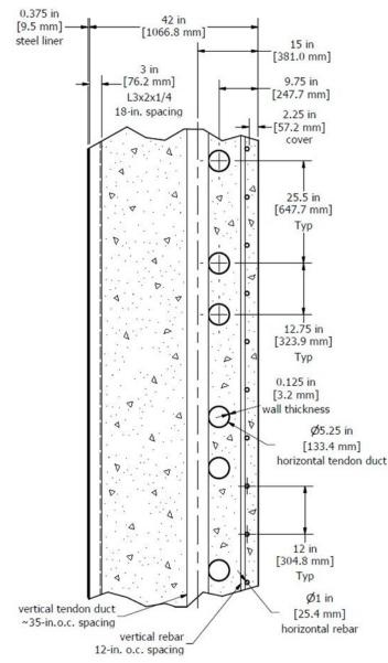
Note: Displayed components are not necessarily in the same vertical plane Figure 3.1: Typical section of CR3 PCC wall
