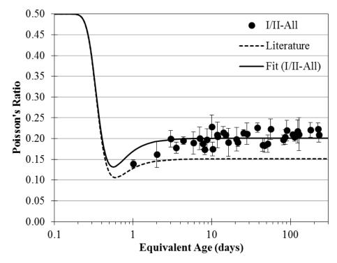
Figure 4.32: Poisson's ratio of all mock-up concrete specimens
