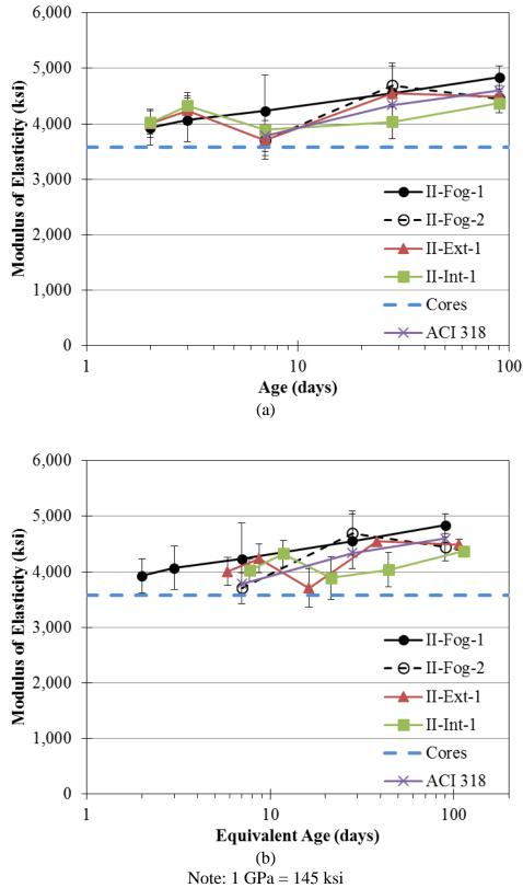
Figure 4.26: Modulus of elasticity of second mock-up concrete as function of (a) chronological age and (b) equivalent age
