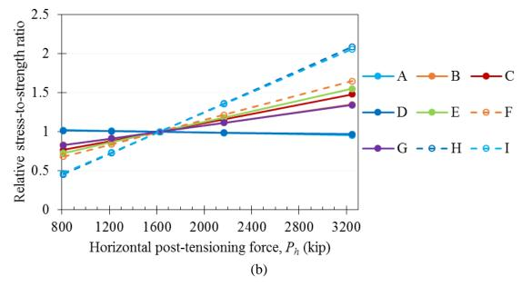
Figure 6.9: Influence of horizontal post-tensioning force on the (a)  $\sigma_1/f_{tsp}$  values at each point and (b) relative  $\sigma_1/f_{tsp}$  values at each point
