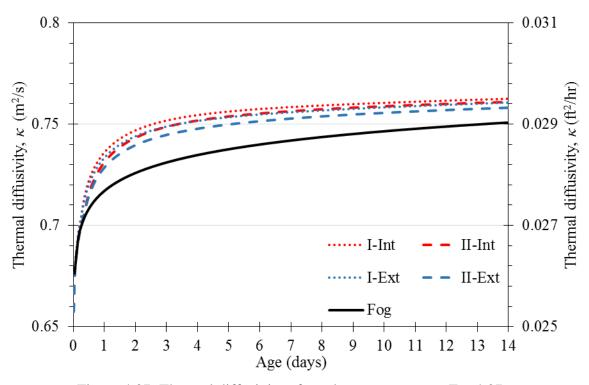
Figure 4.37: Thermal diffusivity of mock-up concrete per Eq. 4.37
