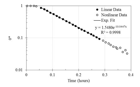
Figure 2.22: Dimensionless temperature history data sampled from diffusivity test in De Schutter and Taerwe (1995)
