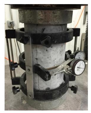
Figure 3.30: Cracked specimen from modulus of elasticity and Poisson's ratio testing
