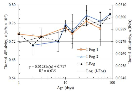
Figure 4.36: Thermal diffusivity results
