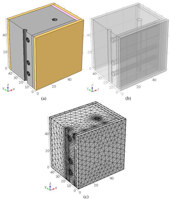
(c) Figure 5.14: Diagrams of final COMSOL model showing (a) materials, (b) embedded components, and (c) finite element mesh
