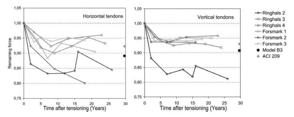
Figure 2.9: Remaining prestressing force from lift-off tests normalized by initial prestressing force. Each point represents the average of all values obtained at the containment at the corresponding inspection. Horizontal (left) and vertical tendons (right) (Anderson, 2007).
