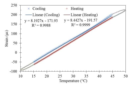
Figure 3.33: Strain as a function of temperature for determination of CTE in accordance with Tex-428-A
