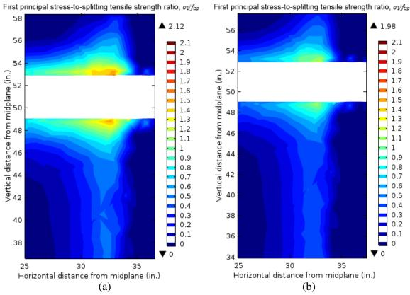
Figure 5.28: Detail contours of modeled stress-to-splitting tensile strength ratio in plane of horizontal ducts with (a) CR3 PCC post-tensioning loads and (b) mock-up posttensioning loads
