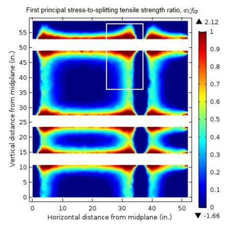
Note: Detail contour is shown in Figure 5.28a Figure 5.27: Ratio of modeled stress to splitting tensile strength in plane of horizontal ducts with CR3 PCC post-tensioning loads
