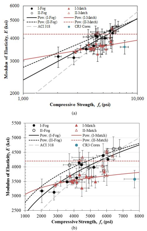
Figure 4.27: Modulus of elasticity with respect to compressive strength of all specimens with individual power law regressions shown on (a) log-log plot and (b) linear plot
