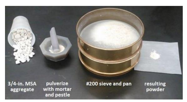
Figure 4.2: Coarse aggregate sample preparation for differential scanning calorimetry
