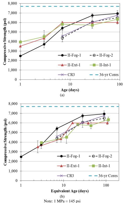
Figure 4.11: Compressive strength of second mock-up concrete as function of (a) chronological age and (b) equivalent age
