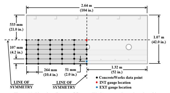
Figure 5.1: Plan view diagram of ConcreteWorks symmetries and results grid
