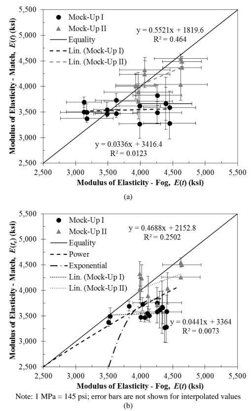
Figure 4.31: Modulus of elasticity of match-cured specimens with respect to that of fogcured specimens at same (a) chronological age and (b) equivalent age
