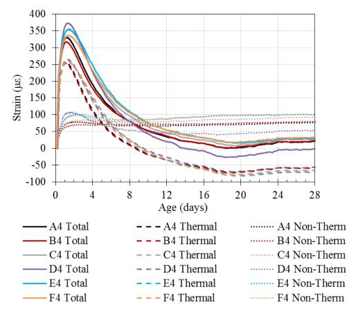
Figure 3.40: Total, thermal, and non-thermal strains measured in second mock-up during first 28 days
