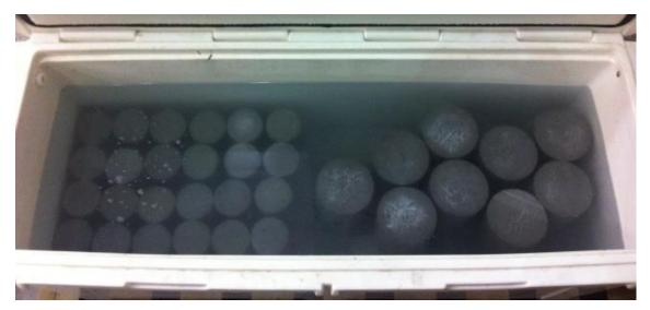
Figure 3.17: Specimens in match-curing storage tank
