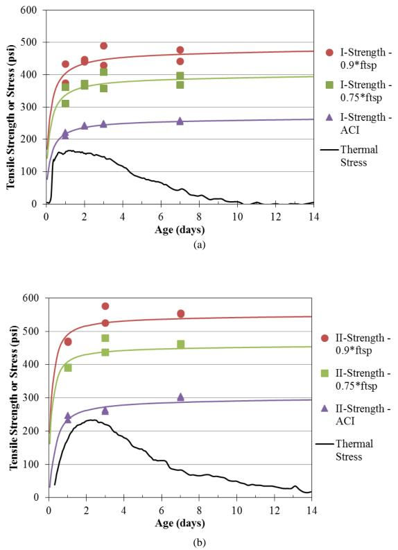
Figure 3.37: Thermal stresses and predicted direct tensile strength of (a) first and (b) second mock-up concrete
