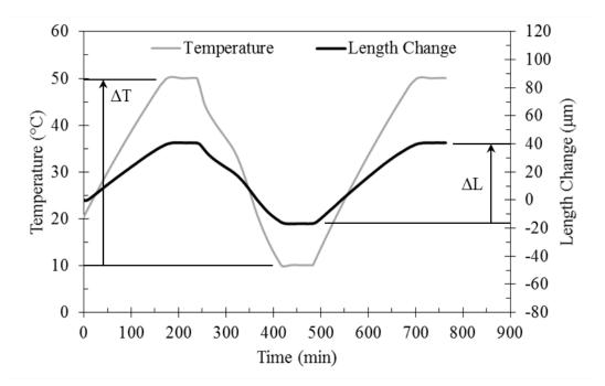
Figure 3.32: Length change and temperature histories for determination of CTE in accordance with AASHTO T 336
