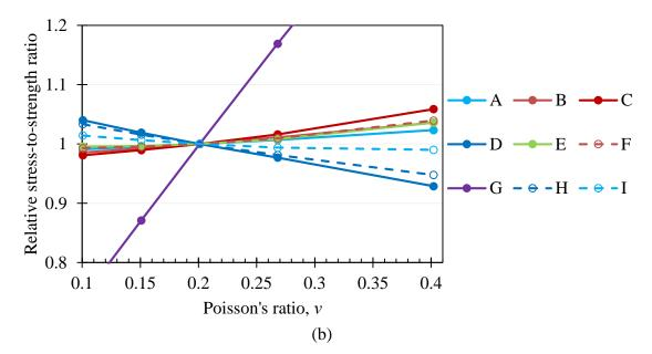
Figure 6.4: Influence of concrete Poisson's ratio on the (a)  $\sigma_1/f_{tsp}$  values at each point and (b) relative  $\sigma_1/f_{tsp}$  values at each point
