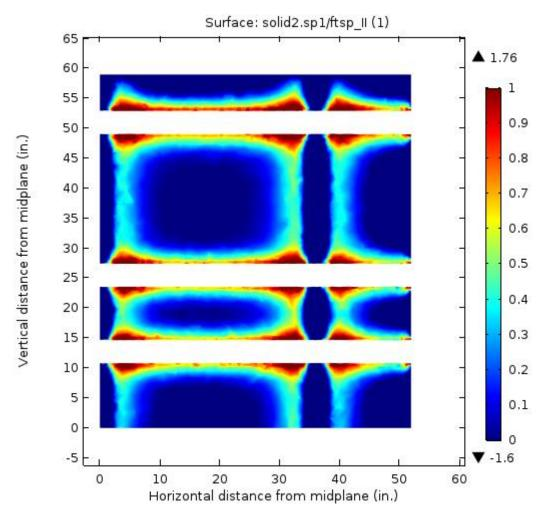
Figure 5.29: Ratio of modeled stress to splitting tensile strength in plane of circumferential ducts in CR3 PCC when post-tensioned without accounting for curing history
