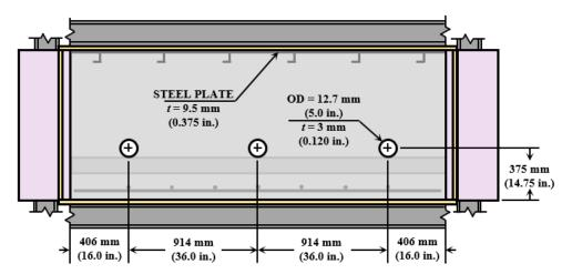
Note: Post-tensioning anchorage reinforcement is not shown Figure 3.2: Plan drawing of mock-ups as cast and cured
