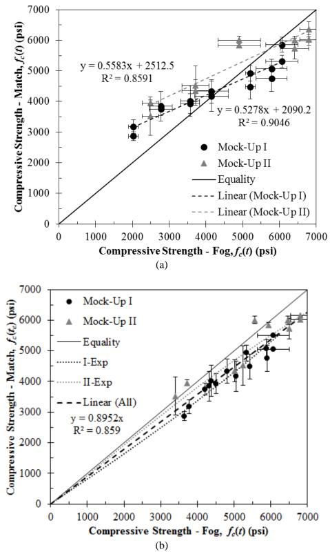
Note: 1 MPa = 145 psi; error bars are not shown for interpolated values Figure 4.14: Compressive strength of match-cured specimens with respect to that of fogcured specimens at same (a) chronological age and (b) equivalent age
