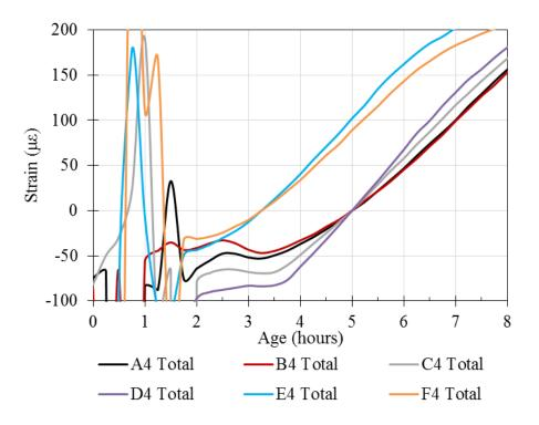
Figure 3.39: Total strains measured in mock-up during first 12 hours after beginning of concrete placement
