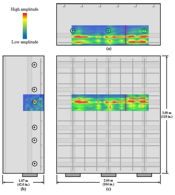
Figure 7.9: MIRA tomograms along horizontal duct; (a) plan view with D-scan, (b) side elevation with B-scan, and (c) front elevation with full-depth C-scan
