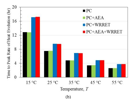
Figure 4.5: (a) Peak rates of heat evolution and (b) times to peak rate of heat evolution for tested cement pastes
