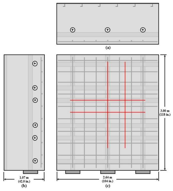
Figure 7.2: Orientation of MIRA scan paths for second mock-up; (a) plan view, (b) side elevation, and (c) front elevation
