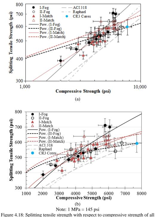
specimens shown on (a) log-log plot and (b) linear plot
