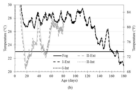
Figure 3.20: Concrete specimen curing temperature histories through (a) 28 days and (b) 180 days
