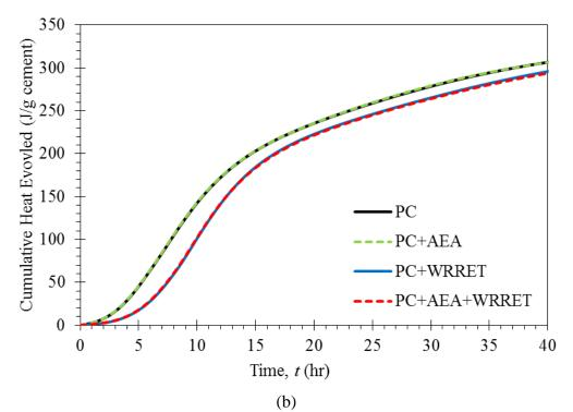
Figure 4.4: (a) Rate of heat evolution and (b) cumulative heat of hydration of representative mock-up cement pastes at 25 °C (77 °F)
