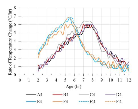
Figure 3.38: Rate of temperature change of second mock-up concrete
