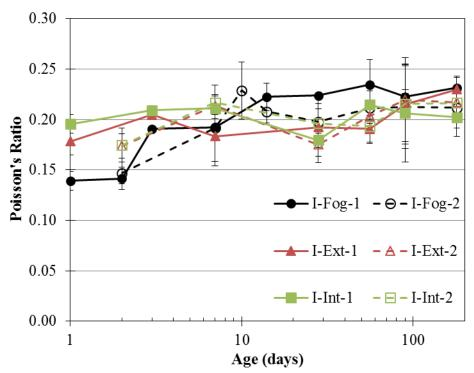
Figure B.7: Poisson's ratio results for first mock-up sorted by truck and curing condition
