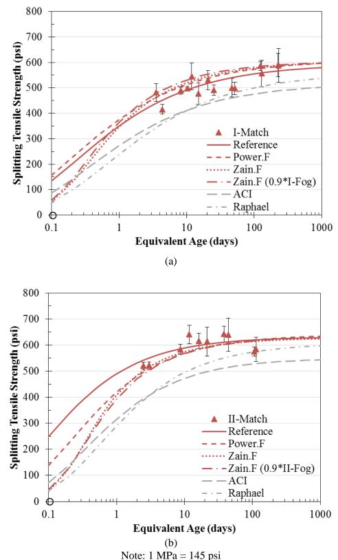
Figure 4.23: Match-cured splitting tensile strengths with respect to equivalent age and corresponding regressions for (a) first and (b) second mock-up
