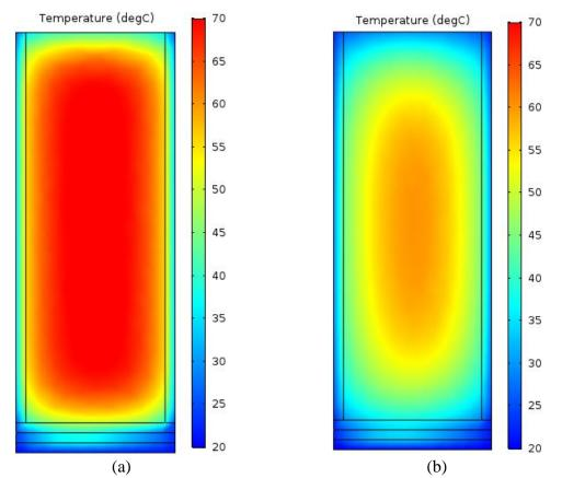
Figure 5.13: Preliminary mock-up temperature profiles modeled halfway between the vertical post-tensioning ducts (a) 24 and (b) 60 hours after concrete placement
