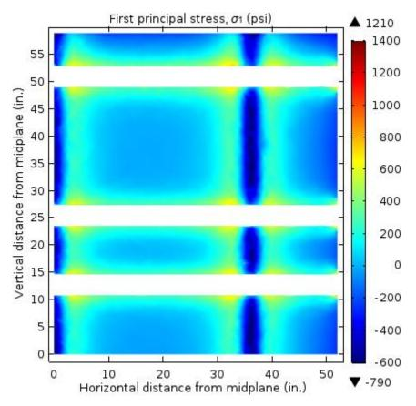
Figure 5.21: Longitudinal section view in plane of horizontal ducts of modeled stresses in post-tensioned mock-up concrete
