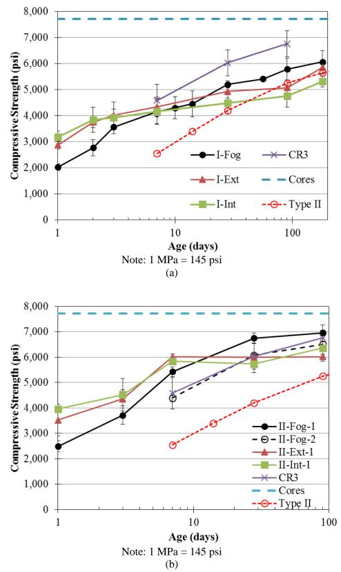
Figure 3.24: Compressive strength of (a) first and (b) second mock-up concrete
