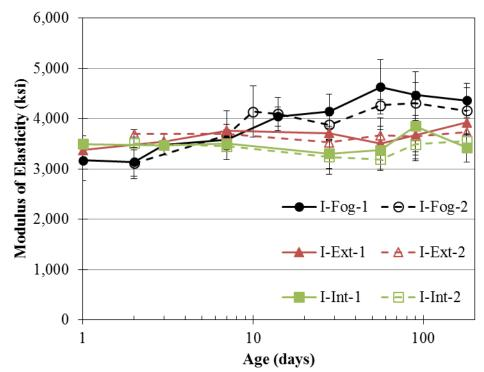
Figure B.5: Modulus of elasticity results for first mock-up sorted by truck and curing condition
