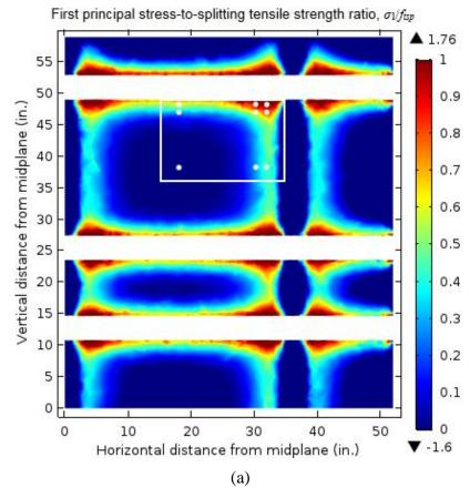
Figure 6.1: Longitudinal section view of modeled stress-to-splitting tensile strength ratio with points of evaluation identified, (a) full section and (b) detail
