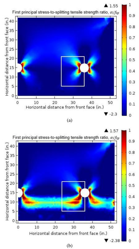
Note: Respective detail contours are shown in Figure 5.18 Figure 5.17: Plan views of modeled stress-to-splitting tensile strength ratio in posttensioned mock-up concrete (a) between horizontal ducts and (b) at top edge of horizontal duct
