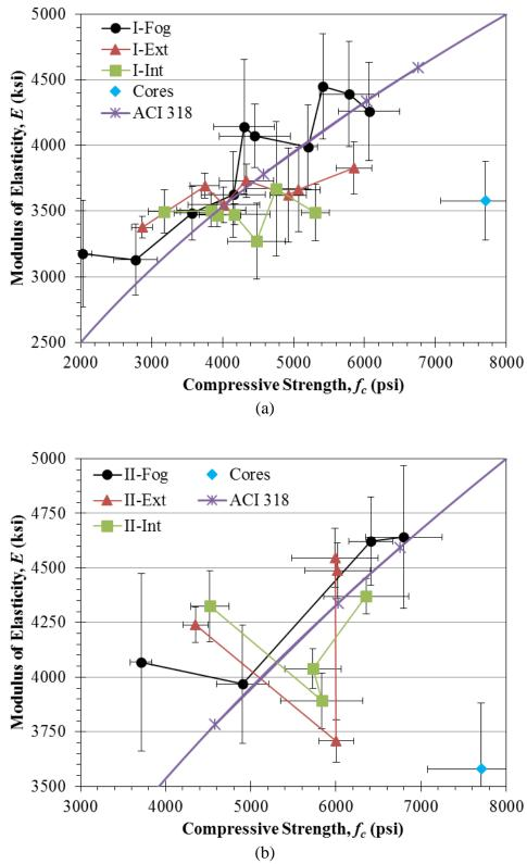
Figure 3.28: Modulus of elasticity versus compressive strength for (a) first and (b) second mock-up concrete
