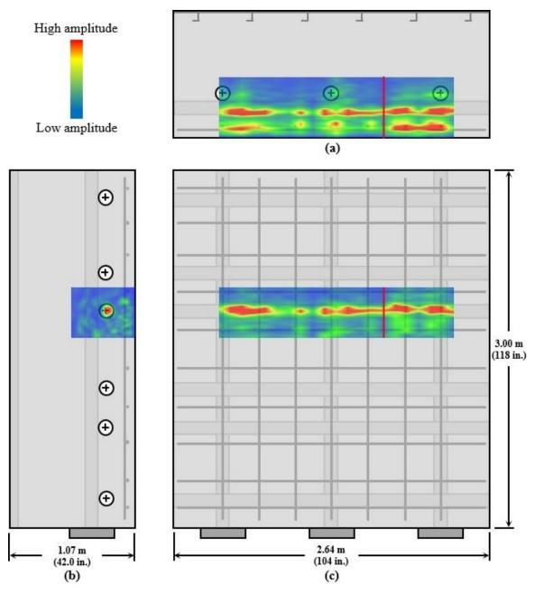
Figure 7.10: MIRA tomograms along horizontal duct; (a) plan view with D-scan, (b) side elevation with B-scan, and (c) front elevation with C-scan at depth of horizontal ducts
