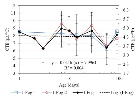
Figure 3.31: CTE results for concrete from the first mock-up tested in accordance with Army Corps CRD-C 39-81
