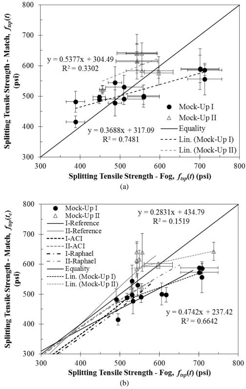
Note: 1 MPa = 145 psi; error bars are not shown for interpolated values Figure 4.24: Splitting tensile strength of match-cured specimens with respect to that of fog-cured specimens at same (a) chronological age and (b) equivalent age
