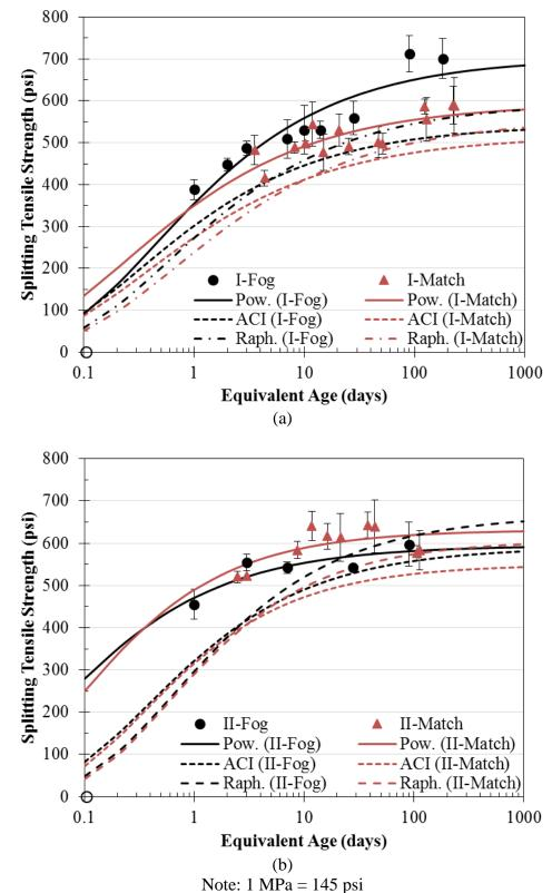
Figure 4.19: Splitting tensile strength as a function of equivalent age of fog- and matchcured specimens from (a) first and (b) second mock-up
