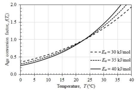
Figure 2.18: Influence of activation energy on age conversion factor;  $T_r = 23$  °C (73.4 °F); 1 kJ/mol = 429.9 Btu/lbmol
