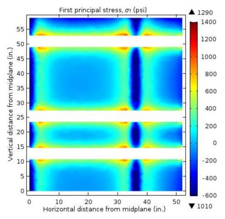
Figure 5.26: Modeled stresses in plane of horizontal ducts with CR3 PCC post-tensioning loads
