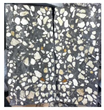
Figure 3.26: Failed I-Int-1 splitting tensile strength specimen tested at 1 day
