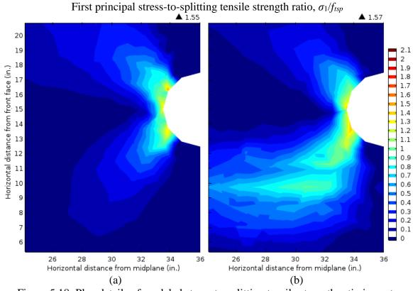
Figure 5.18: Plan details of modeled stress-to-splitting tensile strength ratio in posttensioned mock-up concrete (a) between horizontal ducts and (b) at edge of horizontal duct
