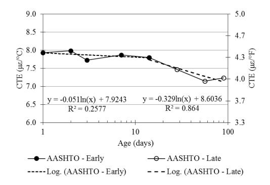
Figure 3.35: Piecewise-linear regression of AASHTO T 336 results with hinge at 14 days
