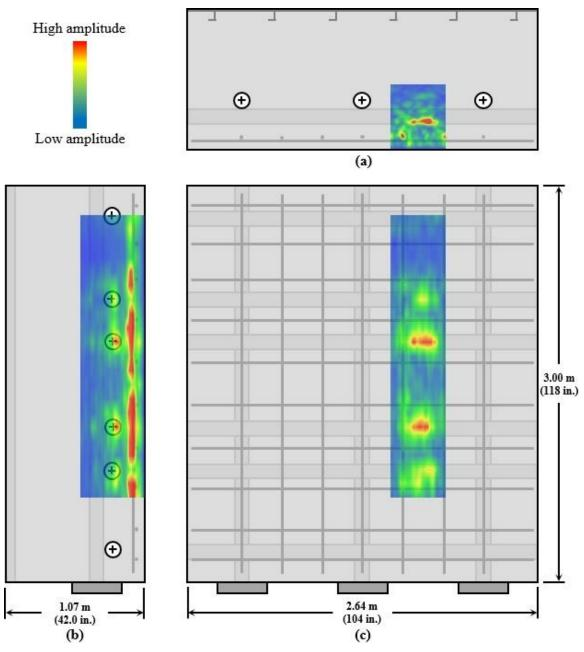
Figure 7.5: MIRA tomograms along path between vertical ducts; (a) plan view with Bscan, (b) side elevation with D-scan, and (c) front elevation with C-scan at depth of horizontal ducts
