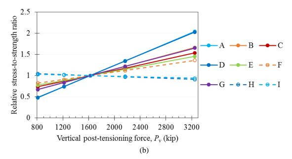
Figure 6.8: Influence of vertical post-tensioning force on the (a)  $\sigma_1/f_{tsp}$  values at each point and (b) relative  $\sigma_1/f_{tsp}$  values at each point
