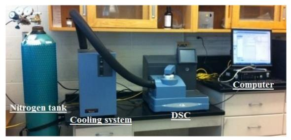
Figure 4.3: Full set-up for differential scanning calorimetry
