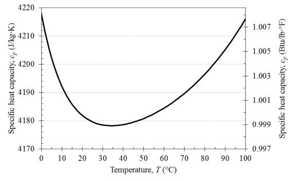
Figure 2.20: Specific heat capacity of water as a function of temperature at 1 atm (101.325 kPa) pressure (Osborne et al., 1939)
