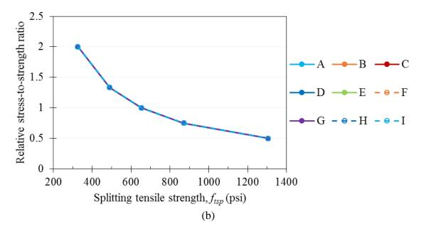
Figure 6.2: Influence of concrete spitting tensile strength on the (a)  $\sigma_1/f_{tsp}$  values at each point and (b) relative  $\sigma_1/f_{tsp}$  values at each point
