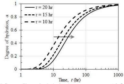
(b) Influence of increasing hydration time parameter  $\tau$ ;  $\alpha_u = 1.0$ ,  $\beta = 1.0$ Figure 2.17: Influence of hydration parameters on the progression of hydration
