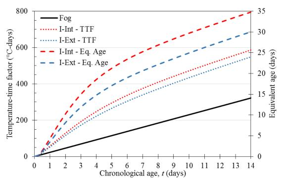
Figure 4.8: Maturity indices of concrete specimens for first mock-up
