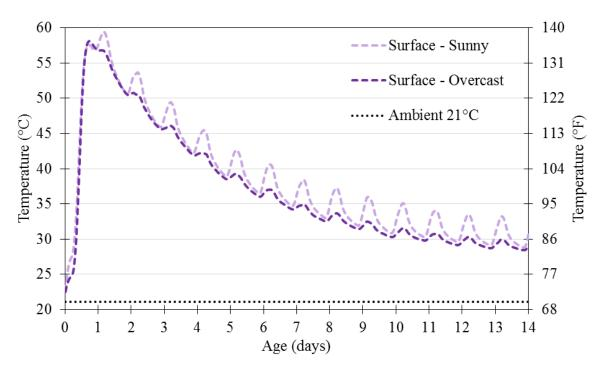
Figure 5.7: Concrete surface temperatures modeled in ConcreteWorks for constant ambient temperature of 21 °C (70 °F) and sunny and overcast conditions
