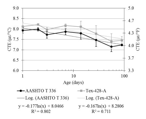
Figure 3.34: CTE results for concrete from the first truck of the first mock-up tested in accordance with AASHTO 336 and the Texas Method
