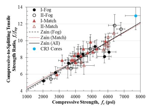
Figure 4.21: Compressive strength-to-splitting tensile strength  $(f_c/f_{tsp})$  ratio with respect to compressive strength
