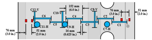
Figure 3.6: Detail A (see Figure 3.5) of series of transverse gauges
