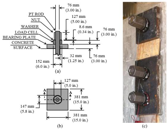
Figure 3.7: Post-tensioning anchorage system (a) Section A-A, (b) elevation, and (c) picture
