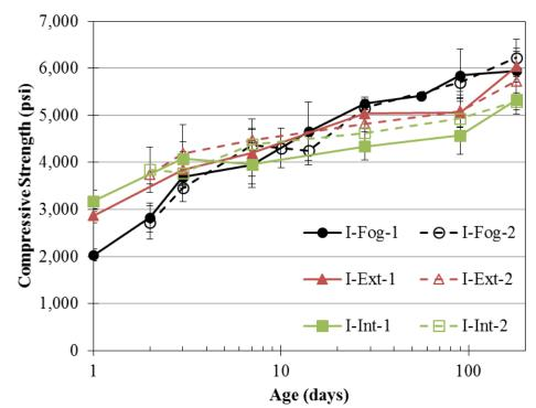
Figure B.1: Compressive strength results for first mock-up sorted by truck and curing condition
