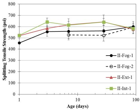
Figure B.4: Splitting tensile strength results for second mock-up sorted by truck and curing condition
