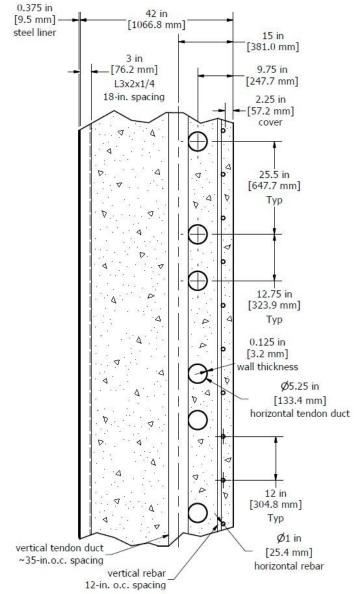
Note: Displayed components are not necessarily in the same vertical plane Figure 2.3: Typical section of CR3 containment wall
