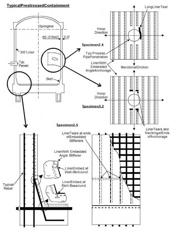
Figure 2.13: Panel mock-ups for investigation of liner behavior at local regions of containment (Hessheimer and Dameron, 2006).
