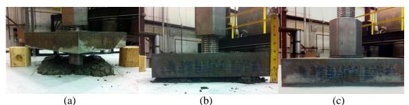
Figure 3.9: (a) Fresh grout placed on concrete surface beneath bearing plate, (b) bearing plate lowered onto grout, and (c) finished grout after hammering bearing plate and tightening nut
