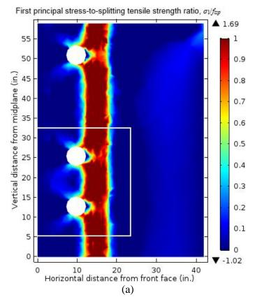
Figure 5.20: Transverse section view of modeled stress-to-splitting tensile strength ratio in post-tensioned mock-up concrete at edge of vertical duct, (a) full section and (b) detail
