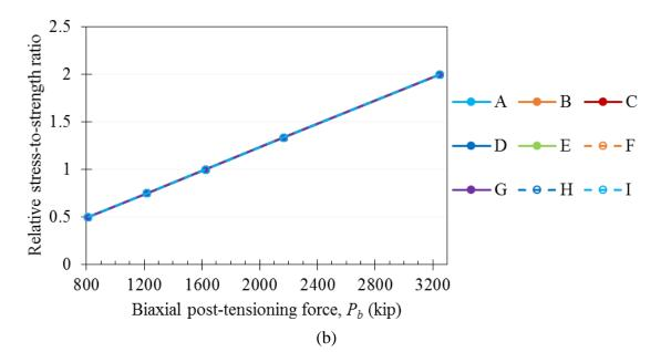
Figure 6.10: Influence of biaxial tensioning force on the (a)  $\sigma_1/f_{tsp}$  values at each point and (b) relative  $\sigma_1/f_{tsp}$  values at each point
