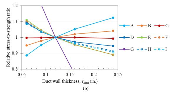
Figure 6.6: Influence of duct wall thickness on the (a)  $\sigma_1/f_{tsp}$  values at each point and (b) relative  $\sigma_1/f_{tsp}$  values at each point
