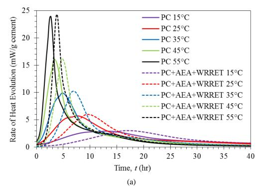
Figure 4.6: (a) Rate of heat evolution, (b) cumulative heat of hydration, and (c) degree of hydration of representative mock-up cement pastes
