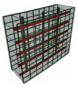
Figure 2.15: Rendering of an RSV with tendons and reinforcement shown Jason et al. (2005).
