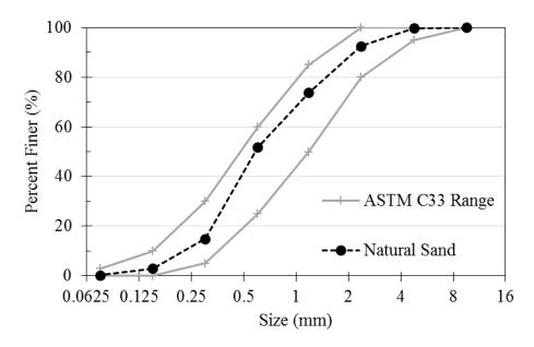
Figure 3.16: Gradation curve of natural silica sand (1 in. = 25.4 mm)
