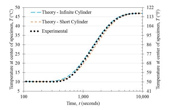
Figure 4.38: Temperature history at center of specimen during thermal diffusivity testing
