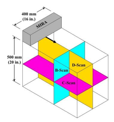
Figure 7.3: Orientation of B-, C-, and D- scan tomograms relative to MIRA antenna and scan path
