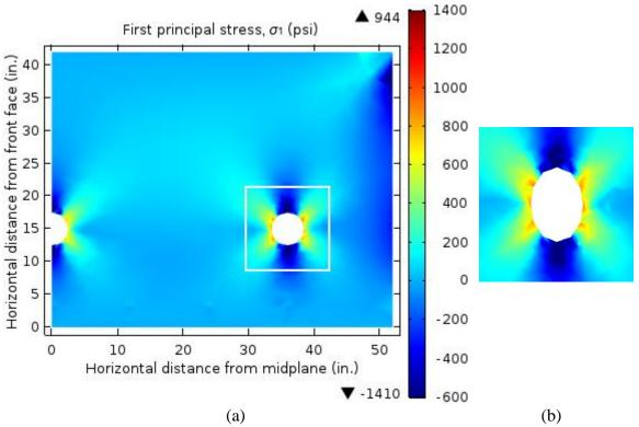
Figure 5.16: Plan view between horizontal ducts of modeled stresses in post-tensioned mock-up concrete, (a) full plan and (b) detail with deformation
