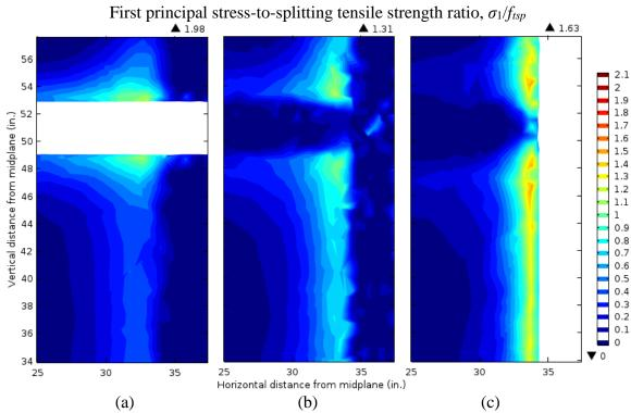
Figure 5.23: Longitudinal section details of modeled stress-to-splitting tensile strength ratio in post-tensioned mock-up concrete in (a) plane of horizontal ducts, (b) plane of contact between horizontal and vertical ducts, and (c) plane of the vertical ducts
