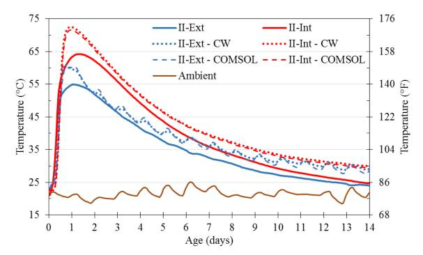
Figure 5.9: Experimental temperatures, corresponding ConcreteWorks (CW) results, and COMSOL Multiphysics results for matching ConcreteWorks
