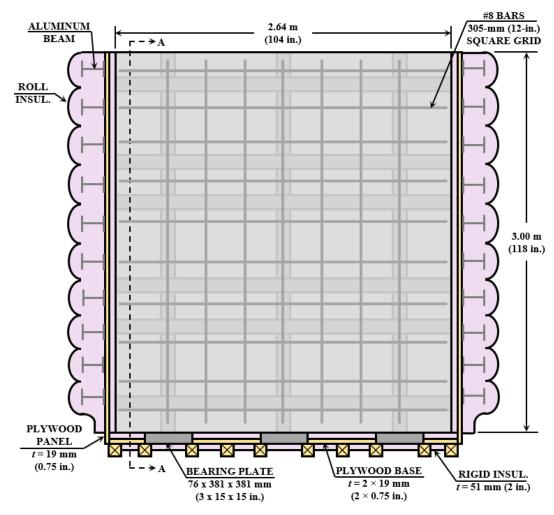
Note: Post-tensioning anchorage reinforcement is not shown Figure 3.3: Front elevation drawing of mock-ups as cast and cured
