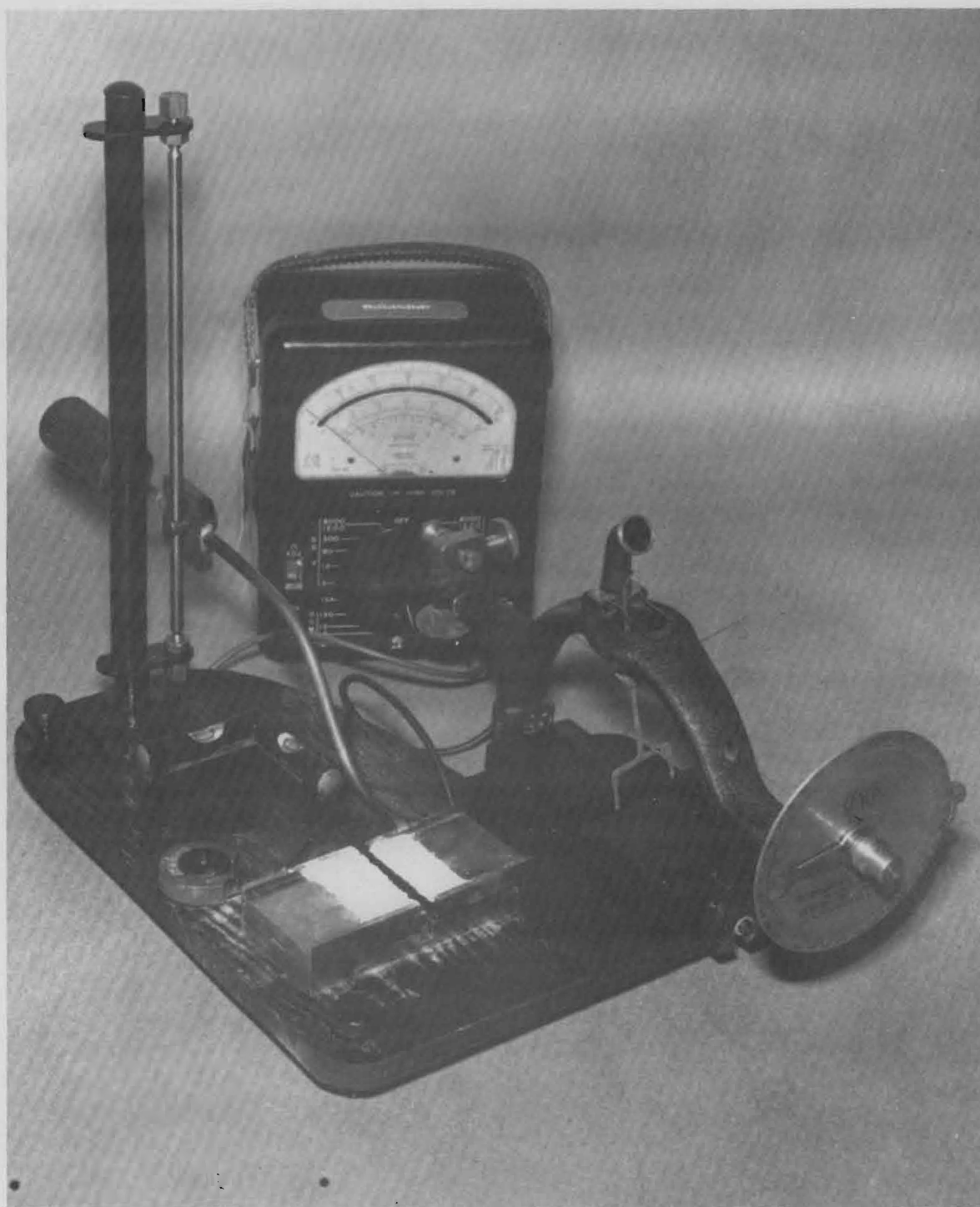
Figure 5. Apparatus for Determining the Bulk Tensile Strength of Uncompacted Powders.
