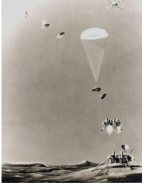
Figure 1: The Viking EDL sequence including rigid, blunt body aeroshell, supersonic parachute, and terminal retropropulsion [5].
