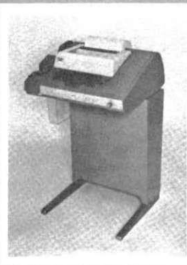
All data can be recorded permanently by a standard teletype.
