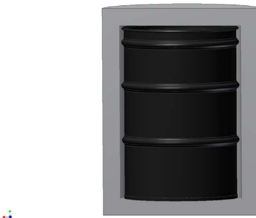
Figure 2.1: Reference drum (black) with overpack (grey) cut away to expose the drum inside
