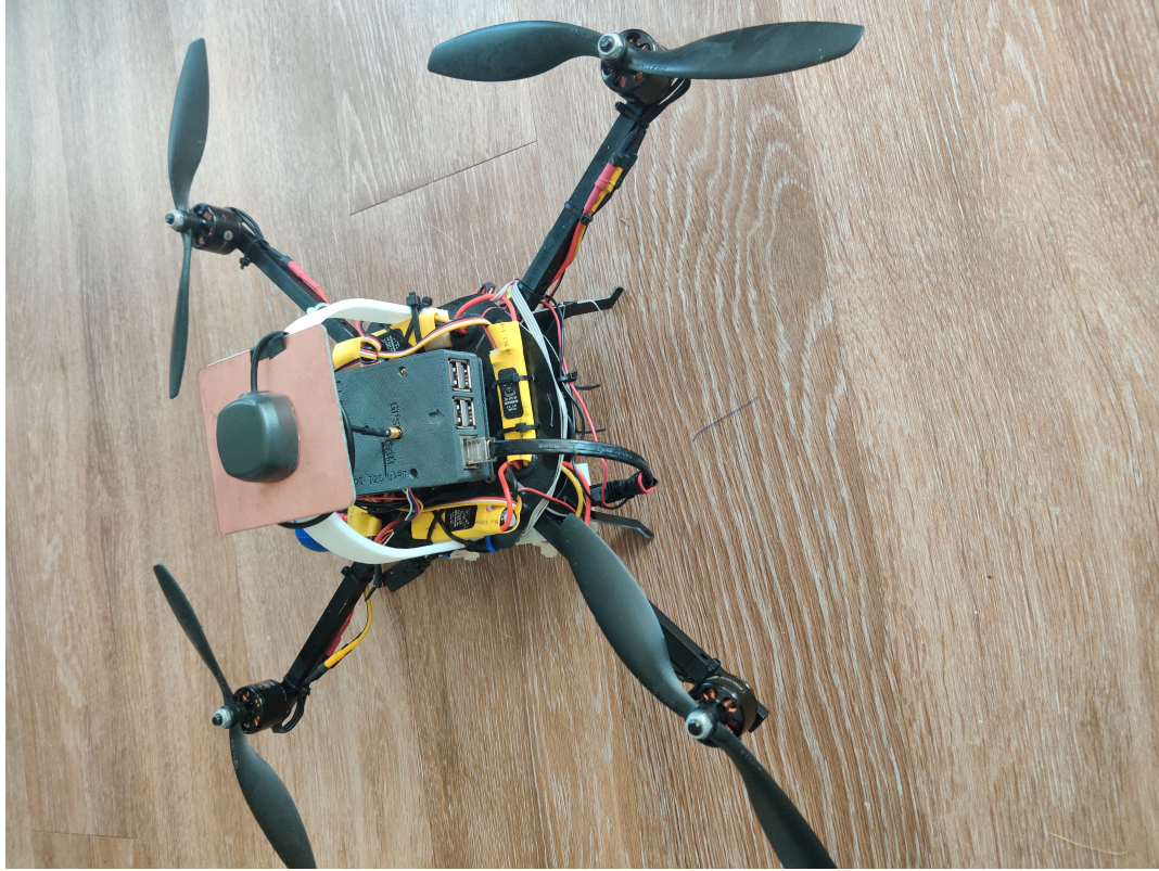
Figure 5.8: UAS research platform used for the flight demonstration. Flight control and onboard computing is provided by a Raspberry Pi 3B embedded computer with an Emlid Navio autopilot sensor suite. UAS frame size is 400mm. A small platform and basic embedded flight computer was chosen to demonstrate applicability to the full range of UAS sizes, as larger platforms can carry more powerful computers.
