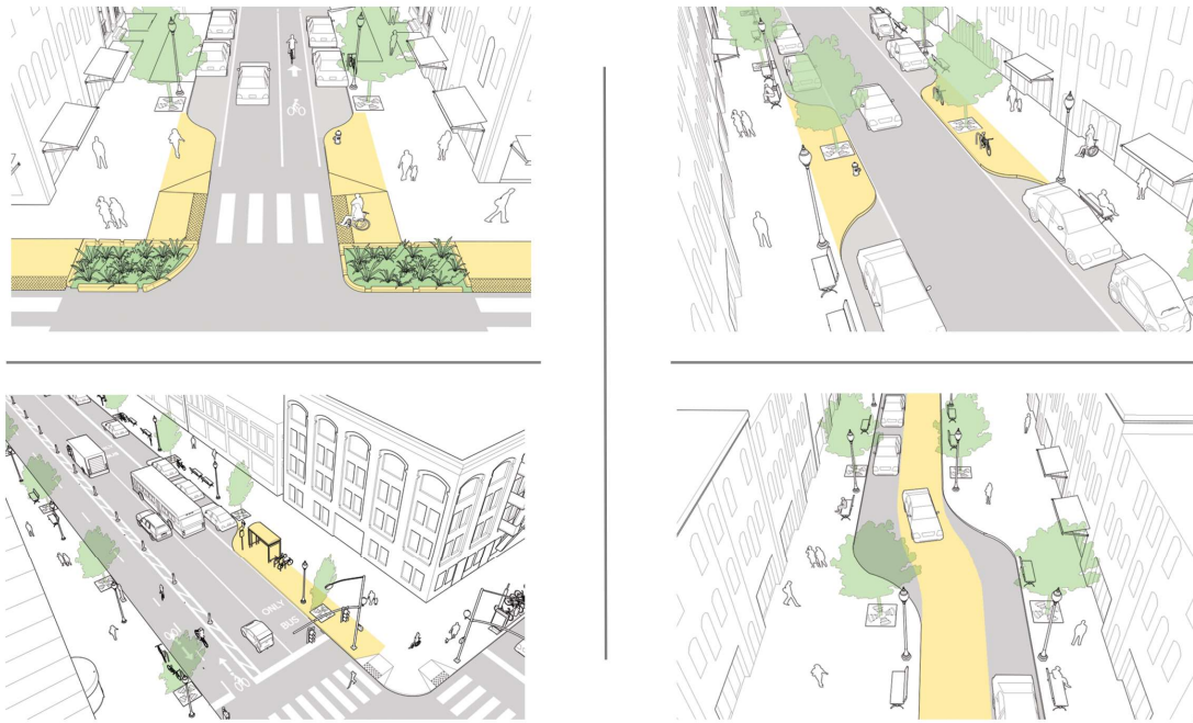
Figure 11 – Stormwater planter and curb extension placements (National Association of City Transportation Officials, 2021)
